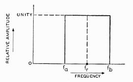
quencies between  $f_a$  and  $f_b$  will be accepted, and all will have the same amplitude. However, such a curve cannot be realized in practice with the use of a single i-f transformer network. Methods which help approach the shape of such a curve entail the use of more than one i-f transformer network, and preferably of three.
