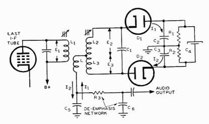
Fig. 7-37. A modified ratio detector circuit in which the coil L receives its voltage by transformer action from the coil  $L_I$ .
