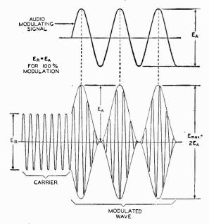
Fig. 1-3. The peak amplitude of the audio modulating signal is equal to the peak amplitude of the carrier wave, resulting in the carrier being 100percent amplitude modulated.
