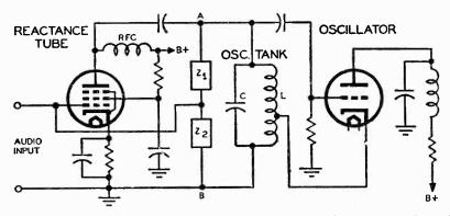
Fig. 3-8. Simplified schematic of a reactance tube modulator (to the left of terminals A-B) with an oscillator circuit of the Hartley type. The impedances  $Z_1$  and  $Z_2$  can be any of the combinations illustrated in Fig. 3-7.
