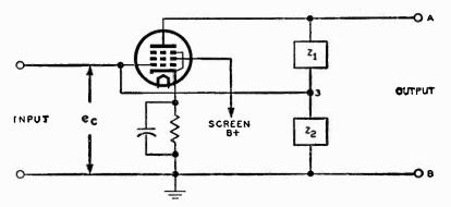
Fig. 3-4. A basic reactance tube circuit. The impedances  $Z_1$  and  $Z_2$  can be a combination of resistance and inductance or resistance and capacitance, but not a combination of inductance and capacitance.
