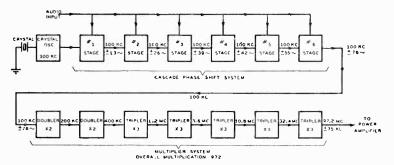
Fig. 4-31. Block diagram of the Raytheon indirect f-m transmitter, omitting the power amplifier stages.
