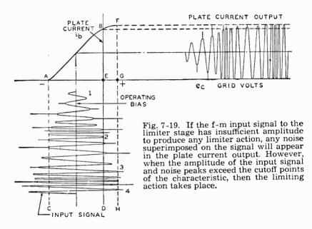
random amplitude. As before, AC and ED represent the points at which limiting action is fairly complete.
