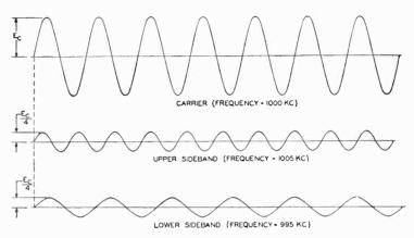
Fig. 1-8. The amplitude of the upper and lower sidebands of a 50-percent amplitude modulated carrier are one-quarter that of the carrier.
