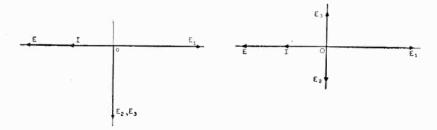
Fig. 7-27 (A), left, (B) right. Vector diagrams of the current and voltage relationships existing in the phase discriminator. Note that in (B) vector  $OE_3$  is shifted in phase by 180° from its position in (A).
