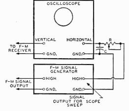
the capacitor C is connected across the horizontal terminals of the oscilloscope, and the resistor is connected in series with the hot lead
