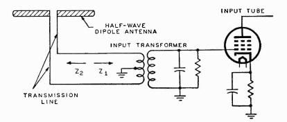
Fig. 6-5. In order to effect a maximum transfer of energy from the antenna to the control-grid of the r-f amplifier tube, the impedance  $Z_z$  of the transmission line and antenna should equal the impedance  $Z_i$  seen looking into the primary of the input transformer.
