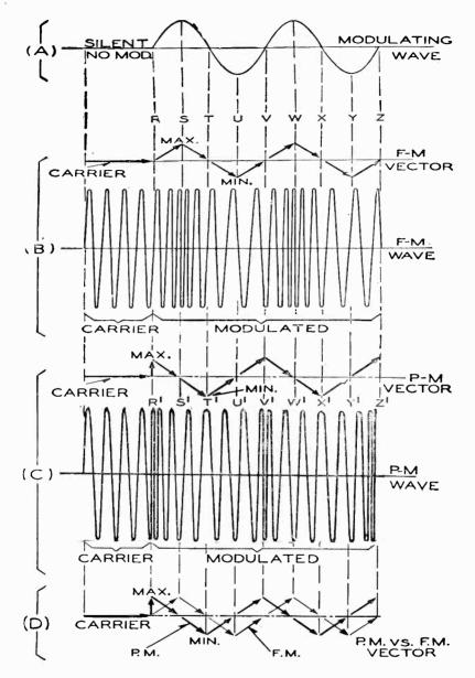
Fig. 1-13. The audio wave at A modulates the same carrier, shown to the left of R and R', in such a way that the resultant wave at (B) is frequency modulated and at (C) it is phase modulated. Above each of these modulated waves is their vector representation, these being combined at (D) for comparison. Note especially where the frequency is increased and decreased in each modulated wave, as indicated by the respective bunching or spreading of the individual cycles.
