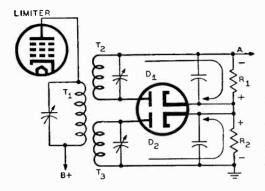
Fig. 7-22. Schematic of the Crosby or double tuned type of discriminator. In this example,  $T_1$  is assumed to be tuned to 10.7 mc,  $T_2$  to 10.775 mc, and  $T_3$  to 10.625 mc, i.e., the two portions of the secondary  $T_2$  and  $T_3$  are tuned 75 kc above and below the resonant frequency of the primary respectively.
