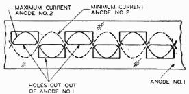
line with the sinusoidal rim of the electron disk. Anode No. 1 is nearer the cathode and anode No. 2, which is a cylindrical electrode without any holes punched in it, lies directly behind anode No. 1, as illustrated in Fig. 4-19.
