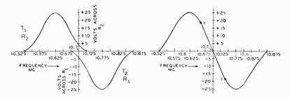
Fig. 7-24 (A), left, (B) right. If the output voltage developed across  $R_1$  and  $R_2$  of Fig. 7-22 is plotted against frequency, the response curves of (A) are derived. These curves can be combined, as in (B), resulting in the S characteristic of a discriminator.
