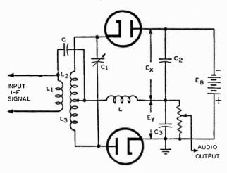
Fig. 7-35. Simplified schematic of the ratio detector. In this circuit the diodes are series aiding with respect to the load instead of series opposing as in the discriminator detector circuit.
