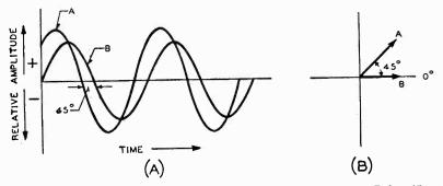
Fig. 1-9. Wave A has a greater amplitude than B and leads B by  $45^{\circ}$ , as indicated. The vectorial representation of these two waves is shown in (B) where the larger vector A is shown leading B by  $45^{\circ}$ .
