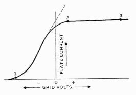
be discussed in detail later on. If diode clipping did not occur, the curve, instead of taking on the shape between points 2 and 3, would continue onward as shown by the dashed line.
