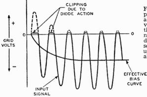
Fig. 7-16. The dotted portions of the wave above the zero gridvoltage axis show what the signal would be if no clipping occurred due to diode action; the solid curves show a uniform amplitude above the zero axis.
