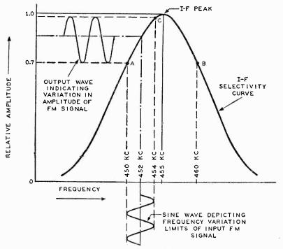
Fig. 4-54. The effect of a typical i-f selectivity curve of an a-m receiver on an f-m signal.
