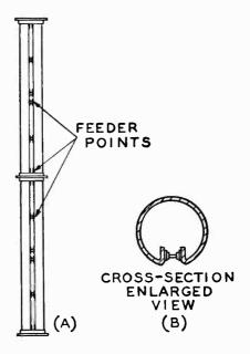
the horizontal radiation pattern and also the length of the antenna section so far as resonance at the desired frequency is concerned. The width of the slot of the antenna is the most important determining factor in the input impedance of the antenna.
