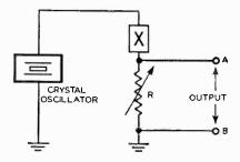
of phase modulators in existence. However, a basic phase modulator circuit will illustrate how p.m. can be produced.
