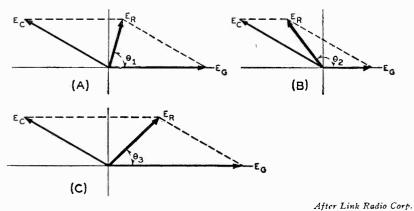
Fig. 4-51. Vector diagrams of the voltage relationships in the circuit shown in Fig. 4-50.
