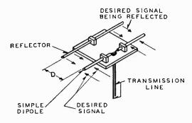
Fig. 6-10. In order to increase the pickup, a reflector element is placed behind the dipole in the same plane at a distance D, that is between onetenth and one-quarter of the wavelength for which the dipole is cut.
