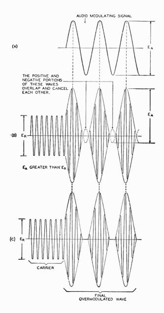
Fig. 1-5. When the peak amplitude of the modulating wave (A) is greater than the amplitude of the carrier wave, the resulting modulated wave (C) is said to be overmodulated. Notice that the resultant overmodulated wave is not continuous, which means that the output of the receiver will be distorted.
