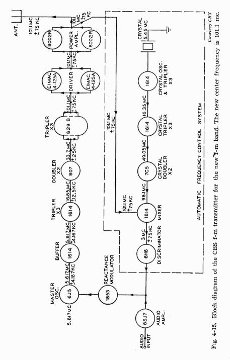
electronic kind described in chapter 3. The center frequency of transmission on the old band was 46.7 mc and on the new band it is 101.1 mc.
