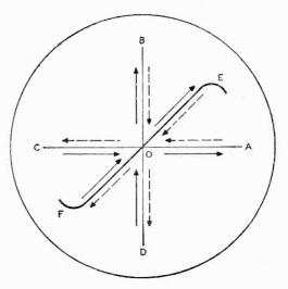
back to point O, shown by the solid line, thus completing the cycle. What actually happens is that from point A when the spot is moving to the left, it is really moving over the same line traced out by OA, but in the picture of Fig. 8-5 it is shown slightly displaced for the sake of illustration.
