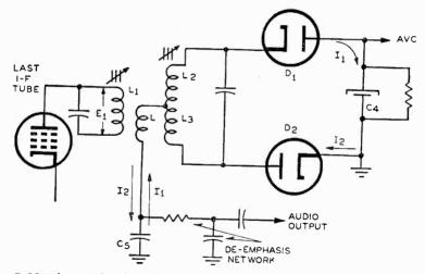
Fig. 7-38. A modification of the circuit of Fig. 7-37:  $C_2$  and  $C_3$  have been removed from the circuit and the cathode of the diode  $D_2$  is now grounded. The coil L is again inductively coupled to  $L_1$ .
