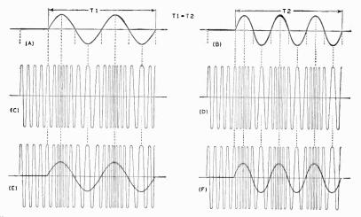
Fig. 2-2. The frequency of the modulating wave of (A) is less than that of (B), the time intervals  $T_{\tau}$  and  $T_{z}$  being equal. Notice the two groups of frequency changes in the modulated wave at (C) and the three in the wave at (D), which occur in the same period of time. The modulating waves are superimposed on their respective modulated carriers in (E) and (F).
