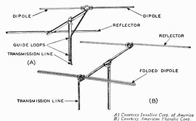
Fig. 6-11. Reflector elements are used not only with simple dipole antennas (A), but also with folded dipoles, as shown in (B).
