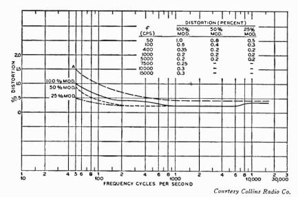
Fig. 4-46. Percentage distortion of the Collins f-m transmitter plotted against audio frequencies is one percent or less for 25%, 50%, and 100% modulation.
