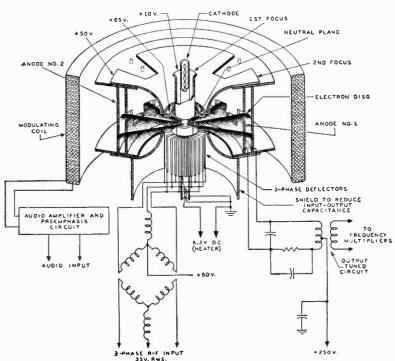
No. 1. A schematic diagram of the Phasitron tube is shown in Fig 4-20 with typical operating voltages shown alongside each electrode.
