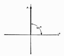
Fig. 1-2. The relative phase of the sine wave in Fig. 1-1 is shown vectorially here by the vector A, being at 90° to the 0° axis.
