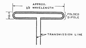
length of wire (or appropriate tubing or rod) bent so that it takes on approximately the shape shown in Fig. 6-7. In Fig. 6-8 are shown three typical folded-dipole f-m antennas as used today. Those shown in parts (A) and (B) are typical outdoor folded dipoles, while that shown in part (C), although suitable for outdoor use (with proper
