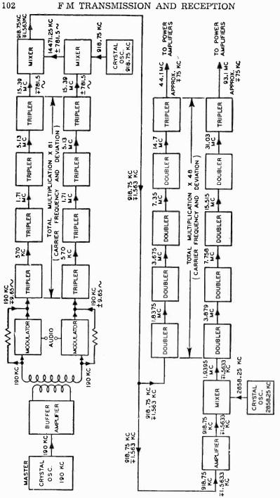
Fig. 4-4. Block diagram of Armstrong "dual channel" transmitter.
