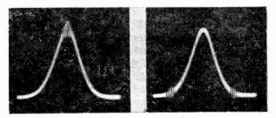
scope. The markers will fall either above or below the center i.f., thus indicating which is the upper limit and which the lower. In Fig. 8-17, the marker frequency identifies the peak of the response curve, and
