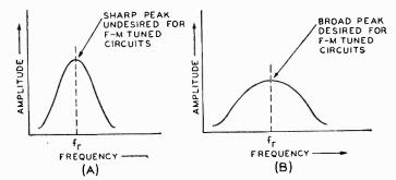
Fig. 7-3. When the Q of a circuit is high, the frequency response is sharply peaked (A) and when the Q is low, the response curve (B) is broad, which is the desired condition for f-m r-f circuits.
