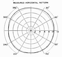
Fig. 5-12. The measured horizontal radiation pattern of the square-loop antenna array is circular, which if it were calculated mathematically, would be approximately a square, as this method does not take into account the end effects of the half-wave elements of each square loop.
