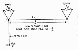
Fig. 6-19. Schematic representation of an omnidirectional antenna, where  $Z_o$  is the characteristic impedance of the transmission line and is also the impedance of the two antenna elements.
