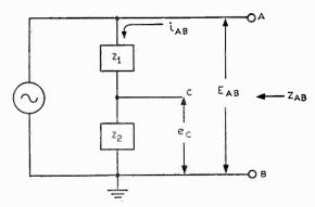
of the series resistance is equal to  $1/g_m$ , and the value of the reactance is equal to  $1/g_m \times Z_1/Z_2$ , where  $g_m$  is the transconductance of the tube in use and impedances  $Z_1$  and  $Z_2$  are, as specified previously, any one of four combinations.
