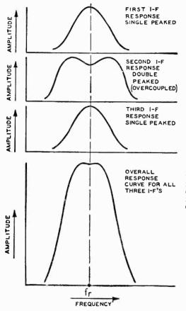
Fig. 7-9. By employing three i-f stages in which two of the stages are single-peaked below critical coupling and the other double-peaked (overcoupled), a somewhat broad, flat-top over-all response curve can be obtained. The response curve for the complete system is obtained by combining the individual response curves of each i-f stage.
