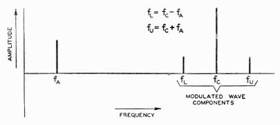
Fig. 1-6. In this spectral distribution of a 50 percent a-m wave,  $f_A$ , is the modulating signal, which is one-half the amplitude of the carrier component,  $f_C$ . The upper and lower sidebands,  $f_U$  and  $f_L$ , are the sum and difference of the modulating and carrier frequencies, their amplitudes being ½ of  $f_A$ .
