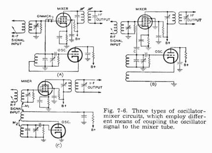
mixer tube. The tickler coil in this oscillator is in the cathode circuit of the tube. The proper choice of the value of C will determine the closeness of coupling between the oscillator and signal circuits.
