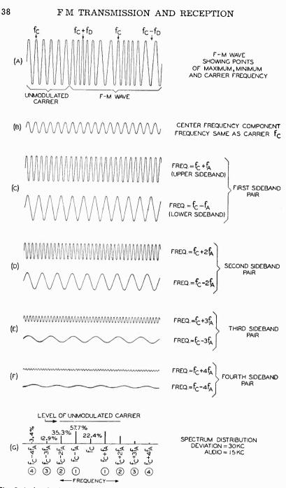
Fig. 2-4. Analysis of an f-m wave with respect to its sidebands and center frequency component.
