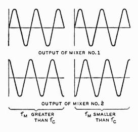
Fig. 4-41. When the instantaneous modulated oscillator frequency  $f_M$  is higher than the crystal frequency,  $f_C$ , the output of mixer No. 1 lags that of No. 2 by 90°; and when  $f_M$  is lower than  $f_C$ , the output of mixer No. 1 leads the output of No. 2 by 90°.
