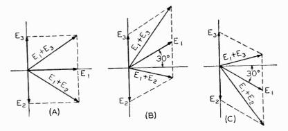
Fig. 4-30. Vector diagrams of the circuit of Fig. 4-29. If the frequency of the input to  $T_1$  is the same as that into  $T_2$ , then  $E_1$  will be 90° out of phase with  $E_2$  and  $E_3$ , as shown in (A). If the input to  $T_2$  changes, then the relationship of  $E_1$  to  $E_2$  and  $E_3$  changes in phase, as shown in (B) and (C).
