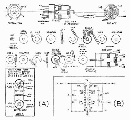
Fig. 7-11. The arrangement of the components making up the f-m and a-m i-f transformers used in a Zenith receiver is shown in (A). The series-connected primary and secondary coils and the capacitors across them are shown in the schematic in (B).
