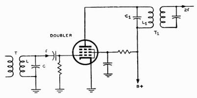
Fig. 3-15. A frequency-doubler circuit has its input transformer T tuned to some frequency f and its output circuit  $T_{I}$  adjusted to 2f, the second harmonic, the tube operating as a class C amplifier.
