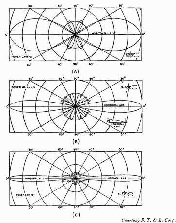
Fig. 5-11. Vertical radiation patterns for 2, 4, and 8 loops in (A), (B), and (C), of the square-loop antenna show that as the number of loops is increased, the vertical power radiated is decreased.
