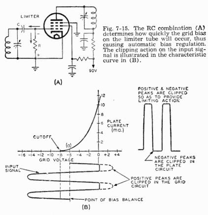
Since there is zero fixed bias on the tube, the control grid will be driven positive during the positive half of the input signal with respect to the cathode, which is at ground potential. As soon as the grid is driven slightly positive, the grid and cathode act as a diode rectifier where the grid takes the place of the diode plate and grid current starts to flow.
