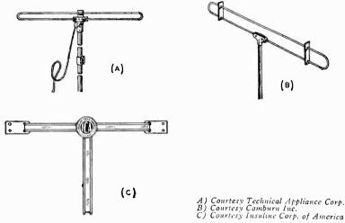
Fig. 6-8. Three types of folded dipole antennas. Those illustrated in (A) and (B) are for outdoor use and that in (C) is for indoor or outdoor use.
