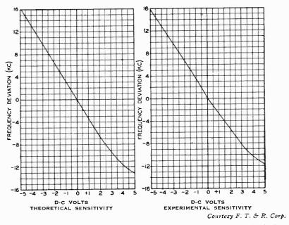
Fig. 4-27. Grid voltage,  $E_c$ , plotted against computed frequency deviation (A) and grid voltage vs. experimental frequency deviation (B). The difference between the calculated and experimental deviation was 8 percent.
