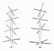
Fig. 5-7. Two types of turnstile antennas are illustrated at the left. In (A) each of the four bays consists of two halfwave dipoles and in (B) each individual bay consists of two half-wave folded dipoles at right angles to one another.
