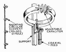
Figs. 5-3, left, 5-4, right, 5-5 below. A four-bay circular antenna, one element of which is shown at the right. Below is shown the horizontal field strength pattern taken at 107 mc for the bottom bay of an 8-bay antenna.
