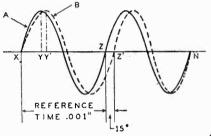
Fig. 1-11, left. Of the two 1-kc waves, A is the reference wave and leads B, as the latter has passed through a variable delay network, which lowers its frequency to 960 cycles at point Z'. At point N, the waves are again at 1 kc as they were at the start.
