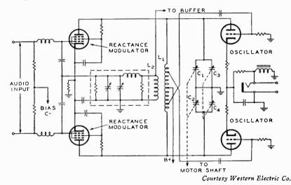
Fig. 4-12. The modulator-oscillator stages of the Western Electric transmitter.
