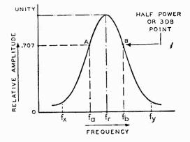
power or 3-db points as shown by A and B on the curve of Fig. 7-7. The frequencies that correspond to these half power points are designated as  $f_a$  and  $f_b$ , respectively. Any signals that fall outside these two frequency limits are considered not to have enough signal strength to be acceptable. This means that such frequencies as  $f_x$  and  $f_y$  in Fig. 7-7 are not acceptable, but that all frequencies between  $f_a$  and  $f_b$  are acceptable.
