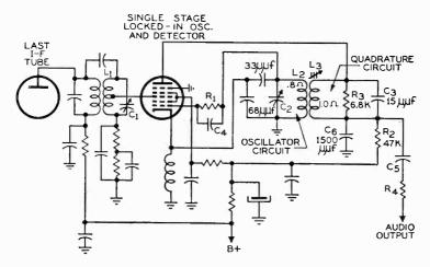
Fig. 8-3. Schematic of the locked-in oscillator and detector circuit, which is aligned by first adjusting the i-f stages, then the detector, high-frequency oscillator, and the r-f networks last.
