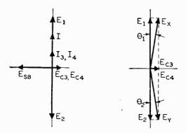
Fig. 4-9, left, 4-10 right. Vector diagram (left) of the electrical quantities indicated in Fig. 4-8, where  $E_1$  and  $E_2$  are equal but opposite phase crystal frequency voltages across  $C_3$  and  $C_4$  respectively. Fig. 4-10 is the vector diagram of the voltages appearing at the grids of the triplers.
