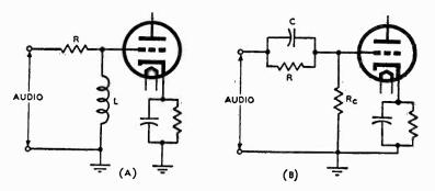
Fig. 4-48. In these two pre-emphasis networks as the audio frequencies increase the voltage to the grids of the tubes also increases.
