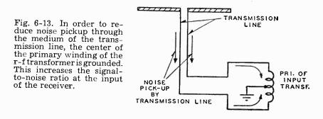
system of noise reduction somewhat clearer. Since the transmission line used may cover a greater area than the antenna itself, it has a tendency to pick up noise voltages, especially if the transmission line is quite long. To reduce this noise pickup and, hence, increase the signal-to-noise ratio at the input to the f-m receiver, the center tap of the primary is grounded. It reduces noise pickup in the following manner:
