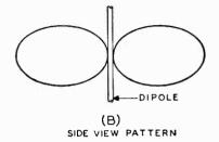
Fig. 5-1. The pattern of the electromagnetic radiation from a dipole antenna is shown pictorially in (A). A cross section of the pattern from the side of the dipole is shown in (B) and its appearance when viewed from an end of the dipole is shown in (C). These views of the radiation pattern are drawn for a vertical dipole.
