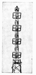
Fig. 5-9, left, Fig. 5-10, below. The square loops of the antenna shown in (A) give a somewhat greater power gain than either the circular or turnstile antennas from the standpoint of the number of bays used in each type. Graph below indicates the number of degrees separation between the loops plotted against the horizontal power gains for a different number of loops. This shows that the greater the number of loops, the greater is the power gain.
