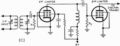
Fig. 7-21. When two limiters are used in cascade, the method of coupling used between them may vary widely. In (A) transformer coupling is employed, in (B) resistance-capacitance coupling, and in (C) impedance coupling is used. In each case the time constant for the first stage is established by R and C and in the second stage by  $R_I$  and  $C_I$ . The time constant for each stage is usually different.
