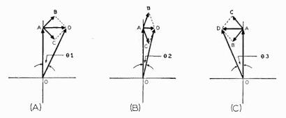
Fig. 3-19. In an f-m signal, the double sideband (vector AD) is 90° out of phase with the carrier (vector OA). The resultant vectors are never smaller than that of the carrier.
