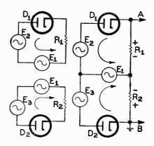
tified current flows through the individual diode circuits put certain polarities on their load resistors. Since the external current in a diode rectifier circuit flows from plate to cathode, the currents in the diode load resistors will be flowing in opposite directions, and the polarities across the individual load resistors will be bucking each other. Thus between points A and B a voltage will exist which will be the difference between the voltage drops across resistors  $R_1$  and  $R_2$ .
