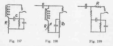
The value of R is about 25,000 ohms maximum for grid chokes up to about 500 henrys. For chokes higher than this values, R should have a maximum value of about 50,000 ohms. It is interesting to note that the usual bypass capacity is not used in this case, the only
