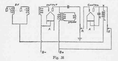
will naturally change the voltage applied to the control tube and the radio frequency amplifiers. If for some reason the current through R is changed and the voltage drop across that resistance is increased, the voltage effective at point X will be less than prior to the increase in current. Now, if a signal voltage is applied across the output tube primary, this voltage is applied across the grid and
