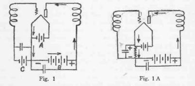
tery in figure 1 supplies the bias for the tube. It is possible however to eliminate the C battery in battery operated receivers by the use of a resistance in the B- circuit so arranged that a voltage
