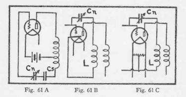
the tube. The neutralizing system consists of the inductance L and the capacity Cn, the complete circuit being connected between the cathode and the grid.
