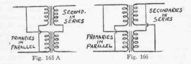
**VOLTAGE WINDINGS IN PARALLEL.**—When the current requirement is in excess of that available from one winding another of like rating can be connected in parallel with the first and the current output will be approximately doubled whereas the voltage remains as that of either one. The primaries must be in parallel. See figure 166.
