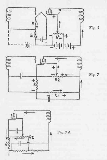
able a variable "+" voltage for the screen grid. If we were to eliminate the use of the resistance R to supply the grid bias, the location of the C battery would be as shown in dotted lines.
