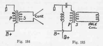
Relative to the designations P.S. in the aforementioned illustrations the former designate the primary winding of the transformer and the latter the secondary winding. The severed connections between S and the voice coil indicate that the circuit is interrupted at two points.
