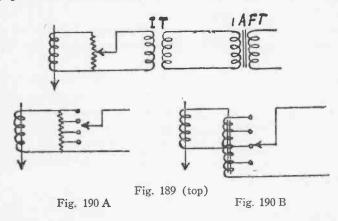
Electric pickup units manufactured for general application are equipped with simple potentiometer type volume control units. The approximate resistance of such potentiometers is about 25,000 ohms. These units are suitable for application unless specification has been made to the contrary, directly across the primary of the audio frequency transformer in the first audio stage.
