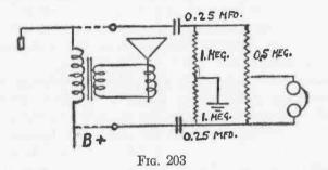
The method of connecting headphones to a push-pull tube output system is as shown in figure 203. The output is connected across the transformer primary. The dotted lines in each case illustrate the connection to be added.
