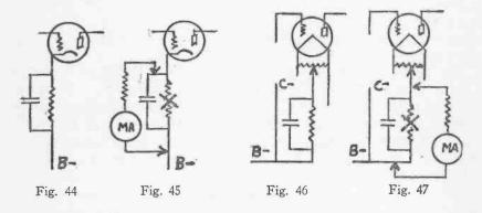
The systems shown in figures 44 and 45 are much more common, wherein the grid bias resistance is located in the cathode circuit or in the filament center tap-B minus circuit. What has been said in connection with an open bias resistance in figure 43 is applicable to figures 44 and 45. We have taken the liberty in figures 44 and 45 to show only the bias systems. In the former the
