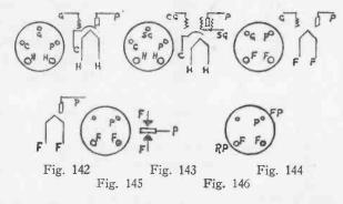
the filaments of the 381 and P is the plate. The grid prong is not used. In the case of the Raytheon tube, the leads from the transformer connect to the filament terminals and the cathode is the
