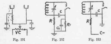
will make necessary shifting of the bypass condenser so that it bypasses the supplementary voltage reducing resistance. This resistor need not be rated at higher than 10 milliamperes and the bypass capacity need not be more than .25 mfd. See figure 191 for the location of the resistance R. VC is the volume control unit. C is the bypass capacity.
