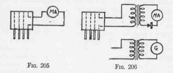
The recommendation of a 0-2 D.C. milliammeter is based upon the fact that such a meter affords a wide scale and will show small variations. However, it is limited to use in systems where the plate current when normal is not in excess of 2 milliamperes. In the event that the normal plate current is in excess of this value, a 30 ohm rheostat can be connected in shunt with the meter to increase its range.
