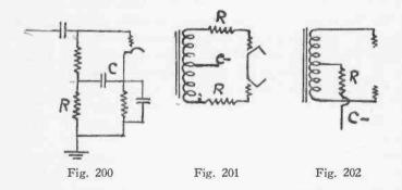
**PLATE FILTER RESISTANCES.**—Plate filter resistances are nothing more than combination voltage reducing resistors functioning in conjunction with a by pass capacity.
