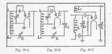
good practice to preclude damage by connecting a fixed condenser in series with C and the tickler coil return. The value of such an isolating condenser need not exceed .1 mfd.
