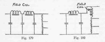
out interfering with the action of the field winding as a choke. When the two are to be separated, the voice coil can remain intact in a speaker not connected to the output of a receiver without interfering with the operation of the field winding when that winding is employed as a choke. . . Let us continue.
