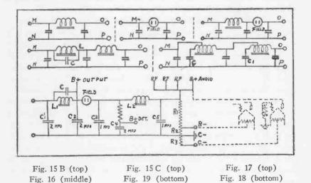
Another modern deviation from the conventional is the use of associated equipment in place of the conventional choke. In days of old, the chokes in the filter were of special construction and bore the designation "filter choke." In many modern receivers one of these chokes is replaced with the field winding of the dynamic speaker. Several manufacturers of radio receivers employ the speaker field winding as the only choke in a single section filter as
