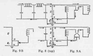
nected to the point Q and the cathode to the point P. The voltage across these two points is the voltage across the grid and the cathode, hence the negative grid bias.
