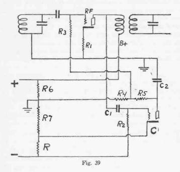
so that the plate current will increase when a signal is applied to the grid. The adjustment of R1 enables the setting of the control tube for whatever volume is desired. The circuit shows the control tube connected across the output transformer primary. Such wiring is not imperative. It is possible to connect the control tube across the speaker terminals, in which case a separate C
