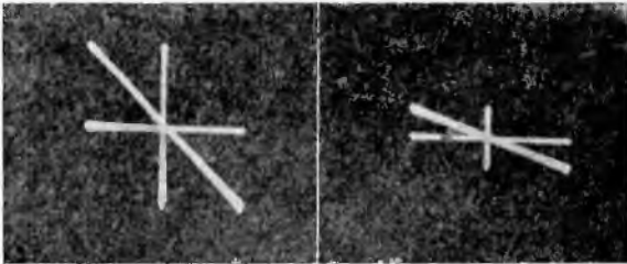
Fig. 93-C, left, Fig. 93-D, right. A phase difference of 0^\circ exists between the two voltages. In C equal amplitudes on both axes give the pattern a 45^\circ angle with the horizontal, but when the horizontal
