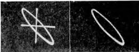
Fig. 93-E, left, Fig. 93-F, right. Pattern for a phase difference of about 45^\circ . Both E and F are the same pattern, but the X and Y axes were omitted from F.
