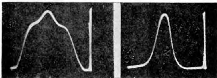
Fig. 276, left, Fig. 277 right. The resonance curve in Fig. 276 is non-symmetrical and that in Fig. 277 is symmetrical. These oscillograms were made using the frequency modulator and sweep described in Fig. 275. The vertical line on the right of each oscillogram indicates the vertical displacement due to change in frequency, but as the sweep was shorted, it is not spread across the screen.
