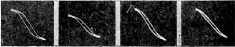
Figs. 142, 143, 144, 145 (reading from left to right). These hysteresis curves were made at 100 cycles. The greater the saturation, the flatter become the ends of the curve. Fig. 142 indicates the greatest saturation of these four oscillograms. Note that the area of these patterns (indicating the core loss due to hysteresis) is less than that of Fig. 147.
