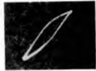
Fig. 146, left, Fig. 147, right. The amount of saturation in these two oscillograms is appreciably less than that shown in Figs. 142 to 145. The core loss due to hysteresis, indicated by the size of the area enclosed by the curve, is fairly large in Fig. 147.
