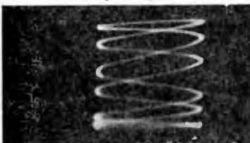
Fig. 103. The ratio between the voltages impressed on the tube's plates was 6-1 when this Lissajous figure was photographed. The six loops are easily seen on the right side of the pattern.
