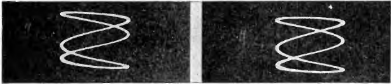
Fig. 97. C, left, D, right. 3-1 ratio patterns obtained by using two different phase relationships.
