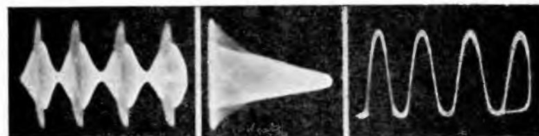
Fig. 418 shows the modulated wave. Fig. 419 shows the corresponding trapezoidal pattern and Fig. 420 shows the audio wave across the modulator output during the operative condition stated. The sudden start and cessation of the uncontrolled oscillation is clearly shown in Fig. 418.
