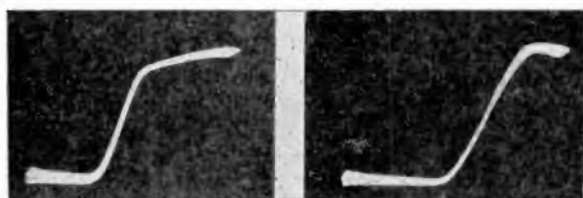
Fig. 132, left, Fig. 133, right. Tube characteristics obtained when the filament, grid and plate voltages were held constant and changes made in the load resistance, R_1 of Fig. 128. The pattern of Fig. 132 was photographed when R_1 = 0 and that of Fig. 133 when R_1 = 10,000 ohms.
