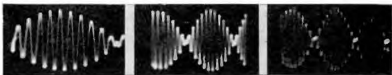
Figs. 436 (left), 437 (middle), 438 (right). These three oscillograms were obtained by connecting the output of two oscillators in series, each delivering a different frequency. With the sweep frequency equal to the difference frequency, the oscillogram of Fig. 436 was obtained. The oscillograms of Figs. 437 and 438 were obtained with the sweep frequency equal to one-half and one-third the difference frequency respectively.
