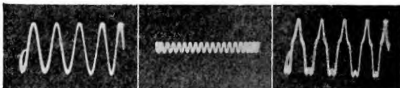
Figs. 170, left, 171, middle, 172, right. The 1000-cycle wave, Fig. 170, is the fundamental and the 4000-cycle wave, Fig. 171, is its fourth harmonic. The composite wave is shown in Fig. 172. Compare with Fig. 167 for changes in the shape due to the substitution of the fourth for the third harmonic.
