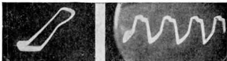
Figs. 193, left, 194, right. The distorted characteristic curve of Fig. 193 was caused by turning the volume control on full and this, with the distorted output wave of Fig. 194, showed that something was inherently wrong in the circuit.
