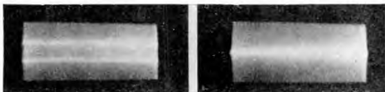
Figs. 384, left, 384-A, right. Two block patterns are here shown. That of Fig. 384 has fifty percent. modulation and that of Fig. 384-A is modulated one hundred percent.
