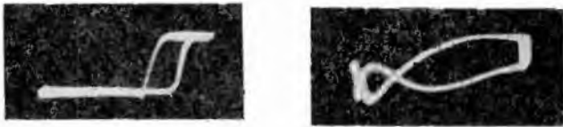
Fig. 139, left, Fig. 140, right. The oscillogram of Fig. 139 was made at 40 cycles and that of Fig. 140 was made at 1000 cycles. The phase shift present in these patterns is clearly evident. Compare Figs. 129 to 133.
