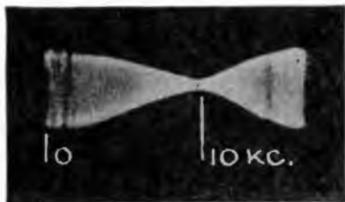
Fig. 343, left. The effect of a tone control on the a-f. response curve is shown at the left.
