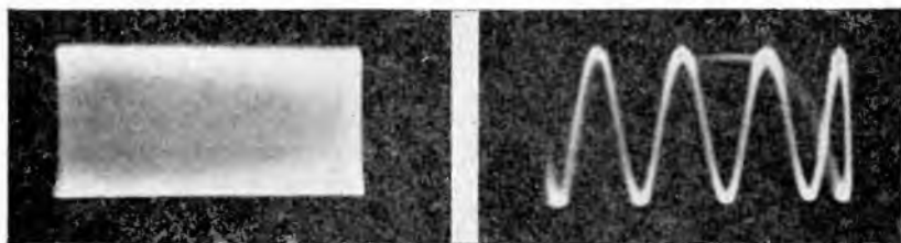
Figs. 227, left, 228, right. The unmodulated 100-kc. carrier from an oscillator that is free of harmonics gives a pattern free of streaks, as is shown in Fig. 227. Several cycles of the wave, which was used to obtain the oscillogram of Fig. 227, are shown in Fig. 228.
