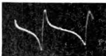
Fig. 255. Two cycles of the waveform produced by the impulse generator, which is that part of the RCA frequency modulator that brings about synchronization between the rate of frequency modulation and the linear sweep voltage.
