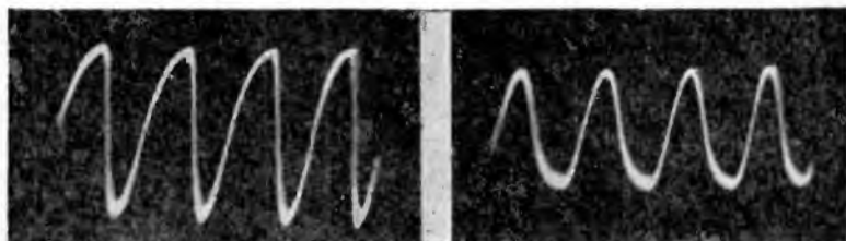
Figs. 222, left, 223, right. The wave shown in Fig. 222 was taken across R-2 (Fig. 221) and shows distortion deliberately introduced. When the voltage was taken across R-5, the wave of Fig. 223 was obtained. Note that the distorted peaks are now on the bottom, showing that the wave has been shifted through 180°, which is the function of the phase inverter tube.
