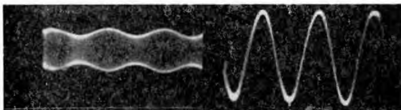
Figs. 196-A, left, 196-B, right. When the i-f. amplifier is functioning properly, the peaks of the modulated wave envelope should not be flattened, see Fig. 196-A. The equivalent a-f. signal, taken across the demodulator load, is shown in Fig. 196-B.
