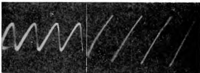
Fig. 35 (left) shows the output waveform of a sweep circuit of a commercial oscillograph with a low tripping voltage, making the charging portion of the wave fairly linear. Fig. 36 (right) shows the same wave with the amplitude control advanced, resulting in a slight departure from the good linearity of the wave of Fig. 35.
