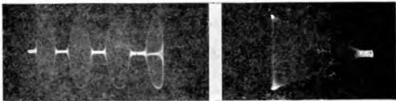
The wave envelope and trapezoidal patterns indicating overmodulation with all other conditions normal, is shown in Figs. 403 (left) and 404 (right)
