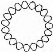
Fig. 124, above, Fig. 125, right. The circuit in Fig. 125 will produce a gear-shaped pattern like that in Fig. 124. The condenser reactance should equal the resistance for the frequency used.
