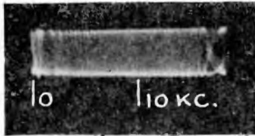
Fig. 337. An oscillogram of the output of the a-f. frequency modulator. Note that it is linear over the band from 0 to 10 kc.
