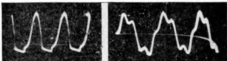
Fig. 237, left, Fig. 238, right. Two oscillograms obtained from an audio oscillator in which regeneration was excessive and a very high L-C ratio.
