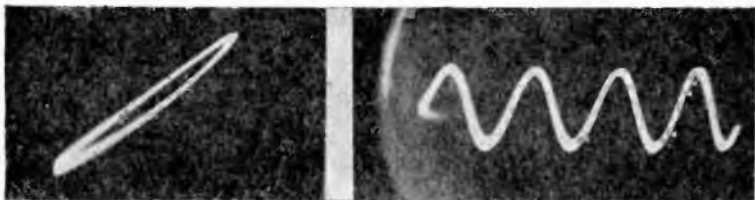
Figs. 189, left, 190, right. The input-output signal voltage characteristic of the a-f. amplifier of a receiver with a medium setting of the volume control, which was the diode's load, is shown in Fig. 189. The sine wave output is shown in Fig. 190.
