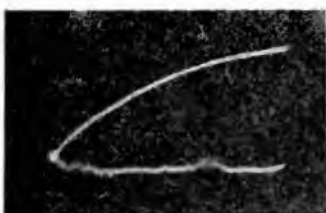
Fig. 257. An oscillogram of the sweep voltage employed in the Clough-Brengle frequency modulator. The horizontal line represents that period of the cycle when the shorting contact is closed and the rising portion of the curve is the time when the condenser is charging.
