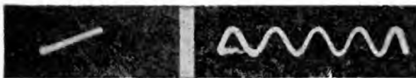
Figs. 181, left, 182, right. The input-output voltage characteristic for distortionless operation is shown in Fig. 181. That it is distortionless is shown by the undistorted sine wave output of Fig. 182.
