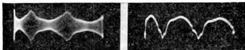
Fig. 236-C, left, Fig. 236-D. The modulated output waveform of the same oscillator when adjusted to 1700 kc., is shown in C. The a-f. output resulting from the demodulation of C is shown in D.
