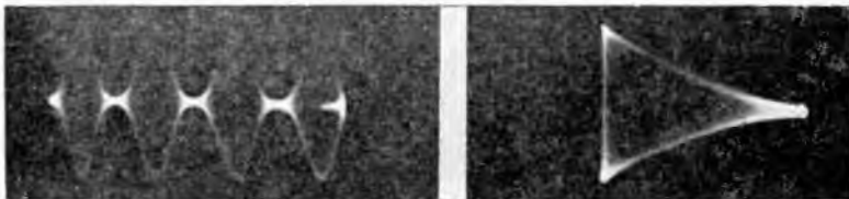
The wave envelope and trapezoidal patterns for this condition are shown in Figs. 405 (left) and 406 (right). Note that the condition is not as evident in the modulated wave pattern as in the trapezoidal pattern.
