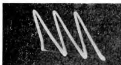
Fig. 138, left. When the sweep frequency was increased after the pattern of Fig. 137 was photographed, the three cycles of the wave, shown on the left, indicate the necessity for having the deflecting coils properly oriented with respect to the sweep
