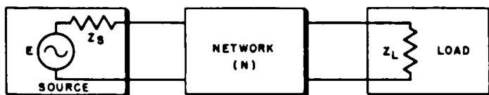
(A) GENERALIZED DIAGRAM SHOWING THE CONNECTION OF A NETWORK IN A CIRCUIT.
