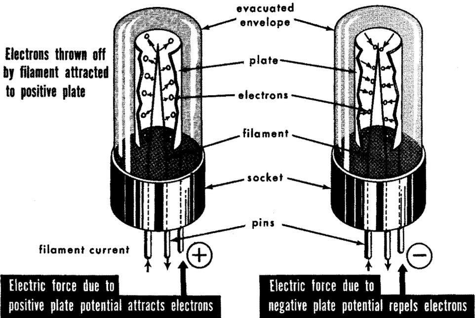
The first electronic amplifiers used a tube type called a *triode* because it has *three* active electrodes. The earliest triodes started with an addition to the *diode* (*two-electrode*) tube which used a filament of wire heated by passing a current through it and a piece of cold metal called a *plate*. These elements were placed in a space from which all the air was evacuated, usually enclosed by a glass *envelope*.
