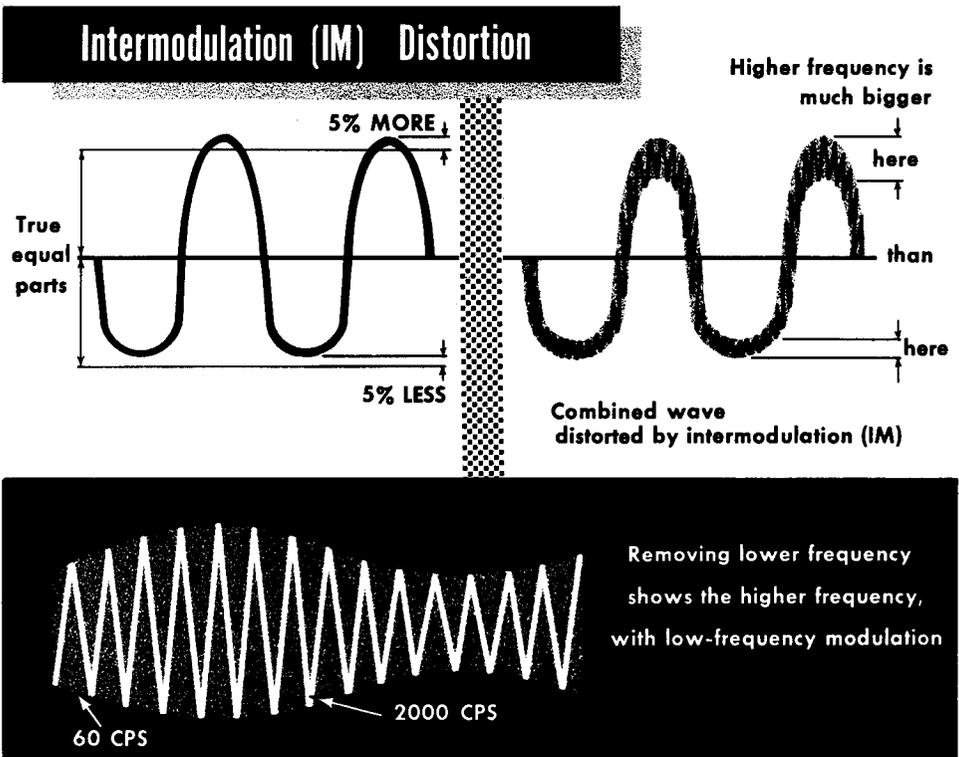
Suppose that a 60-cycle wave has 5% of second harmonic. This will mean one-half of the wave will get amplified by 5% more, while the other is amplified by 5% less. If the amplifier is also called upon to handle a 2000-cycle wave of much smaller magnitude than the 60-cycle wave, this will also get amplified by 5% more on one peak of the 60-cycle wave than it does on the other peak of the 60-cycle wave. Thus the 2000-cycle wave will be fluctuating in amplitude at the rate of 60 cycles.
