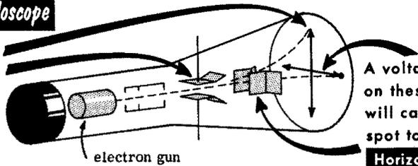
A voltage applied on these plates will cause the spot to move **Horizontally**
