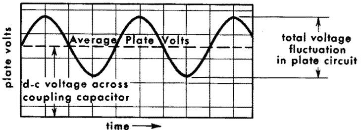
A capacitor placed between the plate and the a-c voltmeter takes on a charge corresponding to the steady or d-c component of the voltage, but does not have time to alter that charge with the alternating component. The voltmeter, therefore, measures only this alternating component.
