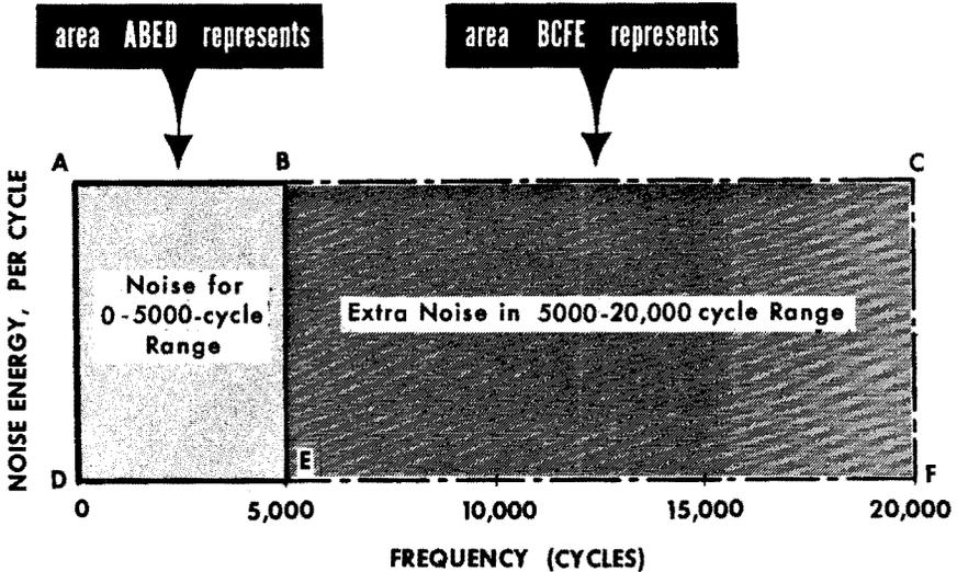
At an average room temperature, the noise energy of any resistor is .0165 micromicrowatt, or .000 000 000 000 000 0165 watt, per cycle. If we take the bandwidth as 10,000 cycles, the noise energy will be 165 micromicrowatts. Once we know the value of the resistance, we can calculate the noise *voltage* it will produce, by the usual formula,  $E = \sqrt{P \times R}$ . For example, for a 1-megohm resistor (1,000,000 ohms), the noise voltage for a bandwidth of 10,000 cycles is:
