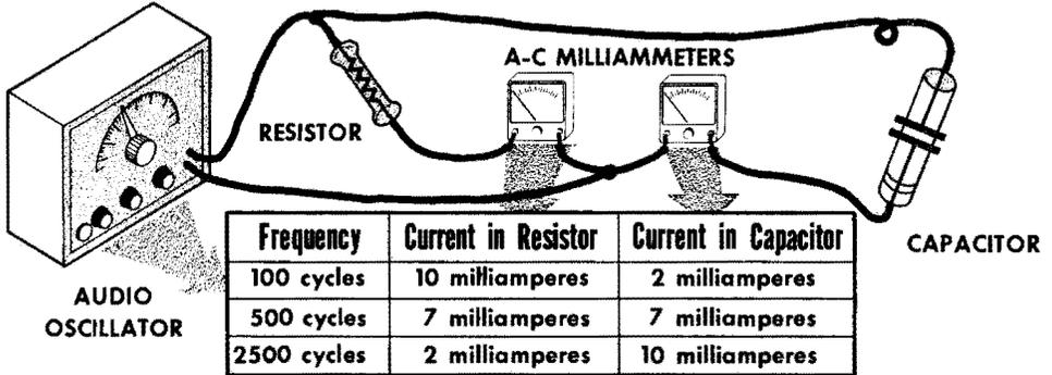
Currents of different frequencies can be separated by connecting the same components in parallel. With a resistor and capacitor in parallel, the resistor draws the current at low frequencies, the capacitor at high frequencies, and in the middle range, the current is shared. With a resistor and inductor in parallel, the resistor draws the current at high frequencies, the inductor at low frequencies, and in the middle range, the current is shared.
