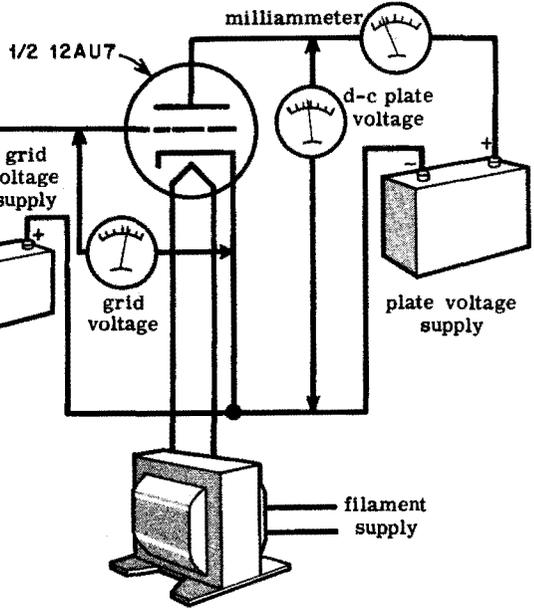
16. Set plate voltage (d-c) to 250, supply voltage reads: 355 volts current reads: 10.5 milliamperes
