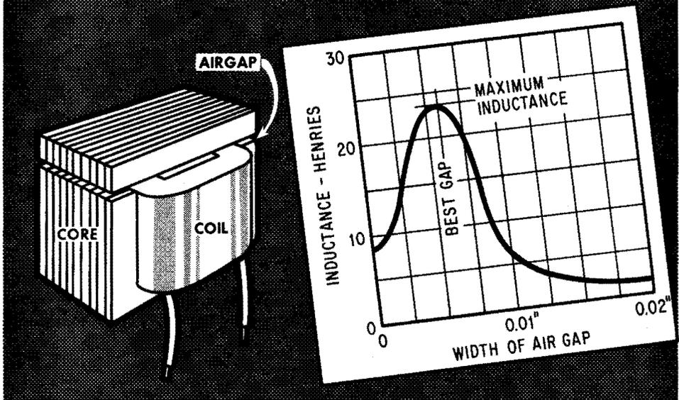
Using too small an air gap, or no air gap at all, means the primary current will cause the core to saturate and thus the inductance will practically disappear. Using too large an air gap amounts to making the transformer almost air cored, which again will result in a very low inductance. There is always an optimum size for the air gap, which will result in the biggest practical value of inductance for a transformer that carries direct current in one of its windings.
