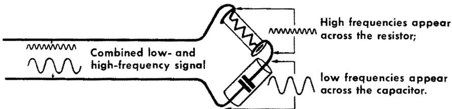
At a low frequency, the charge on the series capacitor follows the fluctuations, and the voltage across it very closely follows the input voltage, only a small current flows, and very little fluctuation appears across the resistor. At a high frequency, the charge on the capacitor does not have time to follow each fluctuation, and the whole of the applied voltage appears across the resistor.
