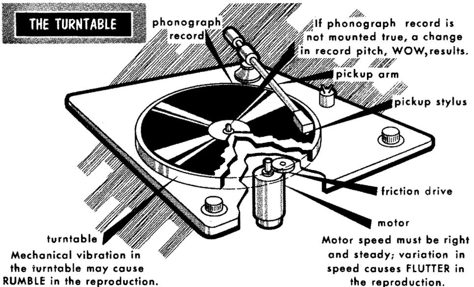
An effect most noticeable on phonograph recording, but entirely exclusive to it, is called *rumble*. This is caused by mechanical vibration in the turntable. The pickup stylus will be moved just as much by the whole groove vibrating as by vibrations that occur in the groove as it passes. Consequently any motor vibration that gets to the turntable will appear in the reproduction as rumble.
