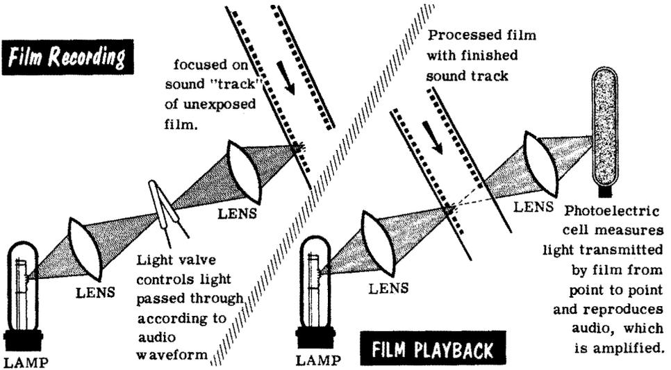
Film recording is usually achieved photographically by producing an exposure on the film proportional to the instantaneous audio. This is accomplished by means of a light "valve" that controls the amount of light falling on the film as it passes by a slot. In playback, the same film, with the recording photographically reproduced on it, is scanned by means of a photoelectric cell, the output from which is amplified by an audio amplifier.
