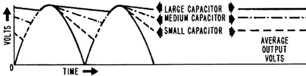
If the capacitor is not large enough to maintain this high a charge over the interval between consecutive half-cycle pulses, the voltage will drop away more during this interval, and the average output voltage will not be quite so high as the peak of the alternating waveform.
