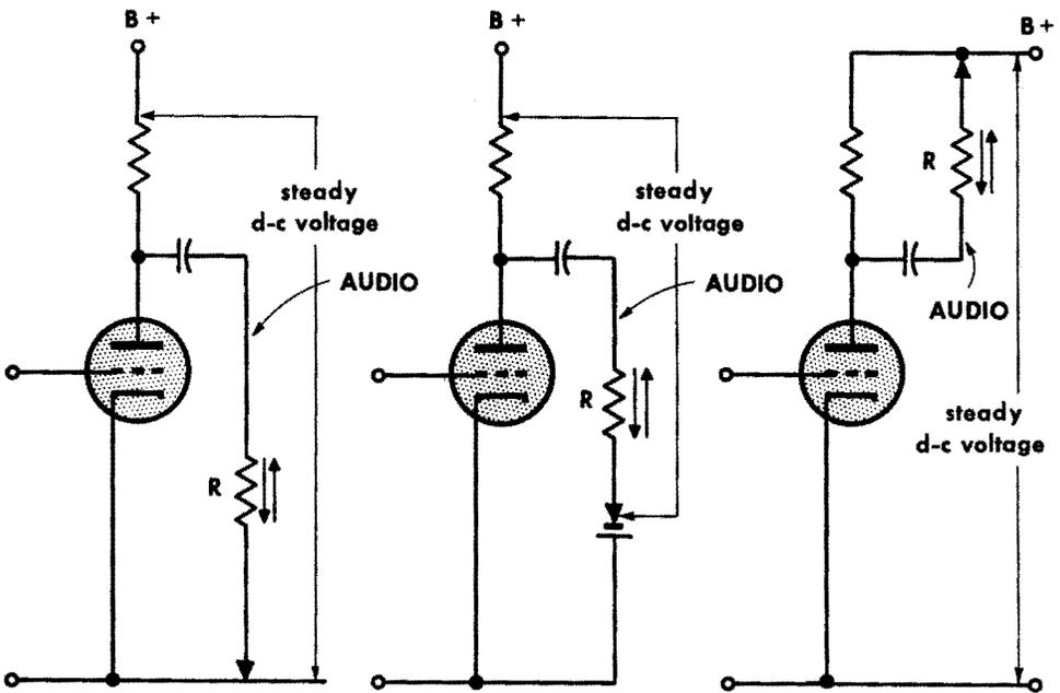
No matter where the other end of resistor R is connected, it takes the same current and voltage fluctuations from the plate
