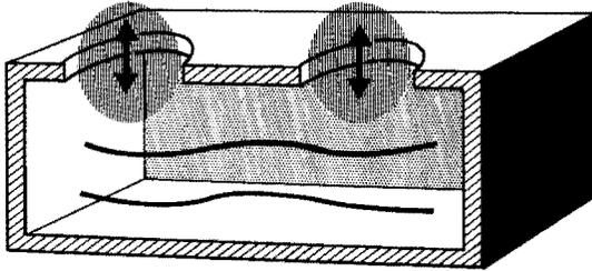
In a box with two holes, the air in the holes moves together
