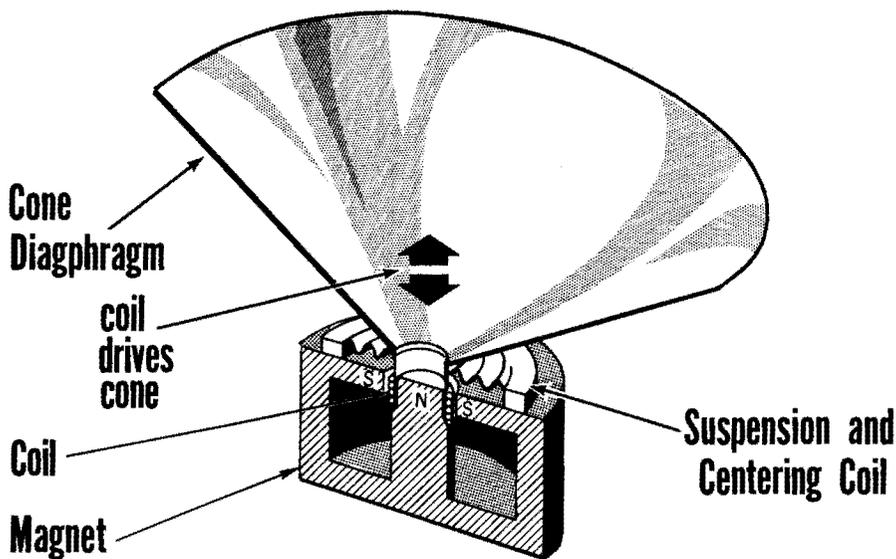
The use of a small coil requires a very intense magnetic field to get the best results. To accomplish this, the gap is made very small. To prevent the coil rubbing against the magnet poles, a centering "spider" or suspension is used, which allows free movement in the direction of vibration, while preventing the coil from moving against the pole faces.
