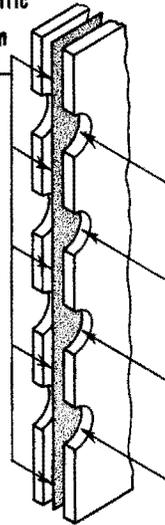
*the Electrostatic Speaker's Diaphragm Is Driven Almost Uniformly*
