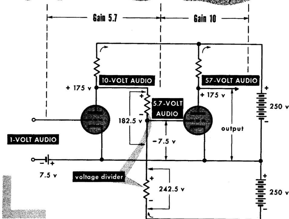
Another system that uses resistance coupling has just two supplies, one positive and one negative. To bring the voltage at one plate down to a suitable level for the following grid, two resistors are used as a voltage divider. Of course these resistors will divide the available fluctuation at the plate as well as dropping the steady voltage.
