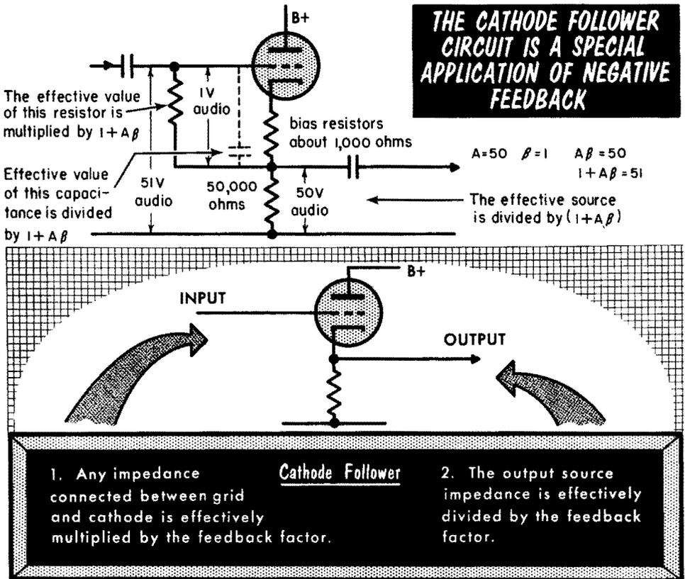
This characteristic makes the cathode follower a very convenient tool for reducing the output impedance of the amplifier. The output impedance in the absence of feedback would be the plate resistance in parallel with the plate load resistor, in this case, about 50,000 ohms. However this gets divided by the feedback factor (in this case 51) to give an effective resistance of less than 1000 ohms.
