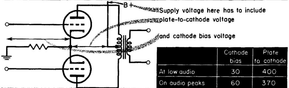
**NOTE:** This table assumes that B+ does not drop with increased current demand. If it does, reduction in plate-to-cathode voltage on peaks is even worse.
