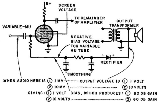
What this circuit does is to reduce the dynamic range of the program. Suppose that an input of 0.1 millivolt will produce an output of 1 volt, which biases the tube to 1 volt negative. This is not sufficient to change its transconductance, so the amplifier works at full gain — in this case, 10,000.
