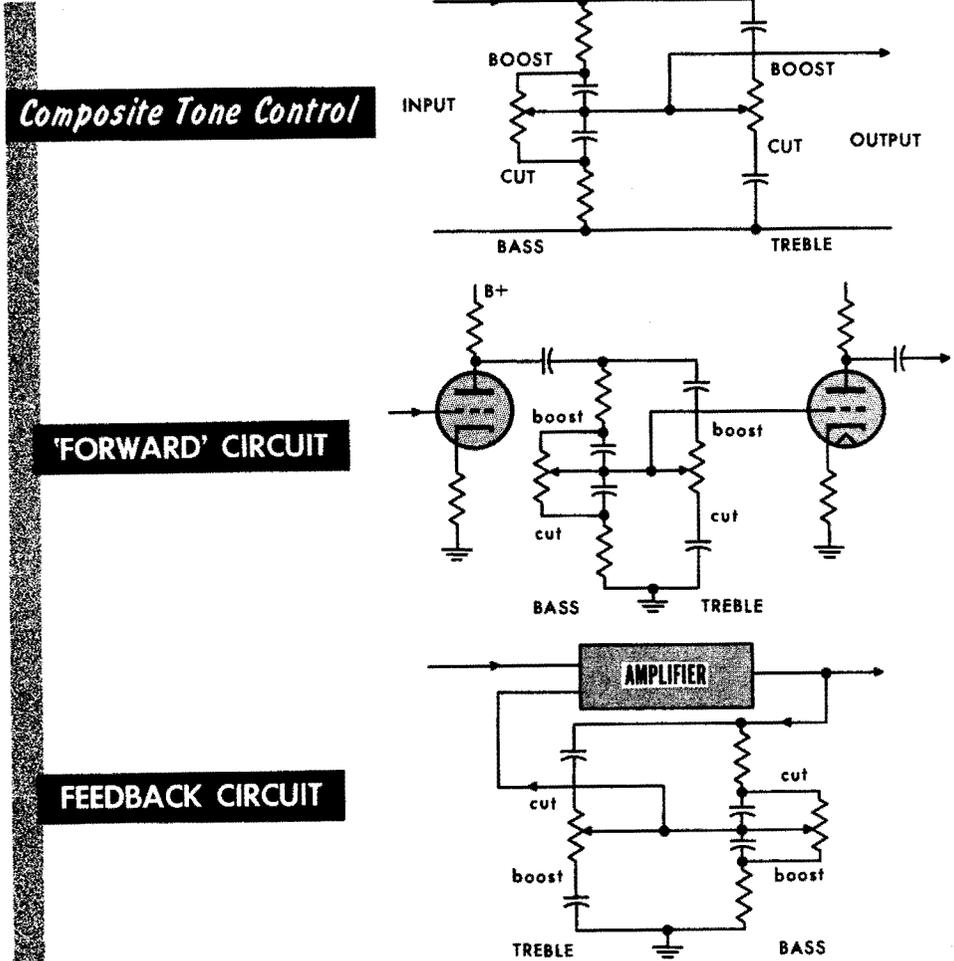
By combining the arrangement and using a potentiometer across the two capacitors, we provide a continuous adjustment that will go from bass boost to bass cut. Most modern tone control circuits combine the two arrangements with two controls, one for the treble boost and cut, the other for bass boost and cut.
