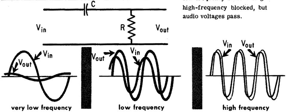
When the capacitance is in series, low-frequency audio voltages are high-frequency blocked, but audio voltages pass.
