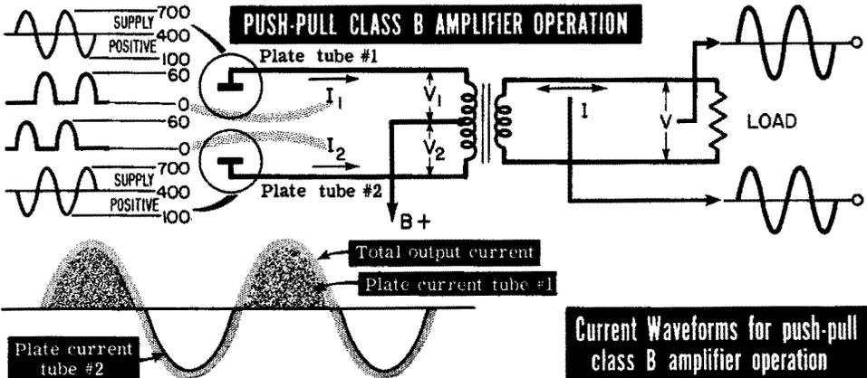
Current Waveforms for push-pull class B amplifier operation
