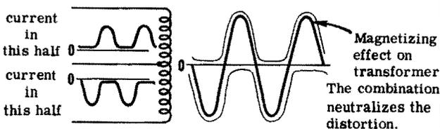
When audio signal is fed into output stage, current in one primary rises, while current in the other falls. On next half-wave, opposite primary currents rise and fall.
