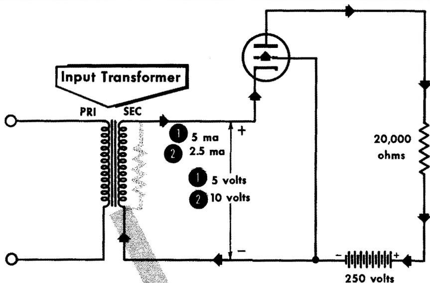
D.C. resistance of secondary must be  $\frac{7.5}{.00375} = 2000$  ohms
