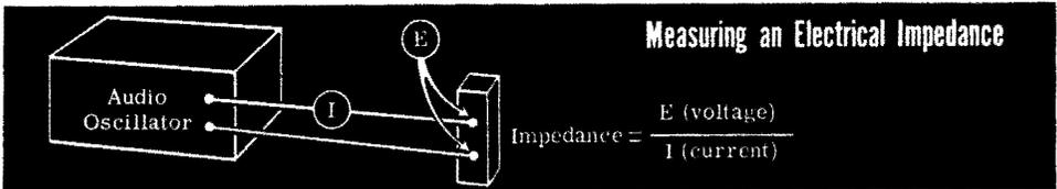
In a microphone, the voltage source is internal or *inside* the component, so that we cannot measure it separately. But we can measure the open-circuit voltage and then measure current when we short-circuit the microphone, so that there is no voltage. The relationship between this voltage and current is the impedance of the microphone.
