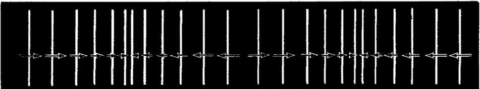
**At low frequencies (long wavelengths), large volumes of air are compressed and expanded, requiring large air movement.**
