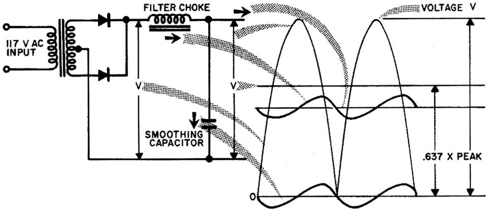
THE OUTPUT OF A CHOKE FILTER
