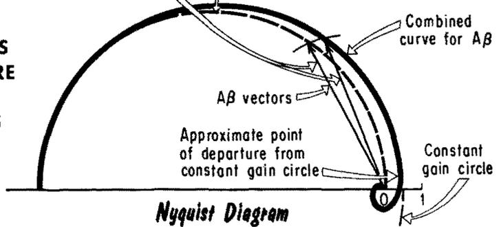
The best way of achieving this proves to be a choice in the combination of coupling capacitors values (for the low-frequency response) that causes one rolloff or 3-db point to occur at a much higher frequency than the other two (or more).
