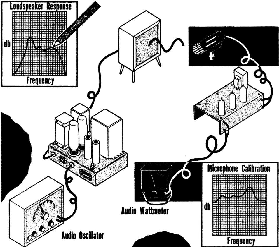
The response of a loudspeaker can also be found by using a calibrated microphone to measure the sound field that it radiates at different frequencies. For all these purposes, it is obvious that the calibrated, or secondary standard microphone should be as near perfect in response as possible, so that little correction will be necessary from its chart. High-quality condenser microphones and a special form of crystal microphone without any lever system, are favored for this purpose.
