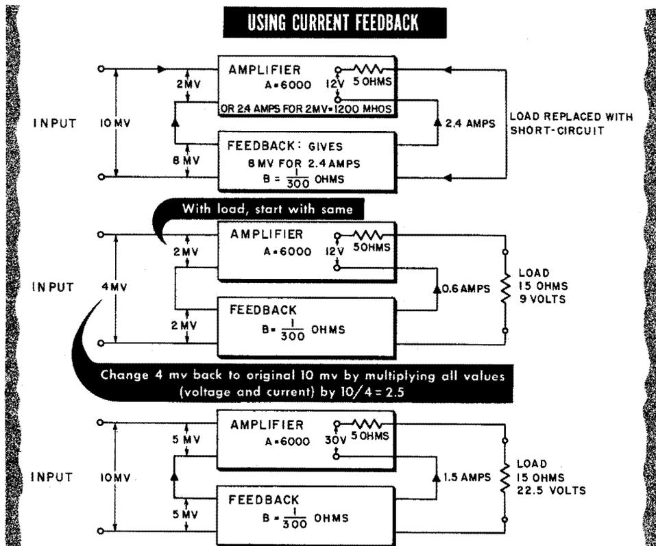
The other way in which the output can be sampled is called *current feedback*. Assume that we have an amplifier that without any load connected gives 12 volts output for an input of 2 millivolts. It has an internal resistance of 5 ohms. When the output is short-circuited, the internal resistance will be the only thing to limit the current— $12/5 = 2.4$  amperes. Assume that this 2.4-ampere output produces 8 millivolts of feedback and that the current feedback is always in this ratio.
