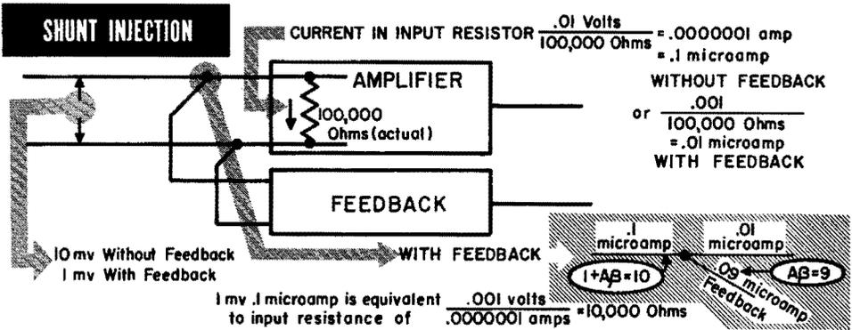
In shunt injection we must also consider the input current as well as the input voltage. Again assuming an input resistance of 100,000 ohms and an input current of 0.1 microampere, this would produce an input of 10 millivolts. However, the feedback current will provide 9/10 of the total input current in this case, or .09 microampere, leaving a current through the input resistance of only .01 microampere. This current would produce a voltage drop of only 1 millivolt.
