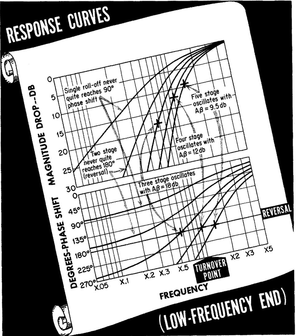
In this way the gain is reduced at the rate of 6 db for every octave with only a little more than 90° phase shift (because the other rolloffs are gradually starting) so it gets the magnitude of  $A\beta$  down to much less than 1 before the phase shift reaches 180°.
