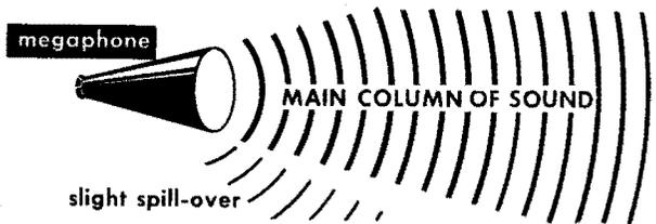
The directivity of a horn is dependent on its precise shaping. For example, a shape called the *tractrix*, which is nearly identical with the exponential shape, except at the mouth, is designed to produce hemispherical waves; in other words, to cover the entire 180° in front of its mouth. This ideal distribution from the tractrix only exists at the lower frequencies it radiates. At higher frequencies, the bell has progressively less effect.
