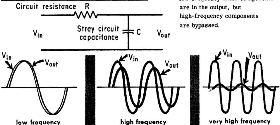
When capacitance is in shunt, low-frequency audio components are in the output, but high-frequency components are bypassed.
