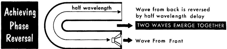
In normal propagation of sound, the only way to get the waves from the back turned around would be to take them for a half-wavelength longer journey than the waves from the front. To reproduce 50 cycles per second, this requires a propagation path of eleven feet, which can hardly be contained in a livingroom piece of furniture.
