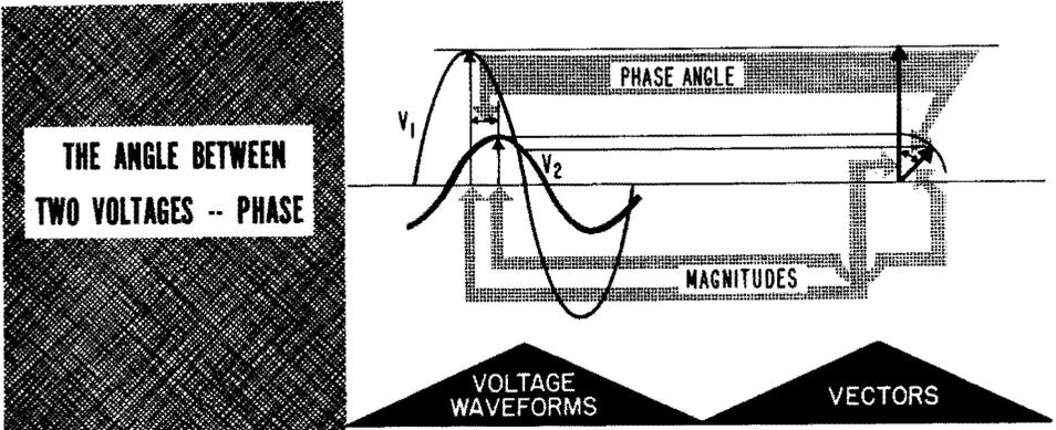
We are fortunate that this time difference between the voltage fluctuation at different points in an amplifier at various frequencies can be designated as a *phase angle*. This means that we can draw a “picture” of the voltage with what is called a *vector*. It is a line drawn at an angle to correspond with the phase angle from a starting point representing zero.
