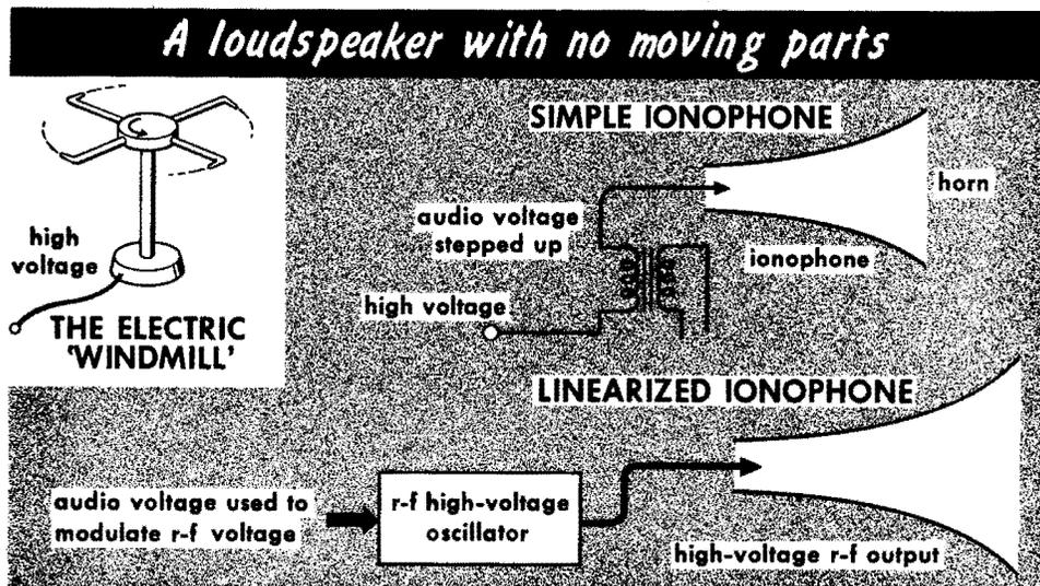
With every kind of loudspeaker, there has always been the problem of mechanical parts which can add effects of their own to the sound radiated. It has long been a dream among idealists in high-fidelity circles to find a loudspeaker which had no moving parts, but converts electrical waveforms directly into sound waves. For this reason the *ionophone* has a strong appeal.
