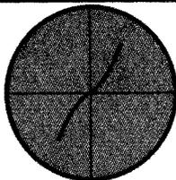
Two curved traces indicating wrong amplifier loading. Both are distorted sine waves.
