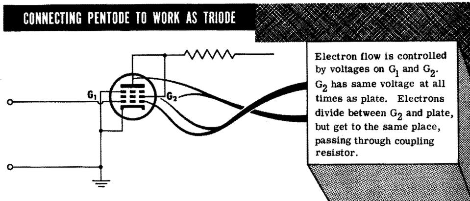
Any pentode-type tube can be made to work as a triode-type tube. This is done by connecting the second grid directly to the plate, so that both swing together at the same voltage. Because the screen grid, in combination with the control grid, is principally responsible for controlling the plate current, the presence of the suppressor grid between the screen grid and plate does not materially alter the tube's performance from that of a triode.
