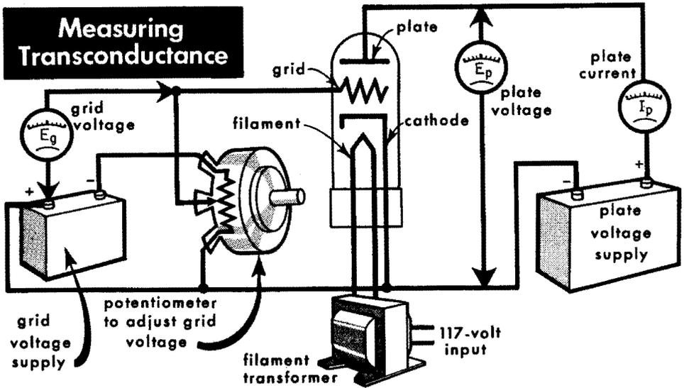
How is it that a small change in voltage at the grid can be converted into a larger one at the plate? Two things control how many electrons get away from the cathode of the tube: the plate voltage and the grid voltage. The number of electrons flowing inside the tube fixes the current in the outside circuit. Using a fixed plate voltage, the grid voltage can be changed and plate current measured each time it is changed.
