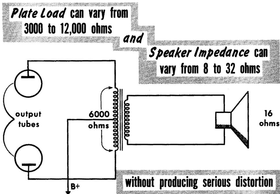
If, for example, the plate load of the two tubes in push-pull should be 6000 ohms, they will not show serious distortion if an actual plate load is used ranging from 3000 to 12,000 ohms, or even more. In terms of the secondary side of an output transformer designed to feed a 16-ohm loudspeaker, it will not produce serious distortion even if it is connected to an 8-ohm or 32-ohm loudspeaker.
