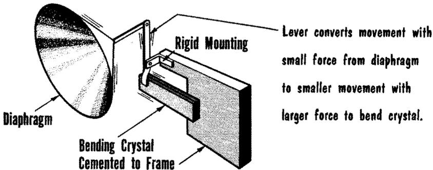
This double crystal is still much too stiff for use as a microphone. For this reason, the diaphragm is coupled to the crystal by a lever action, which transforms a larger movement with smaller force to a smaller movement with a larger force at the crystal. In this way, the tiny movements of air particles in contact with the diaphragm are efficiently coupled to the crystal element to produce as sensitive a microphone as any other.
