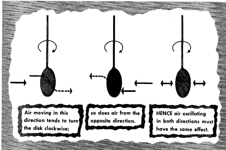
When a small disk is suspended in air, any air movement striking it tends to set the disk "head on" to stop the air. This happens whichever side the movement comes from. In a sound wave, the movement comes alternately from opposite sides, as air particles move back and forth. Both movements tend to turn the disk the same way, hence the torsion on the disk will depend on the *amount* of air particle movement, not its direction or frequency.
