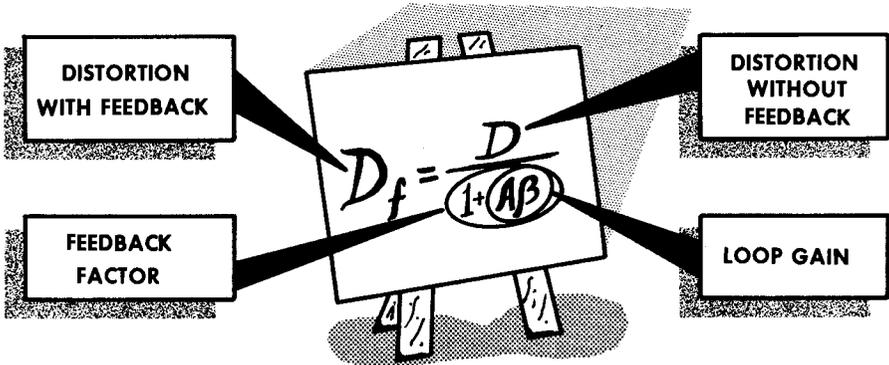
This is the formula for *negative* feedback, because the sample fed back from the output is in the *opposite* direction or phase from the input. In addition, feedback can also be *positive*.
