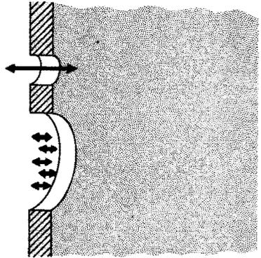
*Putting a diaphragm over a smaller hole increases the effort to move the air and reduces diaphragm movement, improving efficiency in converting voice-coil force to air movement*
