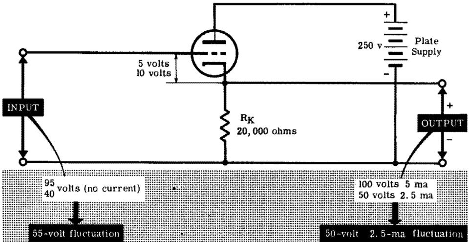
The third way to connect a tube makes the plate common. We do this by connecting the 20,000-ohm resistor in the cathode circuit. Now the change of  $-5$  volts to  $-10$  volts between grid and *cathode* results, as before, in a change in current through the tube between plate and cathode, from 10 milliamperes to 5 milliamperes. Thus the cathode will fluctuate between 100 volts and 50 volts, respectively, due to the different currents flowing in the 20,000 resistor.
