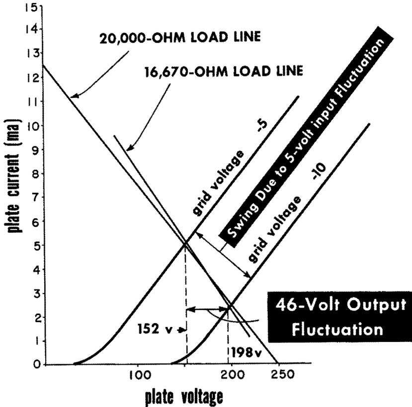
Joining these points and extending the line we can find the new values of plate voltage corresponding to fluctuation of grid voltage between  $-5$  and  $-10$ . The new voltages, instead of  $150$  and  $200$ , as on the  $20,000$ -ohm load line, are now  $152$  and  $198$  volts. Thus a  $5$ -volt input fluctuation yields a  $46$ -volt output fluctuation. The gain is  $46/5$  or  $9.2$ , instead of the  $10$  obtained before.
