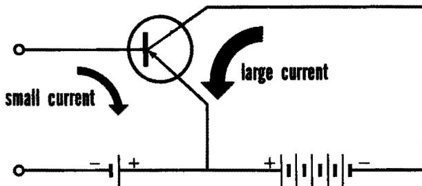
A small current and voltage change in the base circuit produces a much larger Current Change in the collector circuit.
