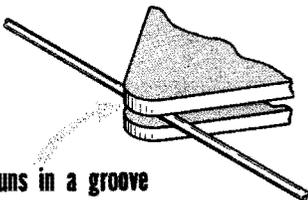
Wire runs in a groove in the 'head,' which otherwise is like tape head.
