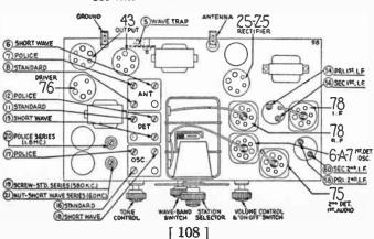
\* Use a 200-mmf. condenser in series as a dummy antenna on broadcast band and a 400-ohm carbon resistor on the shortwave band.
