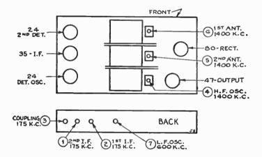
Connect a 200-mmf. condenser between signal generator and antenna post of set, at the antenna post.
