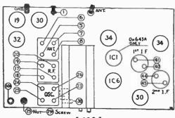
\* Use a 200-mmf, condenser as dummy antenna on broadcast band and a 400olim carbon resistor on shortwave band.
