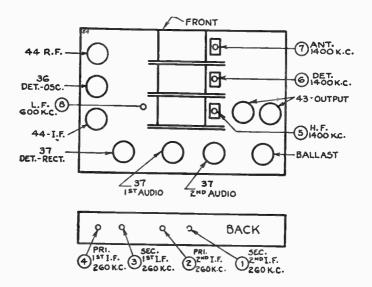
Connect a 200-mmf. condenser between signal generator and antenna post of set, at the antenna post.
