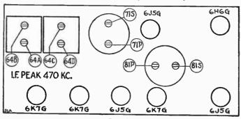
Note 5.—Connect signal generator direct to transmission line terminals. Note 6.—Set magnetic-tuning control in "off" position and fidelity-selectivity
