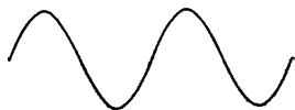
Fig. 66. Here the high-frequency carrier has been removed and the audio voltage shown actuates the loud speaker.
