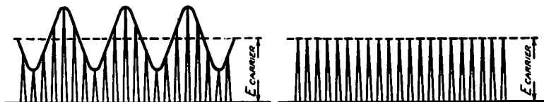
Figs. 19, left, and 20. The average value of the carrier voltage is the same, whether the signal is modulated (Fig. 19) or unmodulated (Fig. 20).
