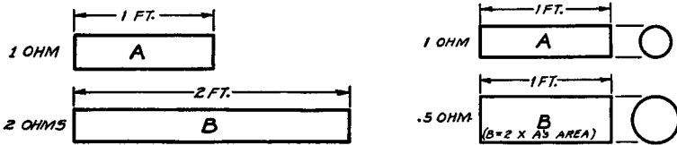
Fig. 3, left, Fig. 4. The resistance of a wire is directly proportional to the length, see Fig. 3, and it is inversely proportional to the cross-sectional area, see Fig. 4.
