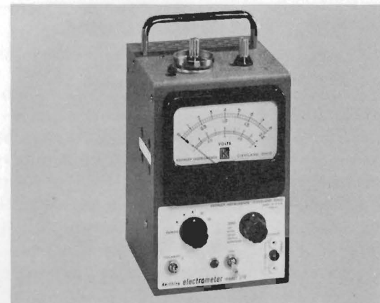
Fig. 14-6. Electrometer. Keithley model 210
