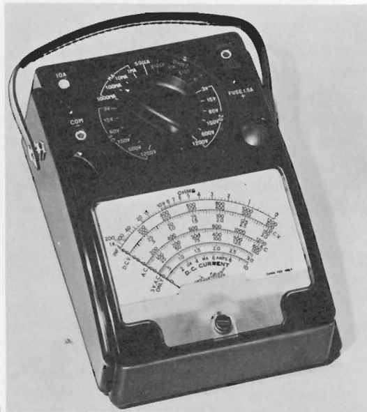
Fig. 15-3. Burnout-proof multimeter. Hickok model 455
