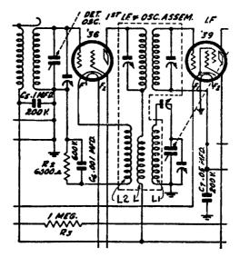
Fig. 32. An example of a screen grid tube used as a mixer and oscillator (Courtesy Electric Auto-Lite Co.)
