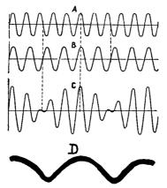
Fig. 4. Curve A, 11 cycle wave; Curve B, 9 cycle wave; Curve C, composite wave; Curve D, waveform of complete cycle of amplitude variation, which becomes beat note when Curve C, is acted upon by mixer tube
