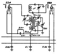
Fig. 36. Note coil assembly between the two tubes. The plate feed back coil—the lower portion of those in the plate circuit—is the only one coupled to the oscillator circuit. See Fig. 37 for coil arrangement
