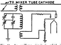
Fig. 41. An oscillator circuit in which is included a "tank"
