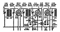
units. Namely, the primary and one secondary winding is resonated to the i-f peak, so that as far as far as alignment is concerned, these special transformers are handled just as if they were standard units.
