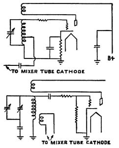
Figs. 38, 39. Examples of feed back oscillator circuits
