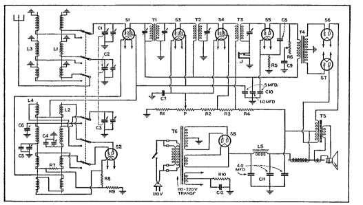
Fig. 23. Superheterodyne with linked multi-wave radio-frequency arrangement. See three upper coils on the left
