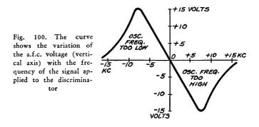
applied to the control tube. When this bias is negative, the frequency of the oscillator is lowered, and similarly, when the bias is made more positive, the frequency of the oscillator is raised. As a result of this connection between the discriminator circuit and the oscillator frequency, the a.f.c. voltage acts to maintain the frequency of the oscillator so that the signal will always pass through the i-f. amplifier at the i-f. peak.
