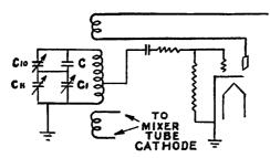
Fig. 40. Good tracking of the condensers is assured by the arrangement here shown
