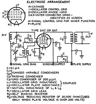
Fig. 45, above. Element arrangement of a-c. pentagrid tube Fig. 46. In this circuit the coupling between the mixer and oscillator is electronic
