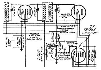
Fig. 60. A typical example of a diode detector used as a combination demodulator and AVC tube. Note that plate and cathode are connected (Courtesy Fada Radio)
