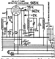
Fig. 48. A temperature controlled condenser, C-40, prevents frequency drifting in the oscillator circuit (Courtesy Stromberg Carlson)
