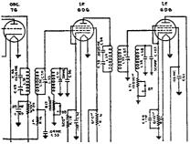
Fig. 97, left. By varying the 10,000-ohm rheostat in series with the third winding of the i-f. transformers, the degree of selectivity is controlled. When maximum selectivity is desired, the switch in this circuit is opened (Courtesy Stromberg-Carlson Tel. Mfg. Co.)
