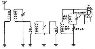
Fig. 24. The double-spot circuit for minimizing image frequency interference
