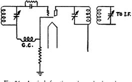
Fig. 26. A single-function mixer circuit using a triode
