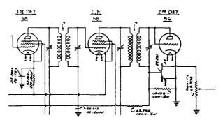
Fig. 61. Another AVC and demodulator combination. Note that the grid and plate are connected (Courtesy Zenith Radio Corp.)
