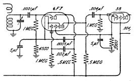
Fig. 62. The 6F7 is used here as a demodulator and a-f amplifier. This is not a reflex circuit (Courtesy Emerson Radio)
