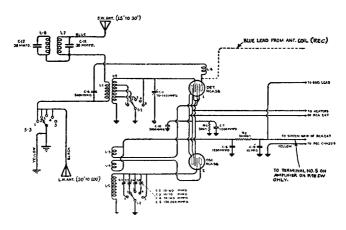
Fig. 11. A-c. superheterodyne converter for four wave bands
