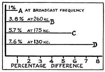
Fig. 14. The apparent increase in adjacent channel selectivity due to frequency conversion
