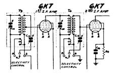
With the coupling between primary and secondary at a minimum, the selectivity of the circuit is greatest and the selectivity of the i-f. amplifier decreases progressively as the coupling is increased.
