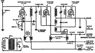
Fig. 9. Short-wave superheterodyne converter (Courtesy RCA-Victor Co.)
