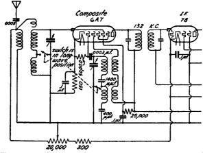
Fig. 49. Oscillator coils are connected to grids 1 and 2, the the latter acting as the oscillator plate (Courtesy Emerson Radio & Phonograph Co.)
