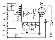
Fig. 42. The sliding switch determines the proper amount of inductance for this oscillator
