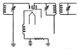
Fig. 27. A single-function mixer circuit employing a screen-grid tube
