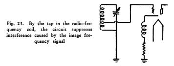
successfully suppresses the image frequency. Naturally the position of the tap is governed by the circuit constants and the intermediate frequency used in the receiver.
