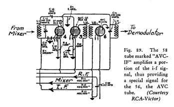
the regular demodulator in the receiver. The first i-f amplifier tube and the AVC amplifier have their grids inter-connected through a .0003 mfd condenser, so that the i-f signal from the i-f transformer is applied to the i-f amplifier and
