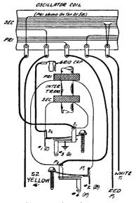
Fig. 37. Physical arrangement of oscillator and I-F coils shown in Fig. 36 (Courtesy U. S. Radio & Television Corp.)
