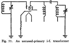
Fig. 55. An untuned-primary i-f. transformer having capacitative coupling between the windings
