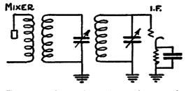
Fig. 54. A three-winding i-f. transformer with untuned primary
