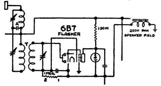
Fig. 57. Flasher circuit incorporated in the i-f. amplifier (Courtesy Colonicl Radio Corp.)
