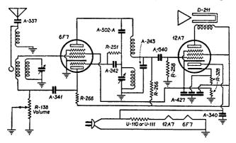
Fig. 88. The 6F7 is an r-f and a-f amplifier and detector and the 12A7 is an output pentode and half-wave rectifier. (Courtesy International)
