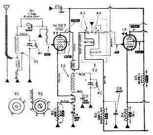
Fig. 35. Note coil arrangements in tank circuit (Courtesy Atwater-Kent)
