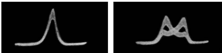
Figs. 291, left, 292, right. Both the resonance curves shown here have their lines broad because of the presence of an appreciable amount of carrier voltage.
