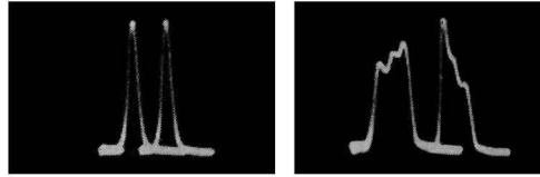
Figs. 314, left, 315, right. The effect of over-synchronization is shown in these two resonance curves. Compare them with those of Figs. 265 and 270.
