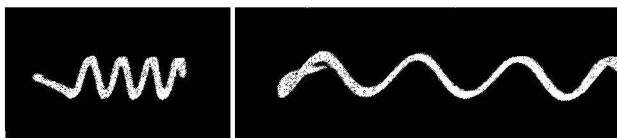
Fig. 86, left, Fig. 87, right. The same wave is shown in both illustrations with the same vertical deflection voltage applied. The horizontal deflection voltage has been increased in Fig. 87, so that the wave appears to be much flatter.
