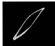
Fig. 146, left, Fig. 147, right. The amount of saturation in these two oscillograms is appreciably less than that shown in Figs. 142 to 145. The core loss due to hysteresis, indicated by the size of the area enclosed by the curve, is fairly large in Fig. 147.
