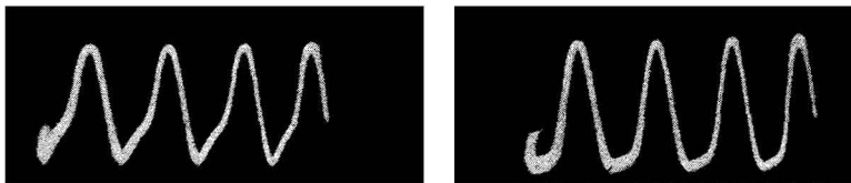
Figs. 204, left, 205, right. Further changes were made in the value of C of Fig. 201. When it was increased to .01 mf. the wave shown in Fig. 204 was obtained and when it was made .05 mf., the waveform of Fig. 205 was obtained. Note the similarity of this wave to the original, which is shown in Fig. 202.
