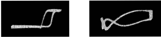
Fig. 139, left, Fig. 140, right. The oscillogram of Fig. 139 was made at 40 cycles and that of Fig. 140 was made at 1000 cycles. The phase shift present in these patterns is clearly evident. Compare Figs. 129 to 133.
