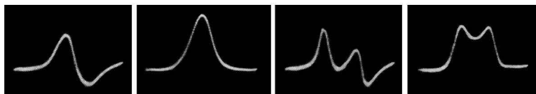
Figs. 286-A, 286-B, 287-A, 287-B, from left to right. The oscillograms of Figs. 286-A and 287-A show phase distortion in single peaked and double peaked curves, respectively. Correct corresponding curves with no phase distortion are shown in Figs. 286-B and 287-B.
