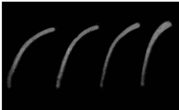
Fig. 37. This waveform is the result of applying the bias necessary to produce maximum amplitude of the sweep. Note the very definite bend in the charging portion of the cycle and the consequent non-linearity.
