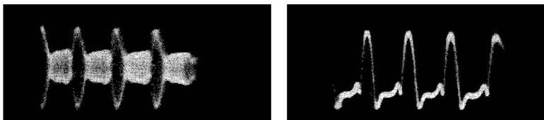
Fig. 235-A, left, Fig. 235-B, right. A. The modulated output waveform of the same oscillator used for generating waves shown in Fig. 234. The frequency here is 600 kc. B. The a-f. signal resulting from demodulation of A.
