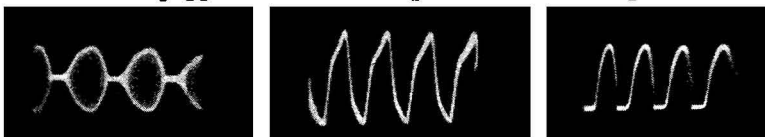
Fig. 232-A, left, Fig. 232-B, middle, Fig. 232-C, right. A. The wave envelope of the modulated output of a commercial test oscillator. B. The a-f. output of the same oscillator. C. The a-f. signal resulting from demodulation of the modulated wave shown in A.
