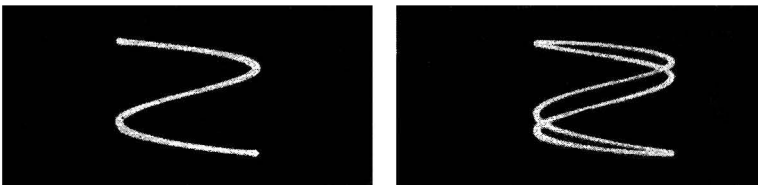
Fig. 97. A, left, B, right. A 3-1 ratio pattern is shown in both illustrations. The pattern in A was taken when the phase difference between the two voltages was 0°.
