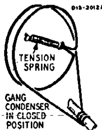
New dial cord stringing for Montgomery Ward model 74WG-1801C.
