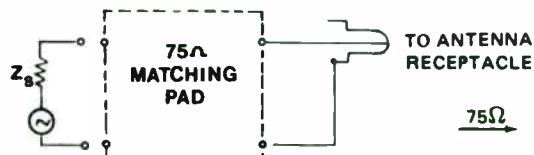
Figure 9. FM Dummy Antenna. (Use Matching Pad if signal generator Z_s is other than 75 ohms.)
