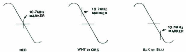
Figure 8 – 10.7 MHz marker position for each of five different ceramic IF filters that may be used in production.
