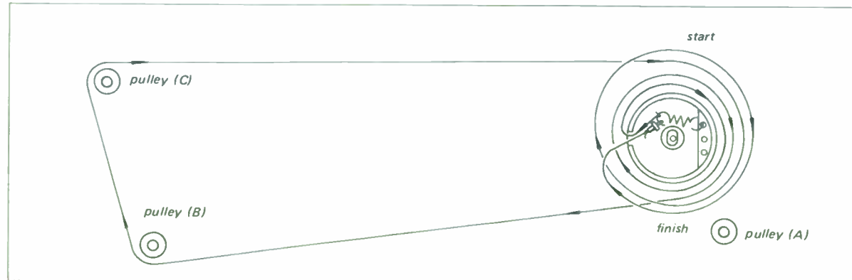
Fig. 2-19 Dial pointer driver cord stringing
