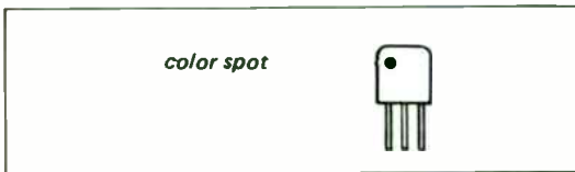
Fig. 3-1 Fm i-f ceramic filter
