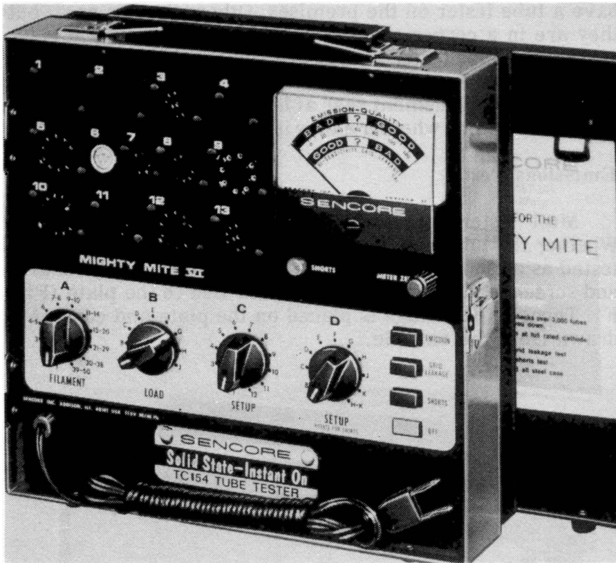
Emission-type tube checker also reveals shorts and leakage. Sencore Model TC154.
