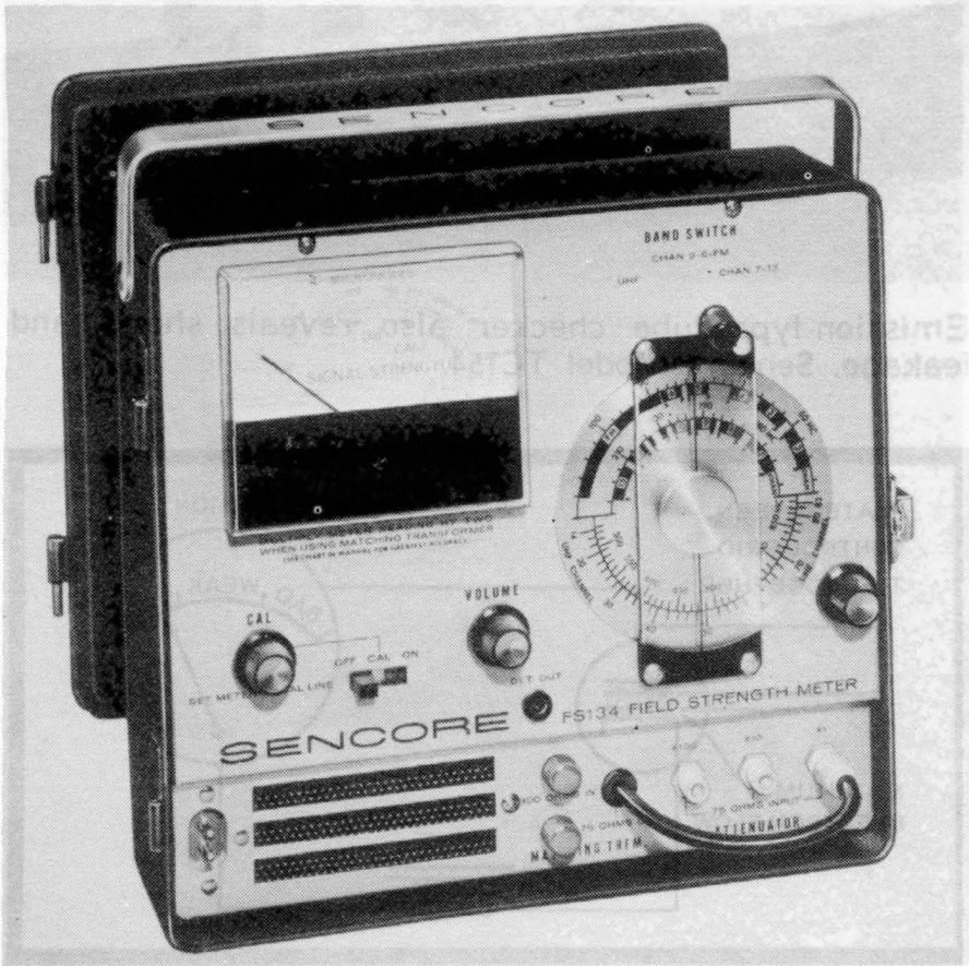
Field strength meter for all TV bands and the FM broadcast band. Sencore Model FS134.
