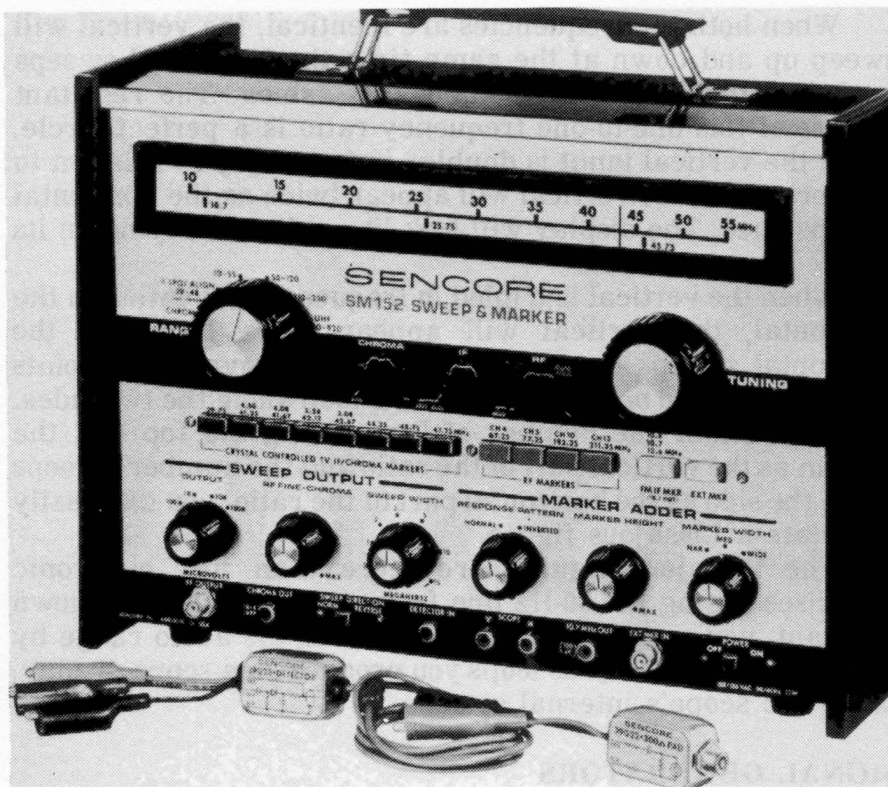
Sencore Model SM152 sweep and marker generator designed for TV sweep alignment.
