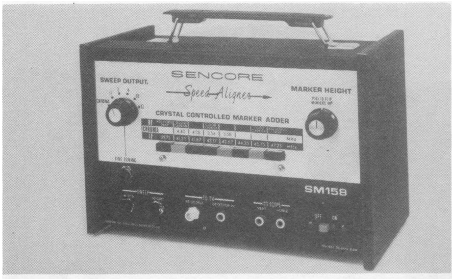
Marker generator, Sencore Model SM158, provides signals for TV IF, chroma and RF alignment.
