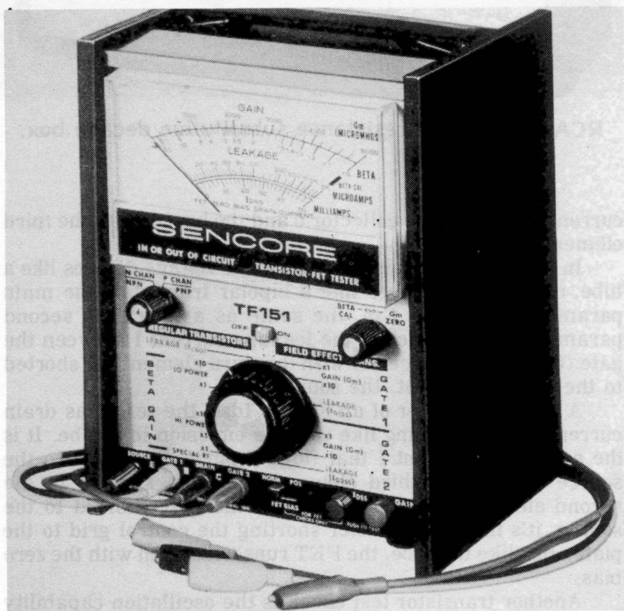
Sencore Model TF151 transistor tester designed to check bi-polar and field-effect transistors.
