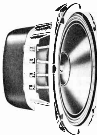
Fig. 6-33. A typical dual voice-coil unit for use as middle speaker in a stereo arrangement.
