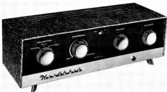
Fig. 4-39. An adaptor to convert tuners for reception of FM multiplex transmissions.
