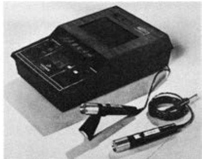
(Q) Fisher RC-80B stereo cassette recorder with Dolby system and provision for chromium-dioxide tapes.
