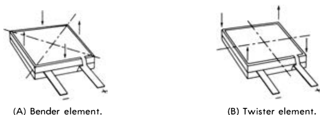
Fig. 4-5. Construction of crystal elements.
