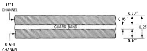
Fig. 3-11. Tracks on two-track stereo tape.
