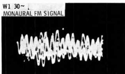
Fig. 3-19. The monophonic FM signal present at point A.
