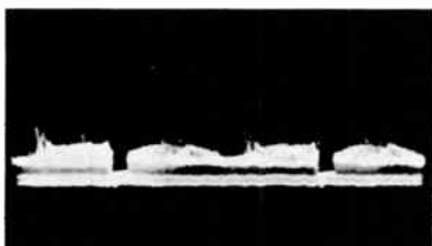
(A) Caused by loss of AGC.
