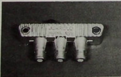
Fig. 6-28. Coaxial cable switch.
