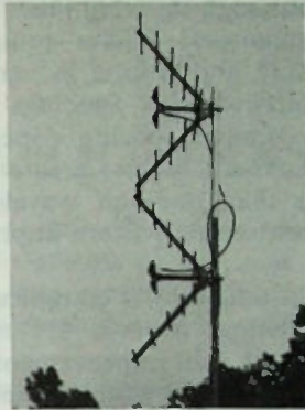
Fig. 8-6. Vertically stacked uhf antennas.
