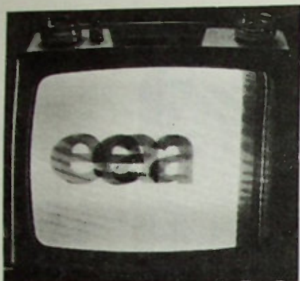
Fig. 1-1. Television picture with multipath interference.
