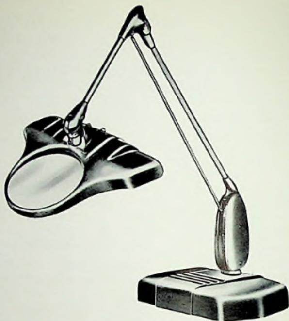
Plate 10. Various types of magnifying lenses which are useful when working with transistors. The top one houses a fluorescent lamp to illuminate the work (Severn Lighting Ltd.)
