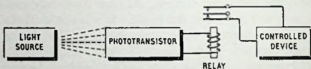
Fig. 12.2—Because the phototransistor supplies more output current, it can operate the relay directly, without the necessity of using an amplifier stage
