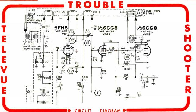
IF THE A.G.C. VOL-TAGE WERE TOO LARGE THE FRONT END AND SOME VIDEO I.F. TUBES WOULD BE CUT OFF. THIS WOULD PREVENTANY SIGNAL FROM PASSING, AND LOSS OF PIX AND SOUND WOULD RE-SULT. THE FIRST FEW CHECKS ASSUME THAT THE SET IS AN INTERCARRIER. IF IT ISN'T THEN NO NEED TO CHECK SOME OF THE I.F.'s OR VIDEO
