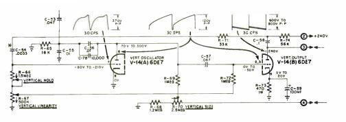
★ C.54, A.0033 MFO CONDENSER, HAS BEEN RELOCATED (TO PREVENT POSSIBILITY OF VERTICAL ORIFT DURING WARM-UP) AND IS HORIZONTALLY MOUNTED ON ETCHED CIRCUIT BOARD, (SEE FIG. #4, PG, 4)
