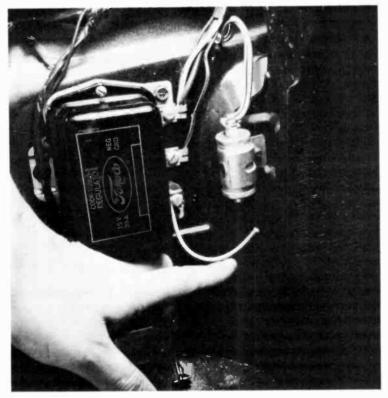
Fig. 6-4. Generator bypass capacitor.
