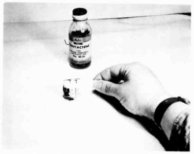
Fig. 9-2. Cleaning send-receive relay contacts.
