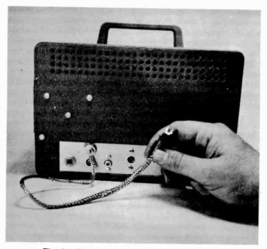
Fig. 6-1. Ground lead connected to transceiver.
