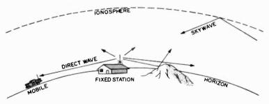
Fig. 5-1. Behavior of CB radio waves.
