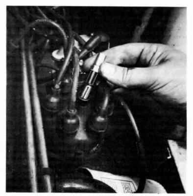
Fig. 6-3. Installation of distributor suppressor.
