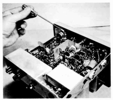
Fig. 9-6. Click test with screwdriver tip applied to control lugs.
