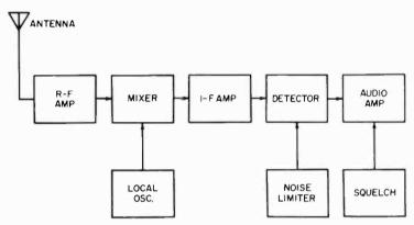
Fig. 4-2. Block diagram of a superheterodyne receiver.
