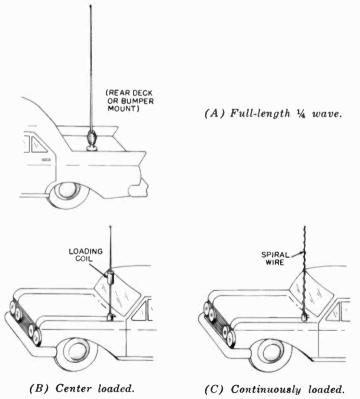
Fig. 5-4. Basic mobile whips.
