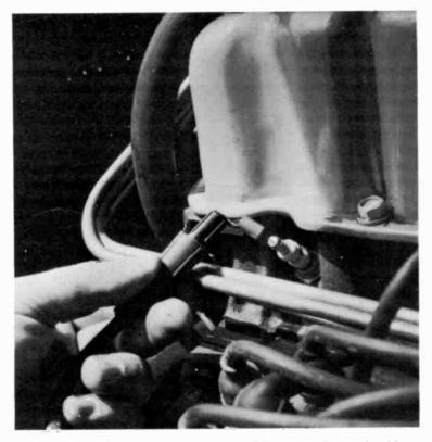
Fig. 6-2. Spark-plug suppressor clipped between plug and cable.
