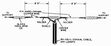
Fig. 5-2. Construction detail of dipole antenna.
