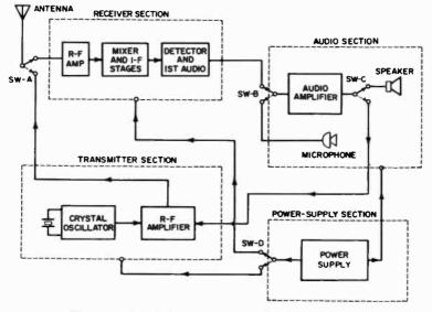
Fig. 4-1. Block diagram of a typical transceiver.
