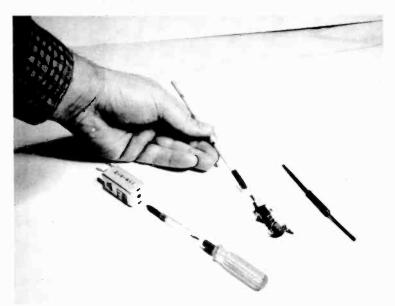
Fig. 7-1. Alignment tools for CB equipment.
