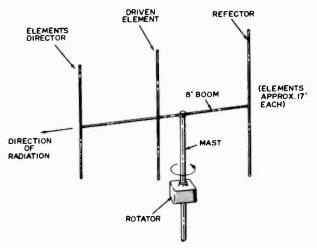
Fig. 5-5. Vertically polarized 3-element directional beam.
