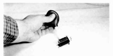
Fig. 9-7. Rubber bulb is useful for blowing out dirt.
