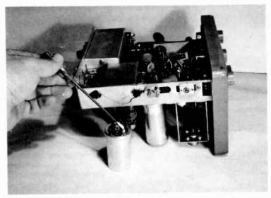
Fig. 9-1. Shorting filter capacitor to prevent shock.
