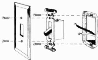
Fig. 3-4. Replacing a toggle switch.
