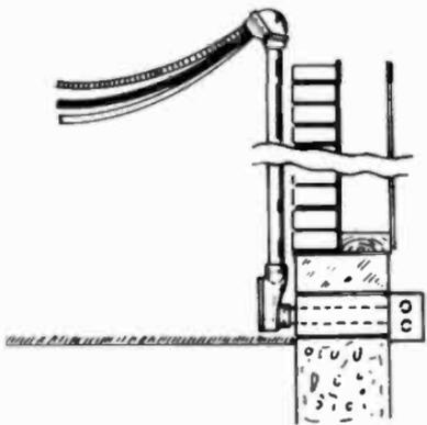
Fig. 5-1. To get power to overhead wires you must install fully enclosed and watertight conduit and fittings. From inside junction box, a short piece of conduit goes through foundation to right angle elbow, through vertical conduit, and out special service head.
