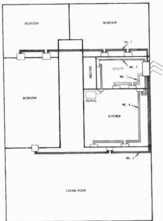
Fig. 1-7. Sample of possible distribution of circuit branches from the central control box. Central heating and refrigeration are separately fused to prevent interruption of these vital services in case of trouble elsewhere in the house. Kitchens should have their own lines because of the heavy loads of high-wattage appliances frequently used in the kitchen.
