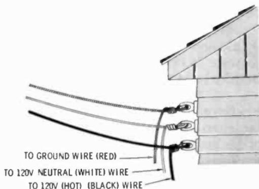
**Fig. 5-2.** Bring overhead wires through saddle insulator and wrap several times around horizontal portion of wire. The extra ground wire does not carry current, but merely completes the ground system.
