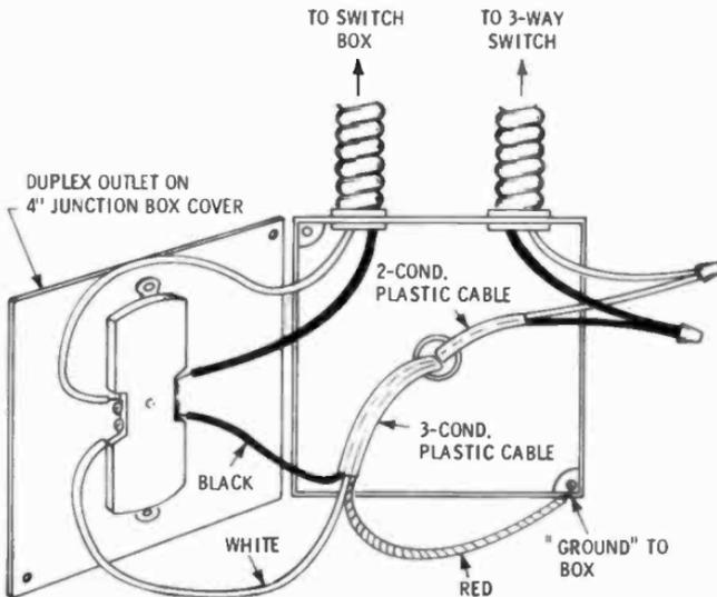
**Fig. V-5. Connections at garage cable input. It includes a duplex outlet at the entrance junction box.**
