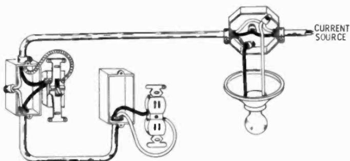
Fig. 4-7. Wiring system when the feed line comes into the ceiling fixture box. Note the three wires from the fixture to the switch. If the feed line comes into the outlet box, only two wires would be needed between switch and fixture.
