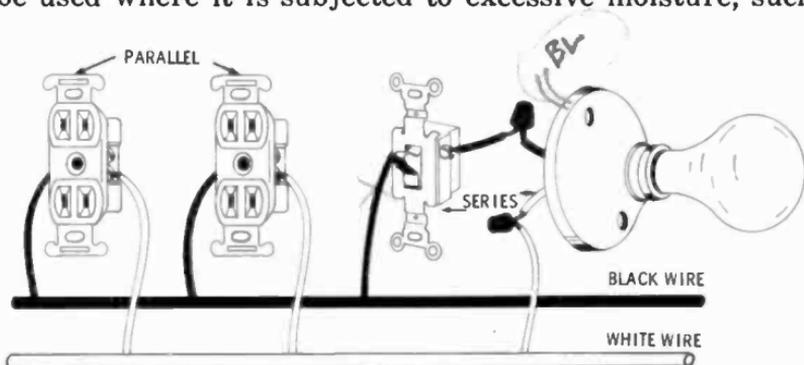
Fig. 4-8. Duplex outlets are connected in "parallel" across the line. Switches are connected in "series" with the light or outlet they control, and the combination is connected in parallel across the line.
