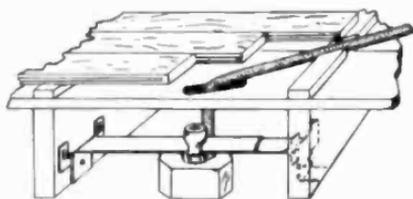
Fig. 4-1. A ceiling box is supported by an adjustable bracket nailed to the rafters. The lower edge of the box must be flush with the surface of the finished wall. Note the long slot cut into the rough floor, to take the gradual bend of the conduit.
