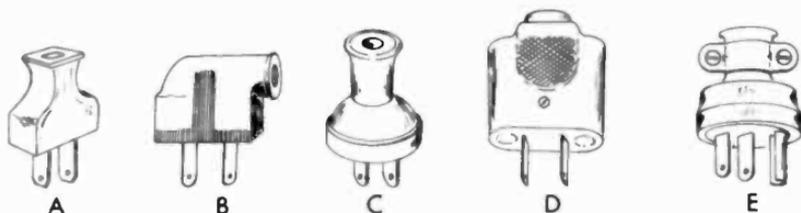
Fig. 3-1. A few representative plugs used as replacements on line cords.
