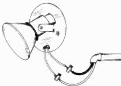
The box must have a black and a white wire coming into it for a source of power. Splice the white wire from the conduit you installed to the white wire in the box. The black lead from the conduit connects to one side of the new switch installed. The other terminal of the switch is "jumpered" to the terminal of the other switch to which the black wire already in the box is connected. Install the second switch to the same wires removed from the original switch (Fig. IV-5).
