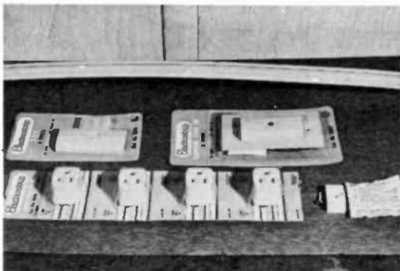
Fig. III-2. Parts used in the surface-wiring project. At top is the plastic strip with wires molded in. The center pieces are a "tee" and a "feed-in." The stripped ends of the cable plug into these fittings. The "feed-in" makes connection to the wires in your outlet box. Bottom row shows snap-on outlets and end-cable finishing pieces at right.
