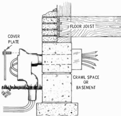
the vertical sections of the thin-wall conduit and out through the elbows. Make the bend at the bottom of the thin-wall sections as gradual as you can to prevent the edges of the conduit from cutting into the plastic. At the entrance elbows, bend the cable and push them through into the house at one end, and into the garage at the other end (Fig. V-2). Leave enough cable out the junction boxes to work with. Put the covers back on the elbows. Push the dirt back into the ditch and tamp it down.
