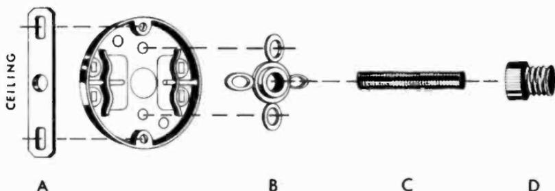
Fig. 2-17. Fittings used to hang fixtures from ceiling boxes. *A* is a strap for fixtures, that mount with two wide-spaced screws. *B* is a stud that screws to the box and accepts the nipple at *C* and is used on center-bolt mountings. *D* is an extension nipple.
