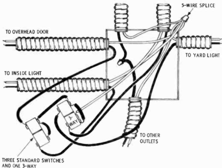
**Fig. V-6. Distribution junction box with three-way switch plus three individual light switches.**
