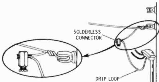
**Fig. 5-3.** A wire drip loop must be formed when connecting the overhead wires to the wires coming from service head.
