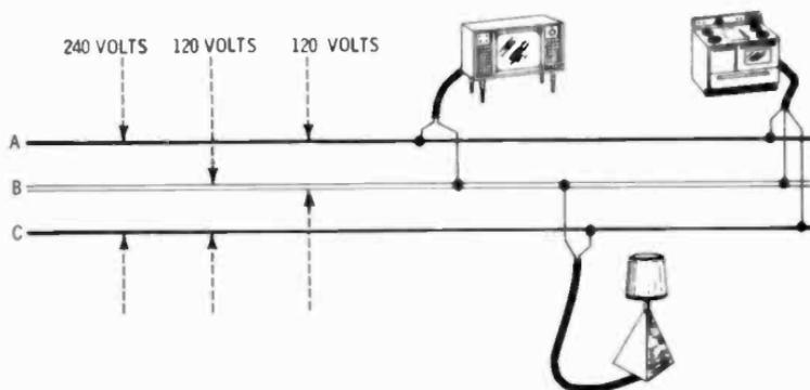
Fig. 1-2. The three-wire service now brought into most homes supplies 240 volts for electric ranges and other high-wattage appliances, and two branches of 120-volt service.
