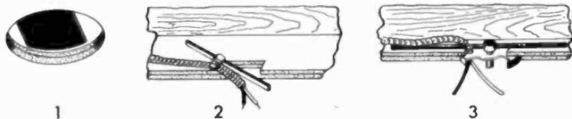
Fig. 4-14. In concealed ceilings a shallow 4-inch round box is fastened to the outside. (1) Cut a round hole slightly smaller than the box. (2) Slip a long bar with a stud and nipple at its center into the cutout. Center the stud over the cutout. (3) Fish the cable through and couple it to the junction box. Place the box slowly up against the ceiling and maneuver the nipple through the center hole. Place a locknut on the nipple and tighten.
