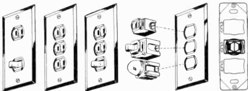
Fig. 2-9. A pilot light, a toggle switch and an outlet are available in what is called "interchangeable" devices. They may be used in any combination of two or three. They crimp to a special plate (shown at right) for mounting to an outlet box.
