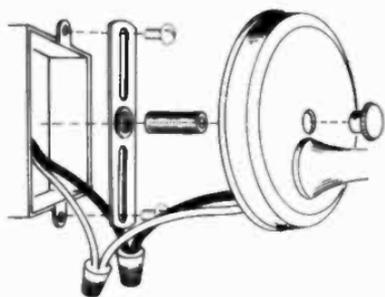
**Fig. 3-8.** Wall fixtures are frequently mounted to the smaller outlet- or switch-type boxes. If the fixture has a center nipple, obtain a bracket that has a threaded hole in the center to take the nipple.
