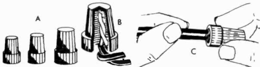
Fig. 2-16. Solderless connectors called "wire-nuts" are used exclusively today to splice wires together for indoor wiring. *A* shows three sizes but there are many, depending on the size and number of conductors being spliced. *B* shows the internal construction. Internal threads twist the wires together. *C* shows how simple it is to make a splice with a wire-nut. Just insert the two wires, and turn the connector clockwise.
