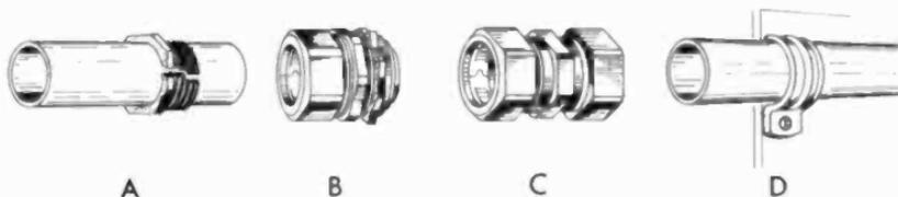
Fig. 2-14. Fittings for use with thin-wall conduit. *A* is a split nut that is placed on the end of the conduit. It is usually supplied with *B*. The thread is tapered. When *B* is threaded onto it and pulled up tight there is a tight friction fit. *C* is similar in use but is double-ended and splices two lengths of thin wall together. *D* is a bracket for holding thin-wall conduit to wood rafters and joists.
