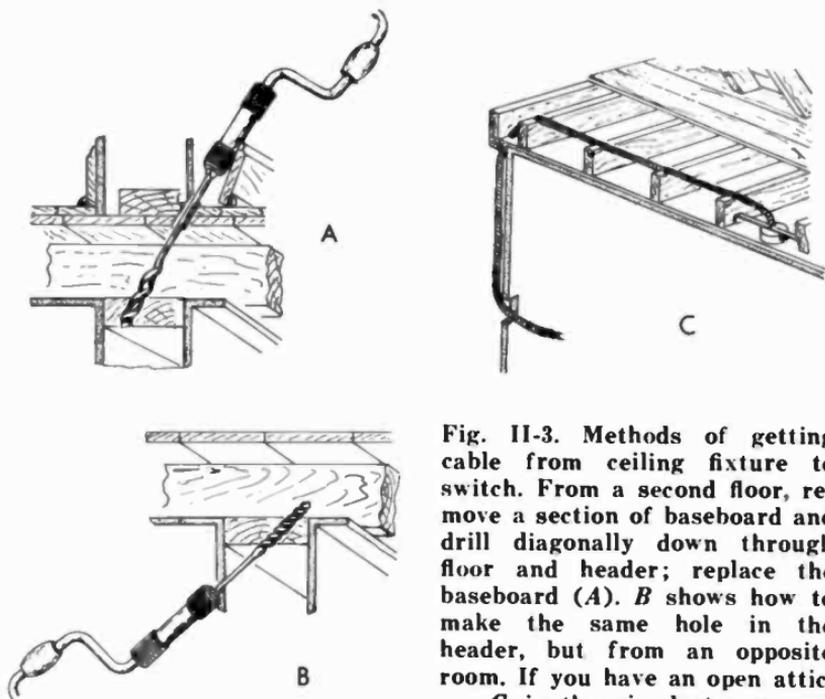
Fig. II-3. Methods of getting cable from ceiling fixture to switch. From a second floor, remove a section of baseboard and drill diagonally down through floor and header; replace the baseboard (A). B shows how to make the same hole in the header, but from an opposite room. If you have an open attic, C is the simplest way.
