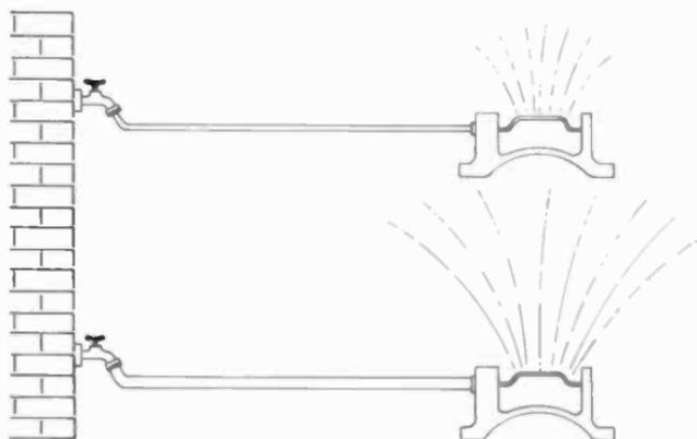
Fig. 1-1. A  $\frac{1}{2}$ -inch hose restricts the flow of water more than a  $\frac{3}{4}$ -inch hose.
