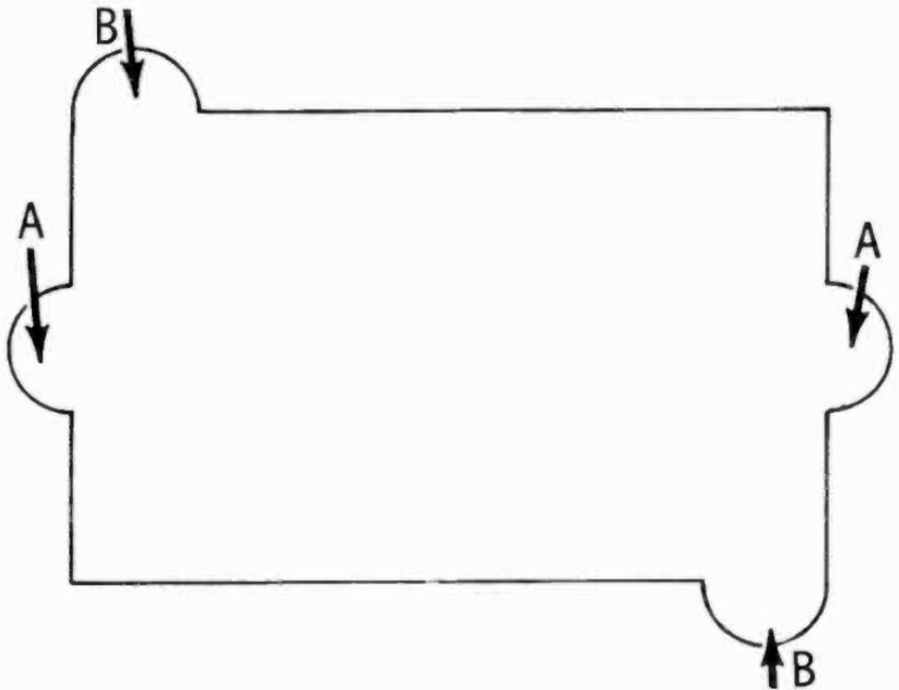
**Fig. 4-11.** This is an exact size pattern for use in cutting out a wall for a switch or outlet box. The ears at *A* and *B* are for holes to be drilled into the wall. *A* is for clearing a screw ear on the box. *B* is a starting hole for cutting the plaster.
