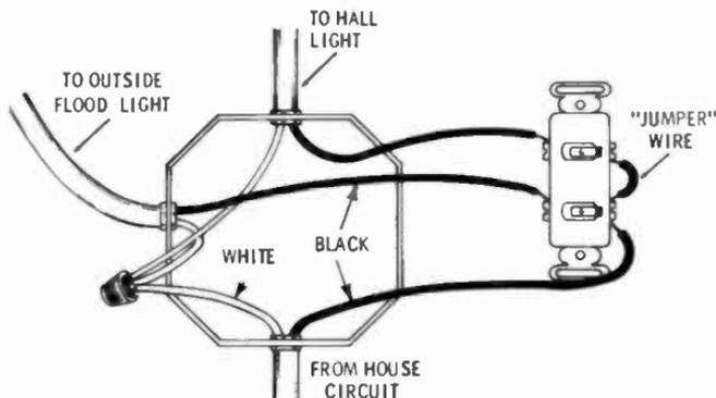
**Fig. IV-5.** Change a single switch to two switches: one for the original inside light, and the other for the new floodlight.
