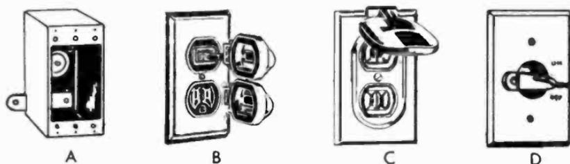
Fig. 2-6. Boxes and outlets of special construction to make them waterproof. *A* is a cast metal box with watertight bushings for use with thin-wall conduit. *B* and *C* are outlets and covers. *D* is a water proof switch.
