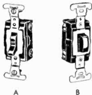
Fig. 2-7. *A* is the general appearance of the average standard snap-action toggle switch, as well as of the silent mechanical switch, silent mercury switch, and the delayed-action switch. *B* has a push bar on the front; push for "on"; push again for "off." Switches are installed with large ears at the top and bottom and flush against the front of the wall.
