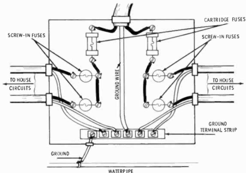
Fig. 1-6. A typical "60-ampere service" box, using fuses. The 240-volt service is brought in the top of the box by the power company. 60-ampere cartridge fuses protect the main incoming line. 15-ampere screw-in fuses protect the separate circuit branches against overload. Note that the "neutral" (colored white) lines are not fused.
