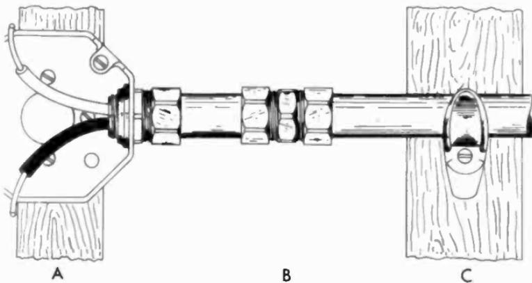
Fig. 4-5. Details of conduit installed in a junction box (A). Also shown is double-ended coupler (B) for splicing lengths of conduit, and bracket (C) for supporting long lengths.
