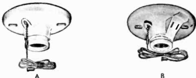
Fig. 2-11. Porcelain ceiling outlets with pull-chain switches. They are inexpensive and are frequently used in closets and areas where a fancy fixture is not needed. *A* is the standard type with Edison socket. *B* includes a convenience a-c outlet.
