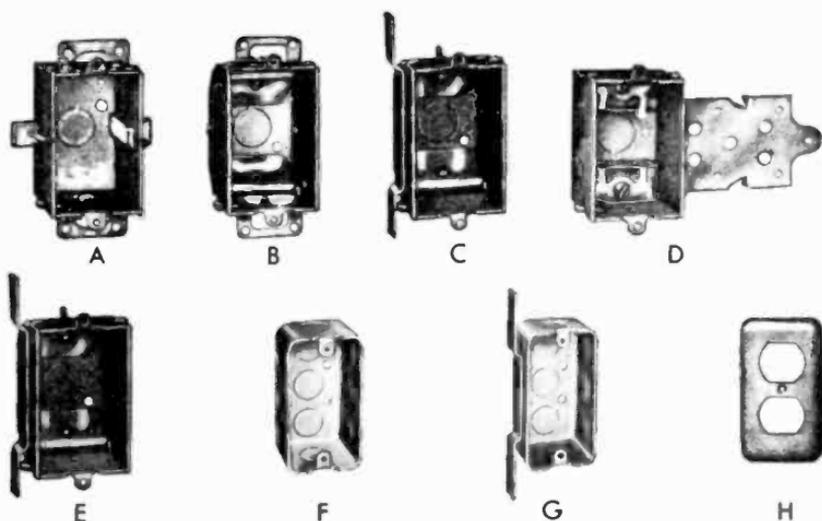
Fig. 2-4. Small boxes used to hold switches and outlets. *A* has pull-up side ears that hold the box to plasterboard and *Sheetrock*. *B* is fastened to the lathing in plaster walls with the top and bottom ears. Both of these boxes are for "old work." *C*, *D*, and *E* have brackets welded on for attaching to wall studs in "new work." *F* and *G* are for exposed mounting, such as at work benches; *H* is a metal cover for these types, providing accommodation for a duplex outlet.
