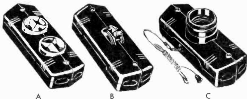
Fig. 2-13. Devices used for surface wiring where exposed wiring is not objectionable. They interconnect with plastic covered cable tacked in place. *A* is a duplex outlet. *B* is a toggle switch, used with *C*, a light bulb outlet.
