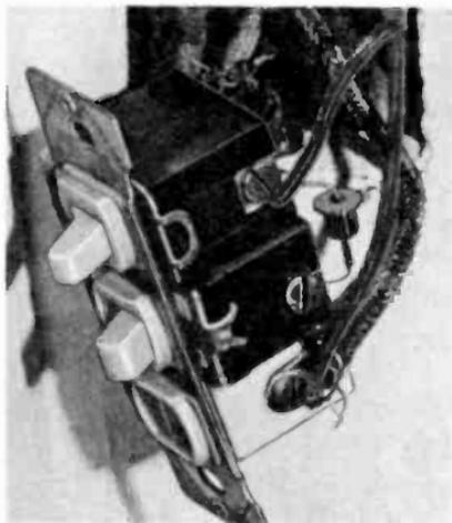
Fig. II-5. Photo shows the "top hat" silicon rectifier used to dim the fixture lights.
