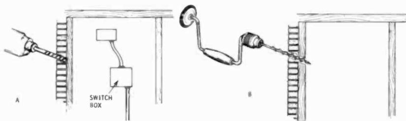
Fig. IV-3. If you must go through brick for bringing in the thin-wall conduit, use a carbide-tipped drill bit and electric drill to start (A). Use a  $\frac{5}{8}$ -inch electrician's wood bit and hand brace for wood(B).
