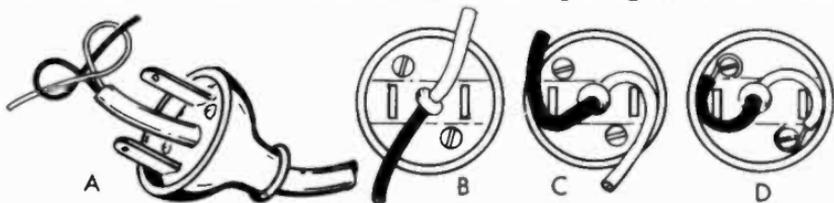
Fig. 3-2. Replacing a plug on an electric cord. Push the cord through the back of the plug. Tie an Underwriters' knot.
