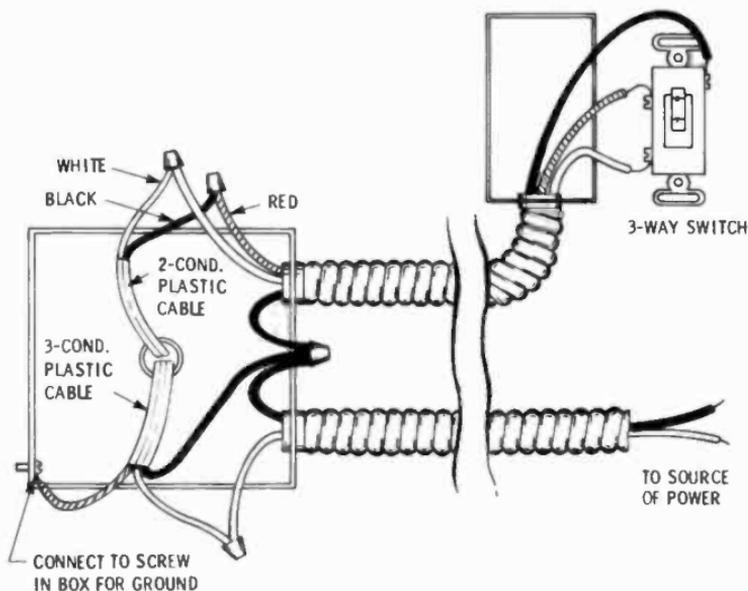
**Fig. V-3. In-house wiring to underground cable to provide switching of lights from house to garage, plus separate power for outlets in garage.**
