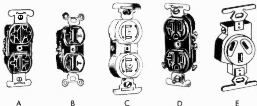
Fig. 2-10. Here are some of the various types of outlets. Most are double (duplex), since two fit the same box. *A* is the most commonly used duplex outlet. *B* is slotted to take some of the older plugs. *C* has spring-loaded rotatable covers to keep children from poking metal objects into the terminals. *D* is for use with the three-prong safety plug, but also takes the standard two-prong plug. *E* is called a "crowfoot" outlet, for 240-volt wall outlets.
