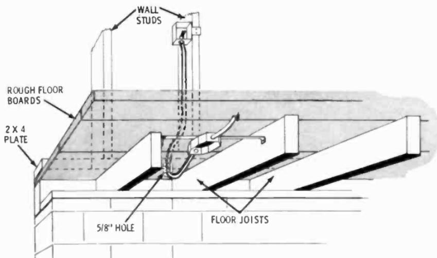
**Fig. 4-15.** To feed cable to a new outlet from the basement, drill a  $\frac{5}{8}$ -inch hole through the "plate"; this is the  $2 \times 4$  put down on the ends of the floor joists when the house was built, and on which the wall studs were nailed.
