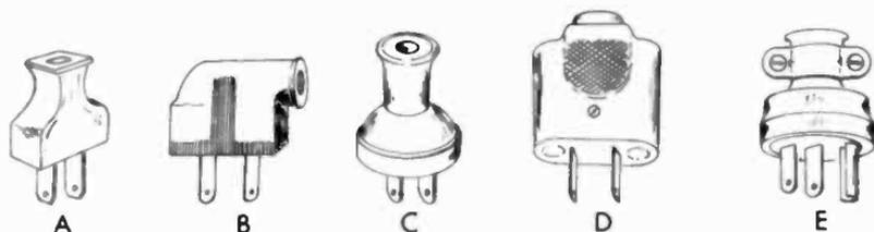
Fig. 3-1. A few representative plugs used as replacements on line cords.
