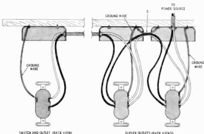
**Fig. I-2. Wiring of workbench front outlets. Note ground wire at X. This is the most important one since there is no other bond between the right-hand box and the rest of the front outlets.**
