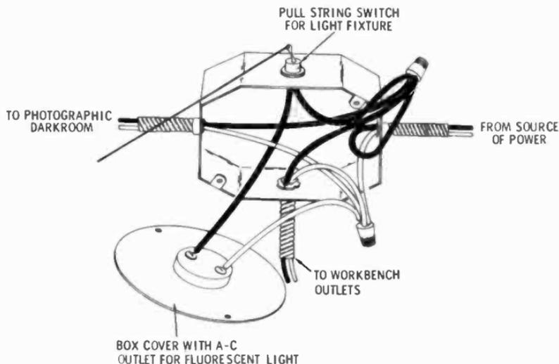
**Fig. I-4. Wiring of junction box above workbench. This illustration shows couplers on the flexible armored cable. The switch is installed by drilling a hole of the proper size in one of the knockout forms.**
