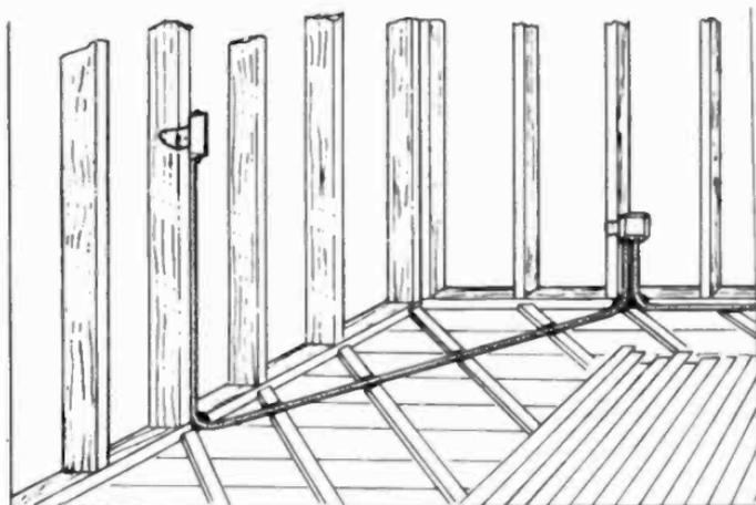
**Fig. 4-2.** Easiest way to put in conduits in "new work" is to lay them across the rough flooring. Note notches in "plate." This is better than notching the wall studs to run conduit across the wall. Boxes and conduit are installed while room is still in the rough. Wire is drawn through the conduit, and fixtures are installed only when the room is completely finished.
