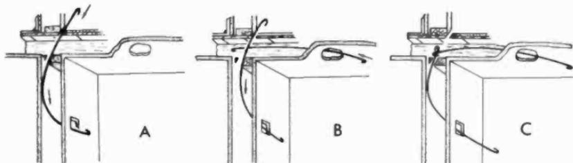
Fig. II-4. "Snake" a short fish line down through the floor board hole and header hole from the second floor, and bring the end out at the 4" x 5" plaster cutout, as shown at A. Push a longer fish line through the ceiling hole and hook the first one, as in B. Draw the short fish line down, and pull the long one through, into the room (C).
