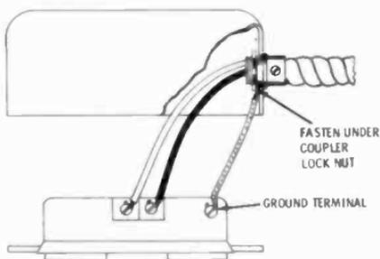
**Fig. 3-6.** On safety duplex outlets, the ground terminal is connected internally to the mounting ears. For added safety, connect a wire from the external ground terminal to a tight screw or nut on the outlet box.
