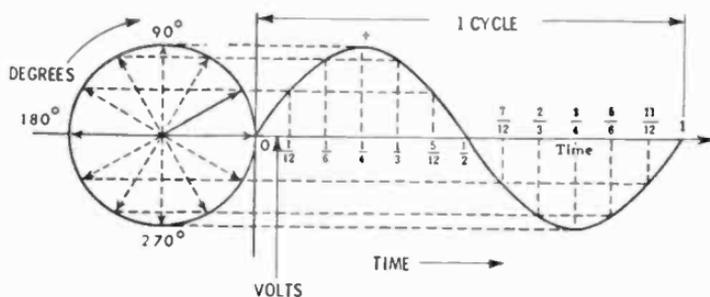
Fig. 1-4. Alternating current changes shown graphically. The curve is plotted against degrees of rotation (of a generator, for example) versus time. The speed of the generator produces 60 cycles per second. The curve is called a "sine wave."
