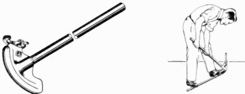
Fig. 4-3. Special bending tool is best for bending thin-wall conduit. It assures bends of proper radius, without kinks. Tool comes without handle. Handle can be a piece of rigid gas pipe.
