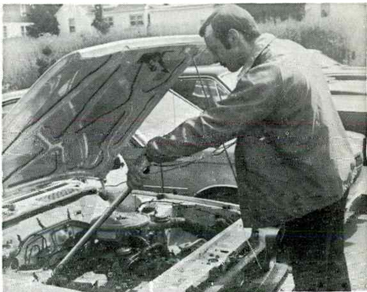
Fig. 26-4. Using the noise locating Sleuth (courtesy of Delco Electronics).
