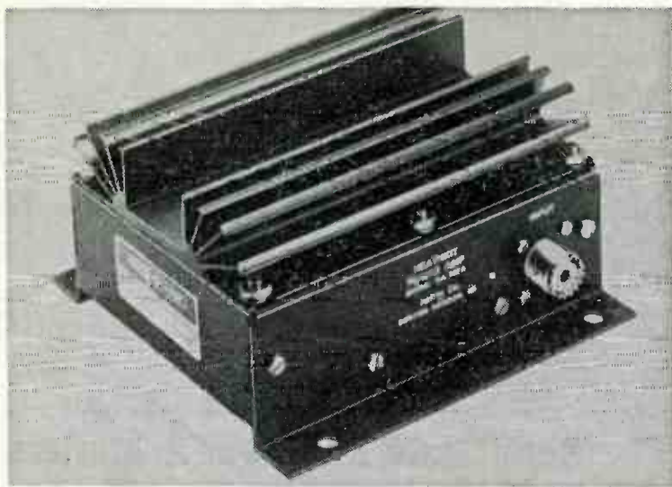
Fig. 8-1. Typical VHF power amplifier.
