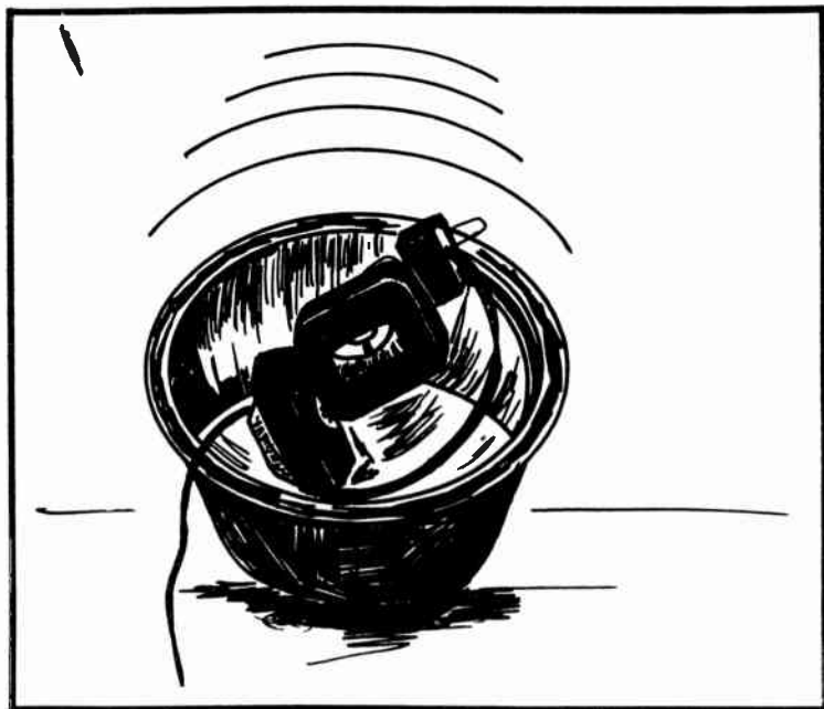
Fig. 4-1. Before loudspeakers were invented, a way of enabling more people to hear headphones was to put them in a pudding basin.
