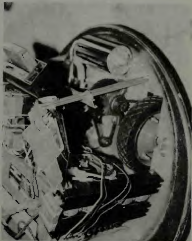
Fig. 3-10. Installation of the tape player at an angle. Heavy duty battery in upper left, some mounting brackets for electronics boards, details of the left drive wheel show bolts used to fasten gear to the wheel.
