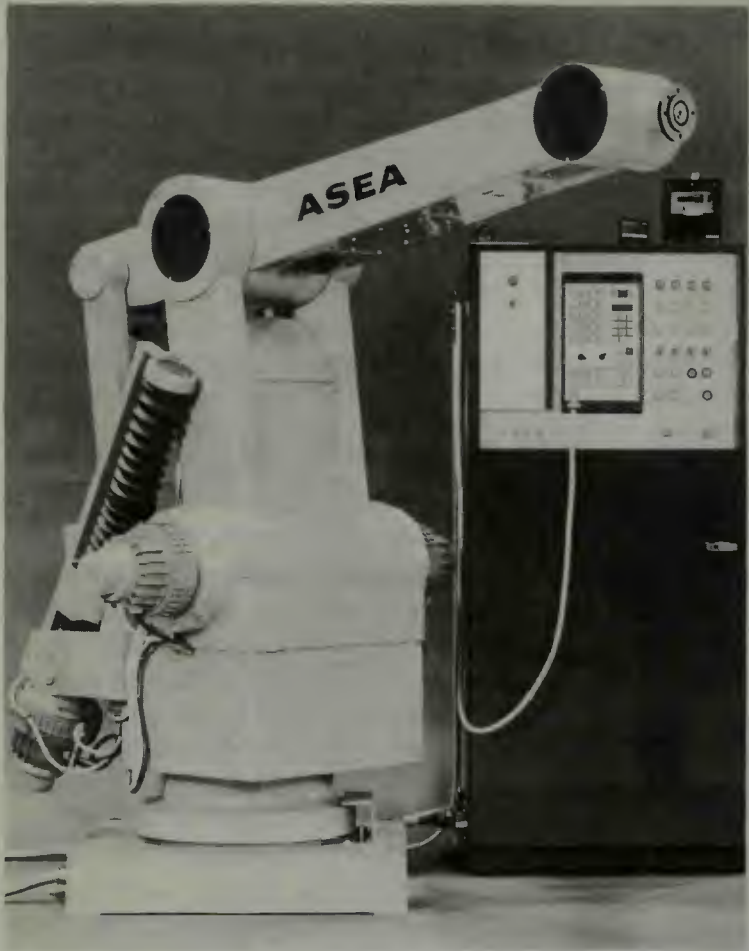
Fig. 8-1. The ASEA robot for industrial applications (courtesy ASEA).
