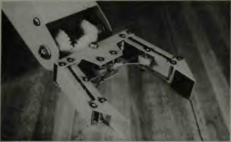
Fig. 7-5. The Mini-Mover 5 hand (courtesy of Microbot).
