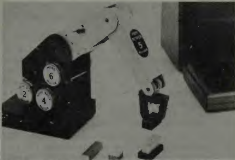
Fig. 7-2. A close view of the Mini-Mover 5, as the arm is called, and three of the six motors used in its operation. Motors 1, 3, and 5 are on the opposite side of the arm in this view (courtesy Microbot).
