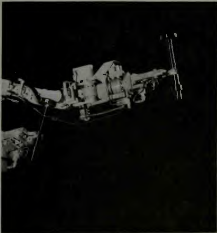
Fig. 4-4. The wrist and gripper of the Cincinnati Milacron T 3 robot (courtesy Cincinnati Milacron).
