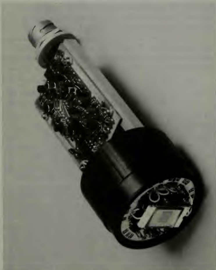
Fig. 9-13. The General Electric Robotic-Eye. Notice the matrix at the end of the tube. It is very small but has a very large number of "cells" (courtesy G.E.).
