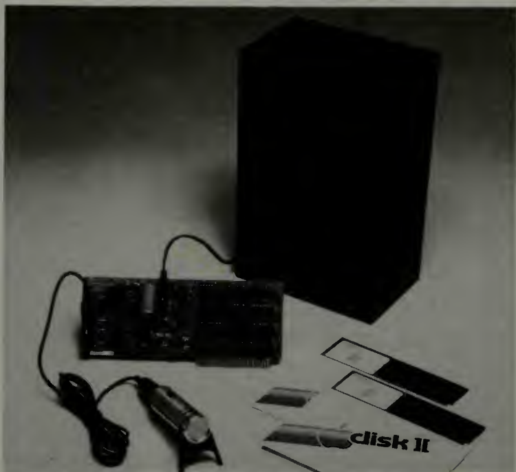
Fig. 13-2. The Mountain Hardware Supertalker system for the Apple computer (courtesy Mountain Hardware).
