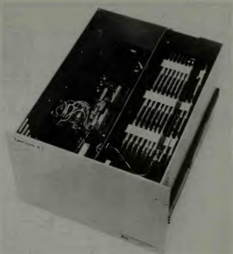
Fig. 10-7. The Eyecom electronics package with removable circuit cards (courtesy Spatial Data Systems).
