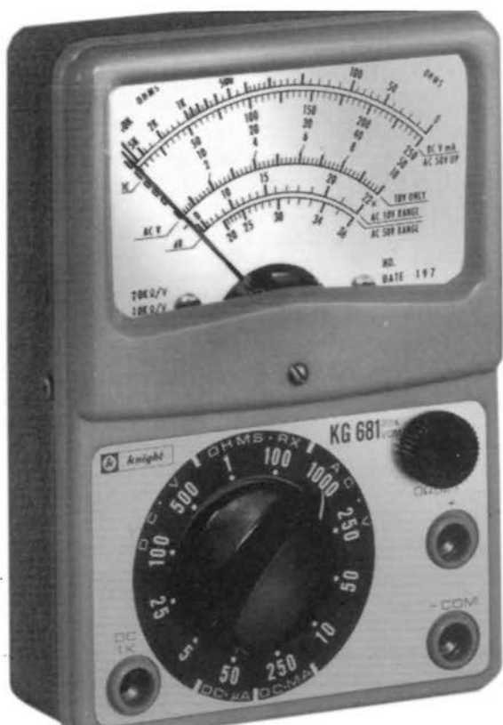
Fig. 1-5. A typical, simple volt-ohmmeter, such as this one, costs from $8 to $10.
