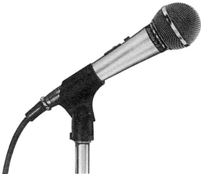
Fig. 5-7. The pickup characteristic of a microphone are not apparent from the appearance. This microphone, a Shure 558SA, actually has a sharp directional pattern.
