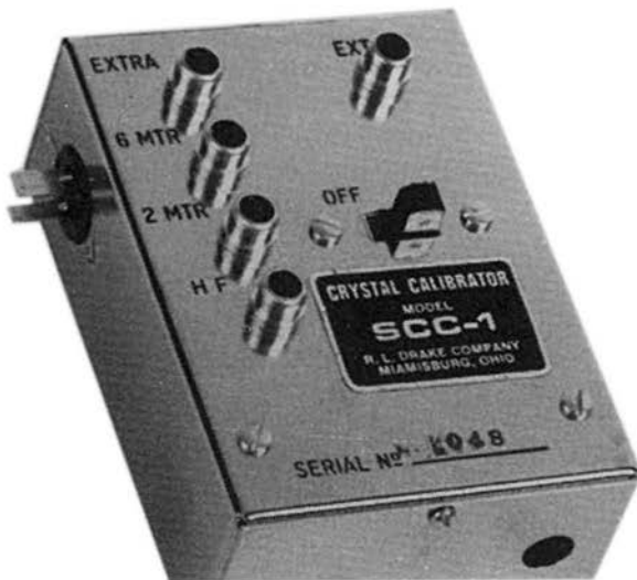
Fig. 4-8. This wide-range calibrator provides markers at 50-kHz intervals up to and including the high VHF band. (Courtesy R. L. Drake Co.)
