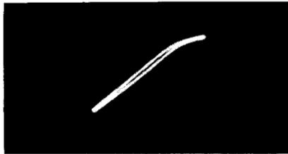
Fig. 708 (left). *Insufficient bias rounds the tops of the waveform.* Fig. 709 (right). *Characteristic corresponding to the condition shown in Fig. 708.*
