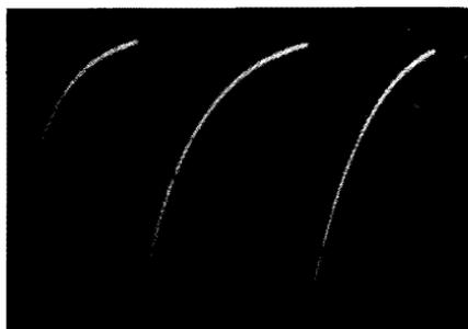
The voltage built up across a charging capacitor, however, is not proportional to time because of the exponential nature of the charging characteristic (Fig. 221). The charging current becomes lower and lower as the voltage across  $C$  approaches the voltage  $E$  of
