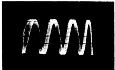
Fig. 1023 (left). *Hum in the X amplifier. The whole trace is shifted back and forth.* Fig. 1024 (right). *Time-base hum. While one end of the trace remains stationary, the other end is swept back and forth.*
