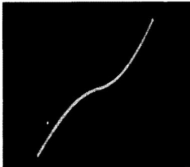
Fig. 642. *Characteristic of a non-linear thyrite resistor (varistor).*
