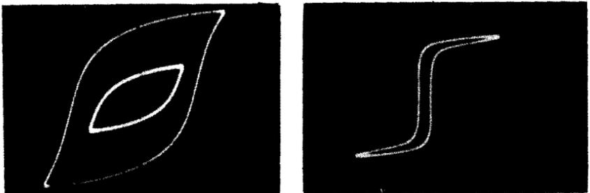
depending upon the direction (increasing or decreasing) of the variation of  $H$ . That explains the loop-shaped aspect of the  $B/H$  characteristic.
