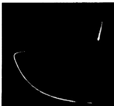
Fig. 763.  $P1/G1$  characteristic of the multivibrator.
