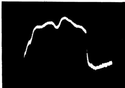
grid (or even into the cathode) of the C-R tube by pickup or by poor filtering of the power supply. This produces an intensity modulation of the trace as shown in Fig. 1008 (a 120-cycle wave is displayed). For a sine wave of higher frequency and the same time-base setting (15 cycles), an intensity-modulated rectangle (Fig. 1009) is obtained.
