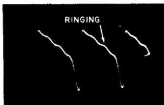
of the waveform will become attenuated in the vertical amplifier of the scope.
