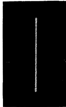
Fig. 404. Calibrating the C-R tube by using a variable ac voltage to produce a 3-inch deflection. The time base is turned off.
