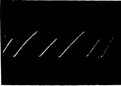
Fig. 236. Sawtooth voltage producing sweeps of different lengths.
