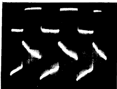
Fig. 766. Waveforms at P1 (above) and G2 (below) of the cathode-coupled multivibrator.
