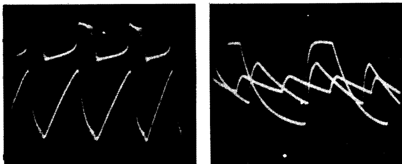
Fig. 246 (left). Above: grid voltage of blocking oscillator; below: sweep voltage across C1 . Fig. 247 (right). Decreasing amplitude and increasing frequency result from increasing R1 .
