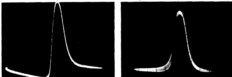
Fig. 851 (left). Base-line distortion resulting from connecting scope input to point C of Fig. 829. Fig. 852 (right). Superimposed rf component appears when the scope is connected to point B.
