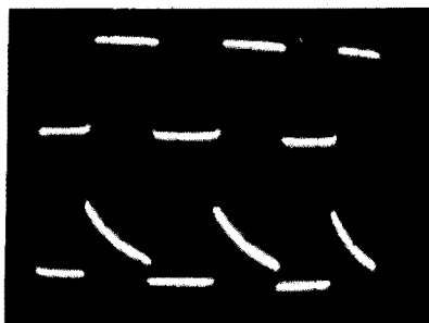
Fig. 767. Waveforms at P1 (above) and K (below) of the multivibrator circuit of Fig. 764.
