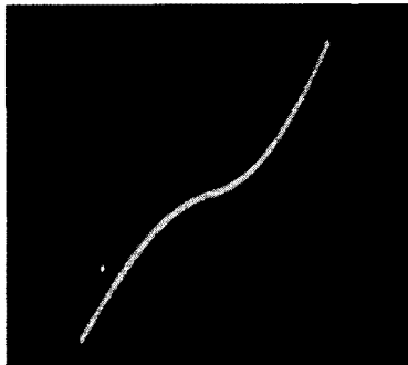
Fig. 642. Characteristic of a non-linear thyrite resistor (varistor).
