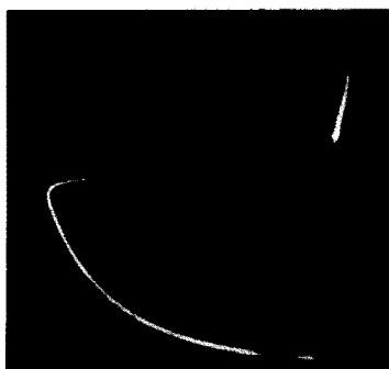
Fig. 763. P1/G1 characteristic of the multivibrator.
