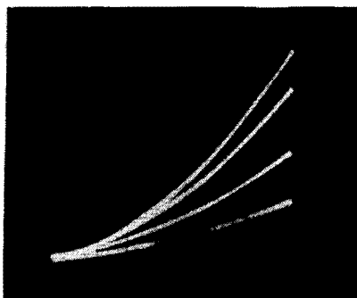
Fig. 613 (left). Effects of various load resistances on 12AX7 characteristics. The top curve is for a zero load. Fig. 614 (right). I_p/E_g curves for different bias voltages.
