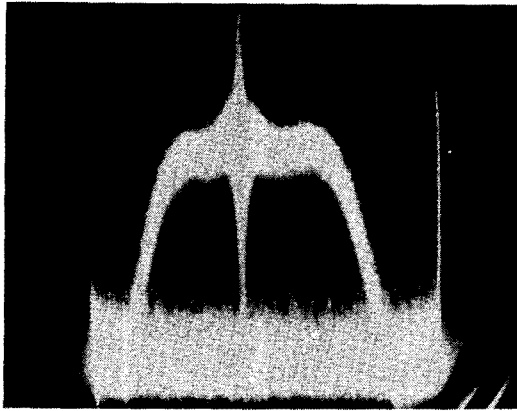
Fig. 910. To avoid noise modulation of video curve an if amplifier tube should be pulled. Use a dummy tube (all leads clipped, except filament) in series-string receivers.
