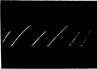
Fig. 236. Sawtooth voltage producing sweeps of different lengths.
