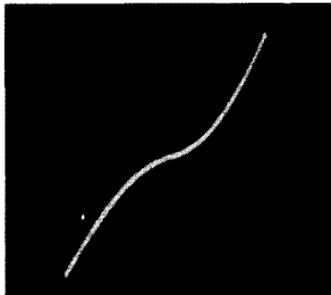
Fig. 642. Characteristic of a non-linear thyrite resistor (varistor).
