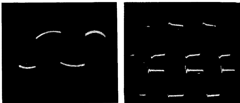
Fig. 808 (left). Rounded tops indicate low-frequency boost. The test frequency was 180-cycles. Fig. 809 (right). Overshoot (upper trace) caused by shunting the transformer primary with a capacitor; ringing (lower trace) produced by shorting the feedback resistor.
