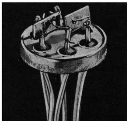
Fig. 714. Interior view of a multi-headed transistor. (Electronic Transistors Corp.)
