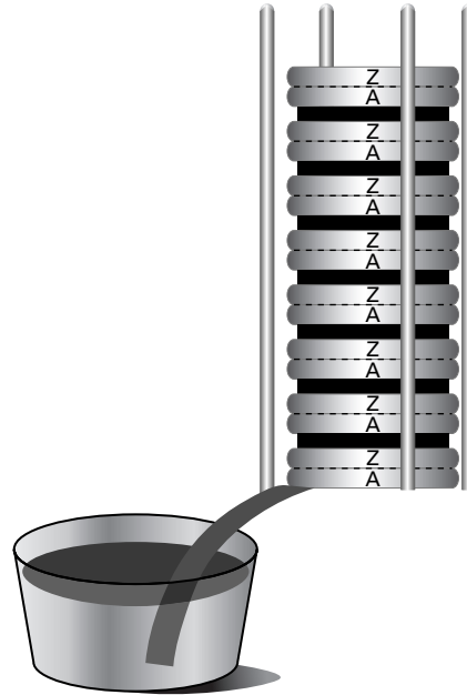
FIGURE 3-1 An illustration of the silver-zinc battery devised by Italian scientist Alessandro Volta. “A” stands for silver and “Z” for zinc.
