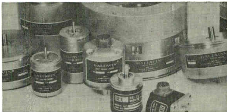
Fig. 9-4. Shaft position encoders convert a shaft position into a digital signal (courtesy of BEI Electronics Inc.)
