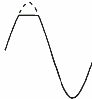
Fig. 5-14 This sine wave is severely clipped on its positive peaks.
