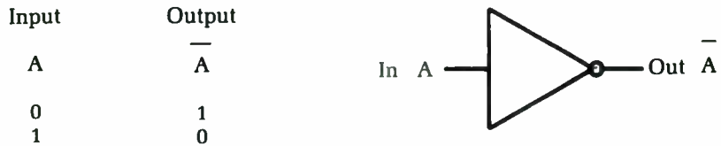
Fig. 10-2 An inverter reverses the input state at the output.
