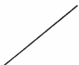
Fig. 5-24 Applying the same sine wave to both inputs produces a Lissajous figure that looks like a simple slanted line.
