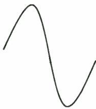
Fig. 1-9 An audio oscillator generates an audio frequency sine wave.
