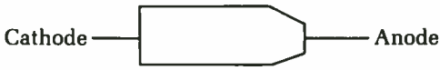
Fig. 6-14 On some diodes, the body is tapered on one end to indicate the location of the anode.
