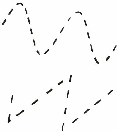
Fig. 1-7 In the chopped mode, the oscilloscope switches between the two signals many times per sweep cycle.
