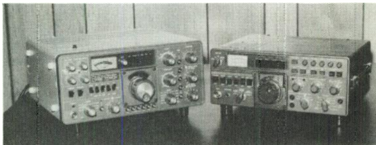
Fig. 3-6. The Kenwood TS1805 and YAESU FT901DM are two state-of-the-art transceivers featuring every modern convenience from frequency memory and bandpass tuning to internal speech compressors, variable IF-bandwidth and effective noise blankers. Both rigs also feature effective air circulation and blowers.
