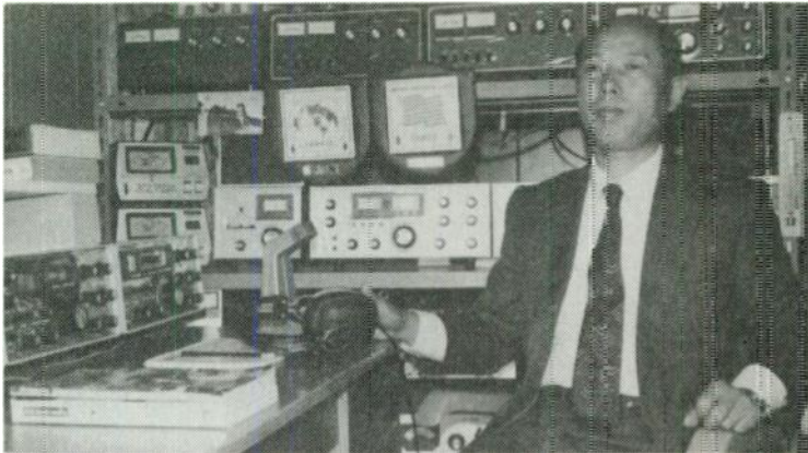
Fig. 3-2. Inside view of the station belonging to Hisanobu Mori, JA9BE. His equipment includes separate FTDX401 transceivers and FL2100B linear amplifiers for 20, 15 and 10 Meters, plus an additional complete station consisting of a FL101 transmitter, FR101 receiver and FT101E transceiver. An all-band receiver is also visible below the tabletop. Note his recently-acquired 5 Band DXCC and 5 Band WAS awards on wall.
