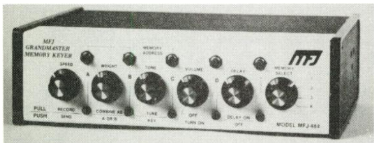
Fig. 6-6. The MFJ Grandmaster Memory Keyer can retain four discrete messages, which can be recalled as desired, or the memories can be combined for transmitting longer messages. The memories can be instantly reprogrammed and the unit is also a high-quality iambic keyer.
