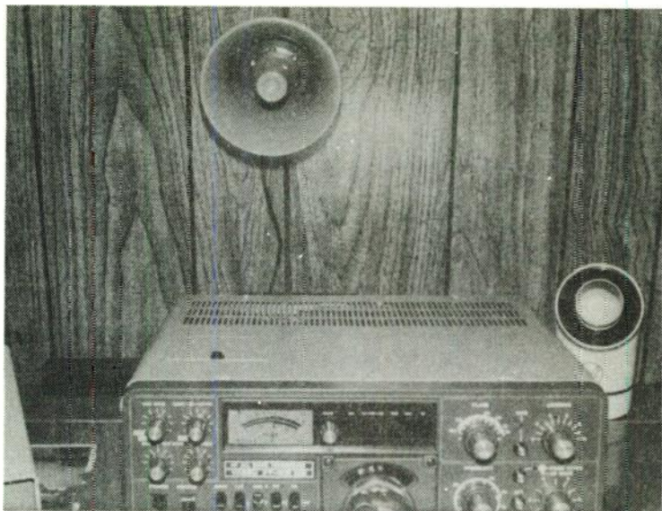
Fig. 6-1. A paging trumpet functioning as a "selectively-tuned" speaker for SSB operations. The frequency response of these units, coupled with their high power handling ability, makes them a staunch performer for many DXers.
