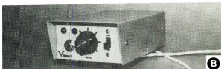
Fig. 6-8. Speech compressors have for several years been considered the DXers special "trump card" for contest and pileup operating. When properly adjusted, a speech compressor can add up to 8 dB of talk-power to SSB transmissions.
