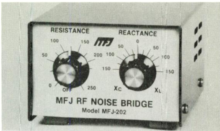
Fig. 6-7. The MF RF Noise Bridge can be used for checking numerous antenna parameters, tuning matching networks, setting plate coil taps and much more. DXers interested in getting top performance from their rigs will surely find this item a station necessity rather than an accessory.
