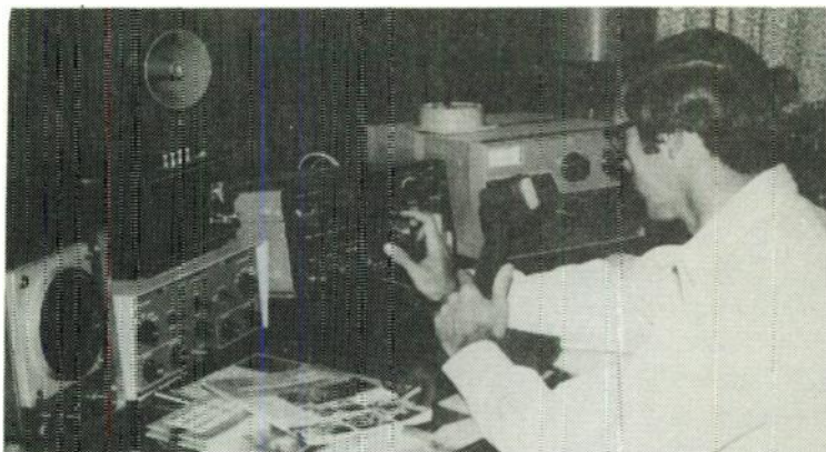
Fig. 1-3. The amateur setup of the author, K4TWJ, blends several aspects of DXing without unnecessary rearrangement. Mode capabilities include SSB, CW, SSTV, OSCAR satellites, 10 meter FM, UHF, RTTY and 160 meters—the equipment is a combination of commercial, modified and home-constructed units. Additional station gear (not visible) is behind the operator's chair and a book-shelf outside the room holds DX magazines, log sheets and operating references.
