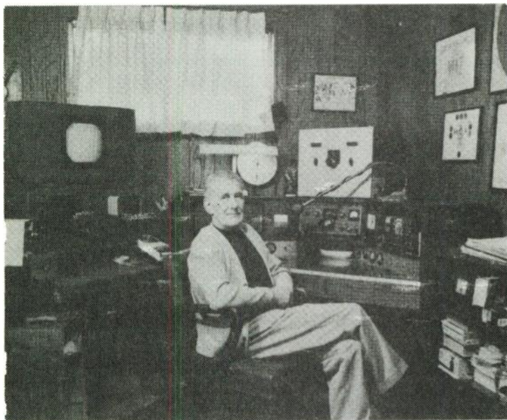
Fig. 1-7. A serious DXer, Glen Tillack, W6KZL; has been at the top of the DXCC Honor Roll for several years. Glen uses two transceivers: one continuously tuned to 20 meters and one for use on the other bands. His amplifier is homebrew—4-1000 final with remote power supply. Homebrew SSTV gear sits on the left of station console. Glen has always been handicapped by an antenna zoning restriction, so antenna is a three-element beam (26 foot boom) atop a mere 45 foot tower. Obviously DXing isn't what you have, but how you use it.
