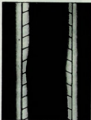
Fig. 17 — Different patterns are used to illustrate the portions of a 78rpm record groove seen by the three photocells. A slightly different view of the record groove is transmitted to each of the three photocells.
