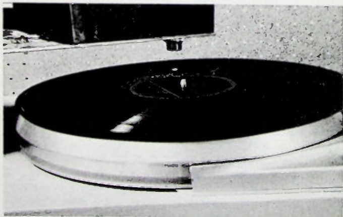
Fig. 20 — One experimental model of a needleless phonograph with all the optics enclosed at the end of the tone arm.
