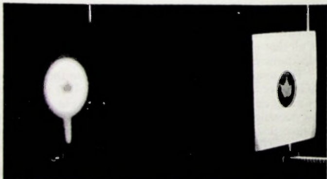
Fig. 2 — A distant light can be used to cast the shadow of the leaf on a screen without using a lens.
