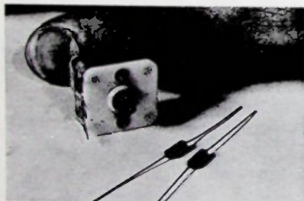
Fig. 6 — Tuning diodes are compared to a miniature mechanical tuning capacitor they can replace.
