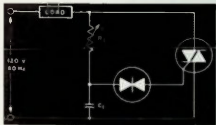
Fig. 11 — A solid-state circuit for controlling the ac current applied to a load.
