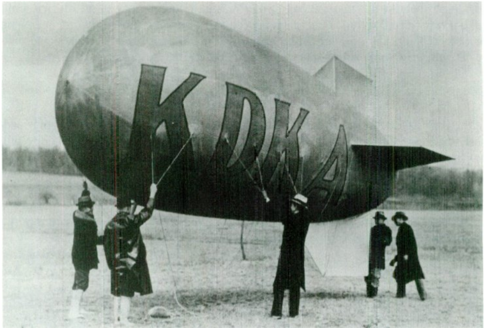
AN EXPERIMENTAL ANTENNA carried aboard a dirigible is tested in the Pittsburgh area by KDKA Radio personnel. Photo taken in the early 1920's.
