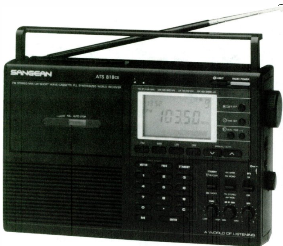
5-3 The Sangean ATS 818CS allows you to record and play cassette tapes.
