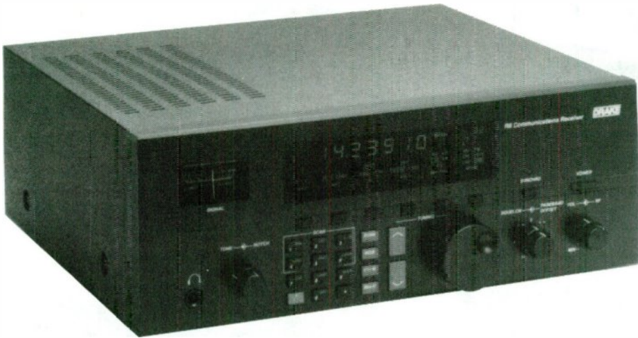
5-4 The Drake RF8, a top-of-the-line communications receiver.
