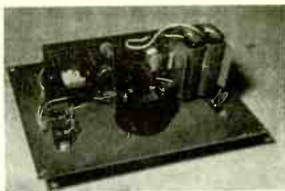
Interior of the transconductance tester. The 1000 Hz oscillator is mounted in the upper left hand corner of the Vero board. The batteries are installed in a metal clip on the far right.
