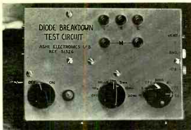
Fig. 5. Top view. I finished the Tester with slow-drying enamel and freshhand India ink lettering.
