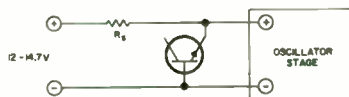
Fig. 2. Using a transistor as a zener diode to stabilize a transistor oscillator stage. Selection of R_s is discussed in the text.
