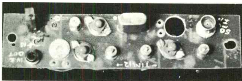
Top view of W6AJF's six meter FET converter. The extra hole by the BNC input jack was used for neutralizing trimmer that proved unnecessary.
