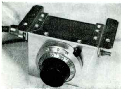
Front view of the six or two meter VFO using a piston tuning capacitor as shown in Fig. 3.
