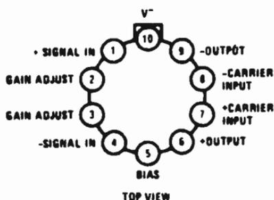
Note: Pin 10 is connected electrically to the case through the device substrate.
