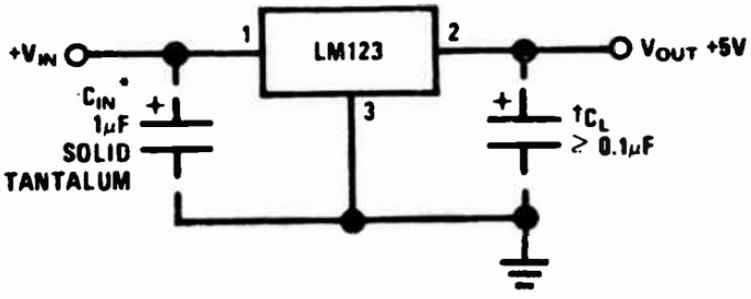
\*Required if LM123 is more than 4" from filter capacitor.
