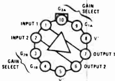
Note: Pin 5 connected to case.
