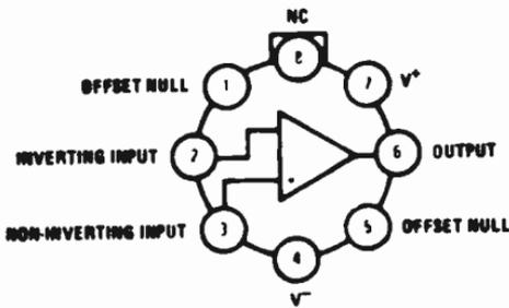
Note: Pin 4 connected to case.
