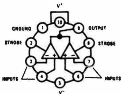
Note: Pin 5 connected to case.
