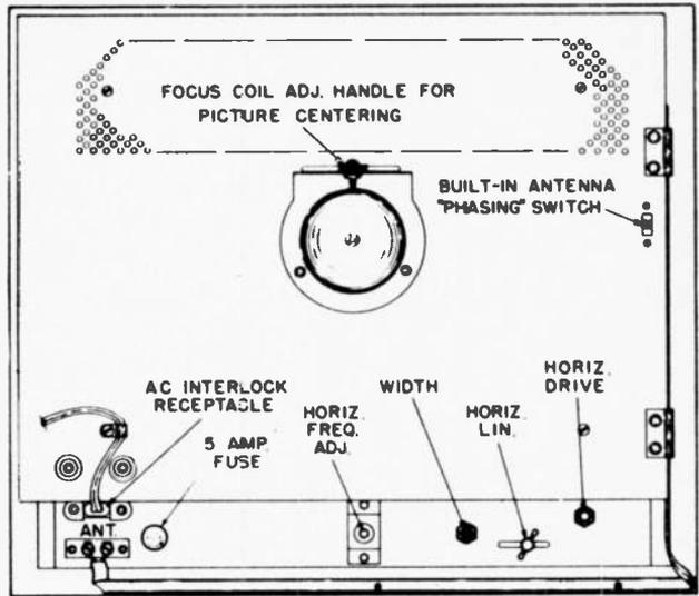
screwed onto the back of the cabinet, partly to protect people from the set, and partly to protect the set from people (children, and the "fools rush in" type). Usually, removing the back cover disconnects the electric power from the set, as will be explained later.
