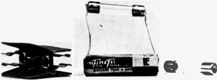
Fig. 59—In the center is a pig-tail fuse, which needs to be soldered in place. At right is a cartridge fuse. At left is an adapter which can be used to convert from pig-tail to cartridge type fuse, to avoid soldering in a replacement. One side of the adapter snaps onto the existing pig-tail fuse in the set, and a new cartridge fuse is snapped into the other side.
