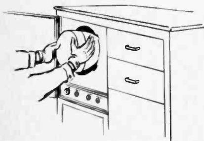
Fig. 29—Removing the picture tube.
