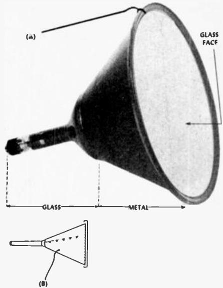
Fig. 28—Metal cone picture tube/High voltage may be connected to the lip (A) or to a snap fastener on the plastic sleeve which covers the metal (B).
