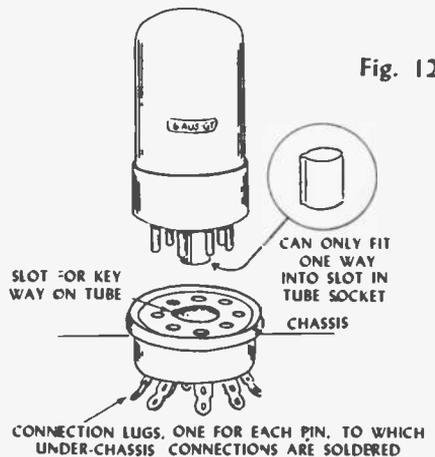
are places to connect wires and other parts which connect the tube into a "circuit."
