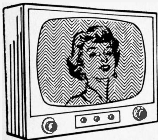
lines, a herringbone pattern, a moire pattern, etc. The "venetian blind" effect, described in the previous chapter, can be considered a form of interference. Auto ignition and electric motor interference appear like little black dashes or hyphens at random throughout the picture. Snow is NOT interference, as has been explained.
