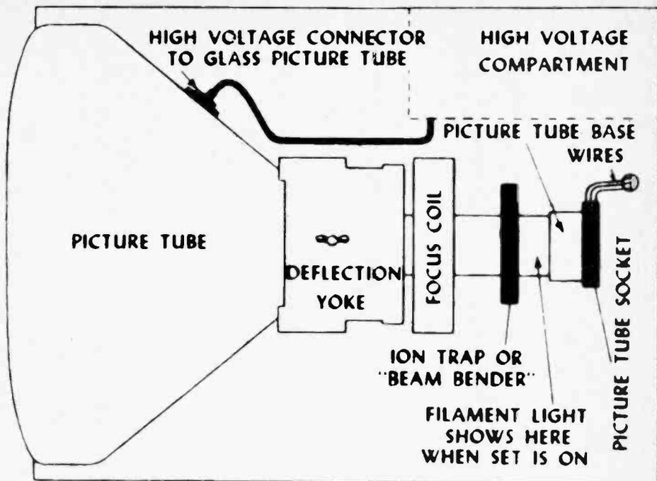
Fig. 30—Typical view from top of chassis, showing placement of yoke, focus coil, ion trap and high voltage connection. In removing picture tube, the high voltage connector and the tube
