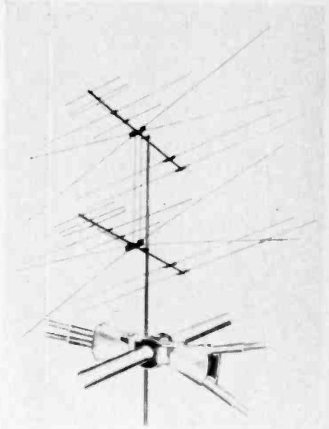
Fig. 42 (left)—Almost any type of antenna can be stacked. "C" at left is a 4-stacker, while "D" and the Channel Master Conical-Yagi in Fig. 43 (above) are 2 stackers.
