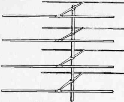
(C) 4-STACK DIPOLES AND REFLECTORS
