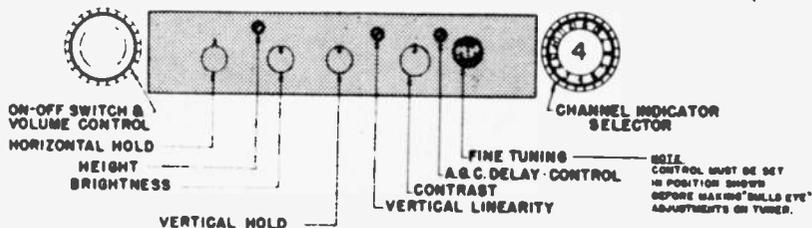
Fig. 5—Simplified front operating controls (Zenith M2237R). Adjustments in the shaded area are concealed behind a drop panel instead of being on the
