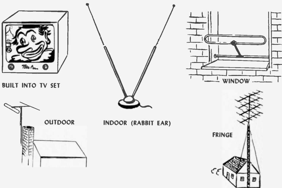
Fig. 38—The strength of the signal in your locality will determine which of these five antenna types will work for you.
