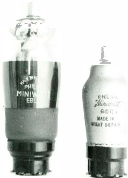
Examples of Continental side-contact bases, known by Philips as Cap P. c. 1938.
