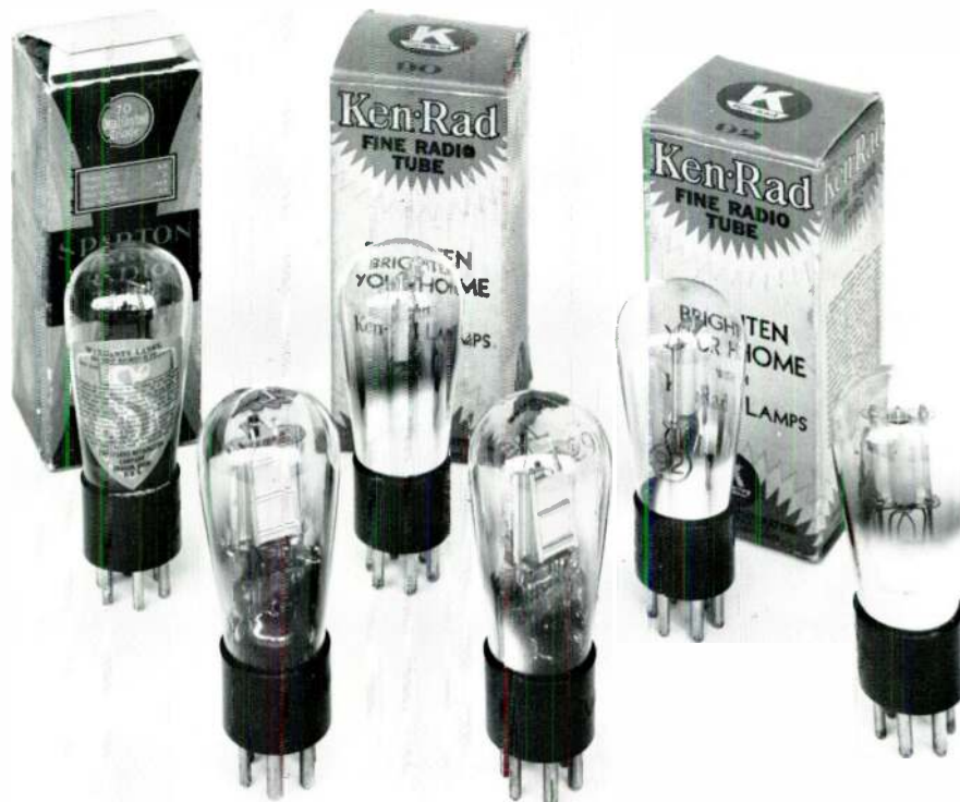
A group of dual-grid detector tubes (1932).
