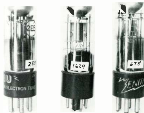
American 'Magic Eyes.' Note octal base on centre tube.
