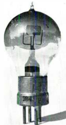
Example of the original French 4-pin metal base.
