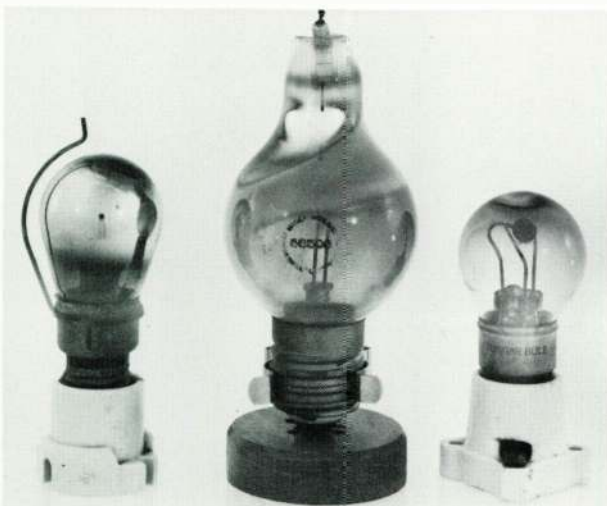
Two versions of the 2-amp Tungar bulb (outer) and a 6-amp (centre).
