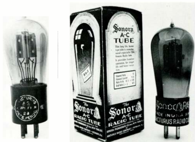
Arcturus AC28 and Sonora RA-1. These tubes had 15-volt carbon-heaters.
