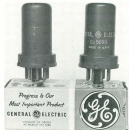
Two post-war GE metal tubes in the Red 'computer' range c. 1950.
