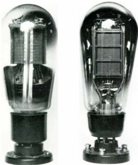
Philips F443 Osram PT25 Giant European pentodes of 25 watts anode dissip. There were no American equivalents.
