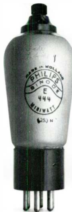
Philips E444 'Binode' fitted with American 6-pin base.
