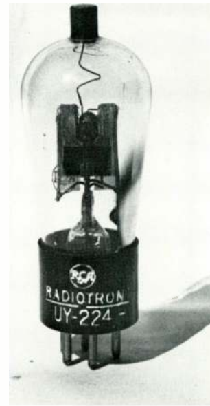
Early production model UY-224. Note fork-shaped screen assembly.
