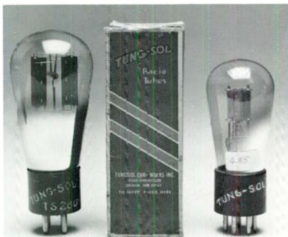
Tung-Sol TS280 (L.) and 485 (R.). The latter is a Sparton replacement.
