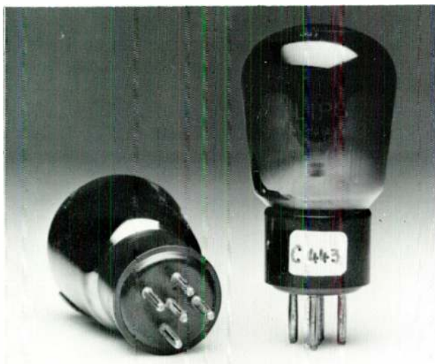
The standardised European 5-pin base introduced in 1929.
