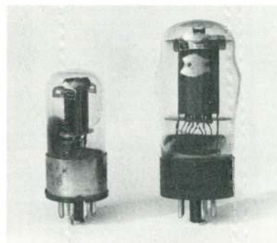
6H8C 6P3C Two Russian octal-based tubes (1954).
