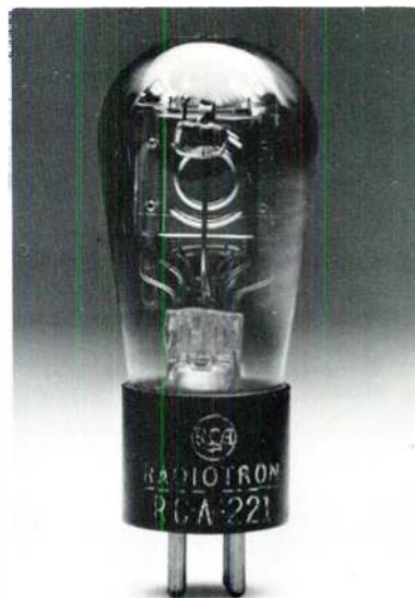
RCA-221. The 'export only' tube. Filament rating was 5V, 0.06A.
