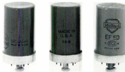
War-time versions of the EF50/VR91 metal-glass RF pentode.
