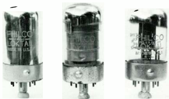
Tubes using Loktal bases (Circa 1940)
