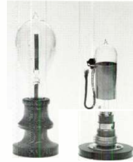
Replica of an Edison 110-volt carbon-filament lamp compared with a commercial version of a Fleming diode.
