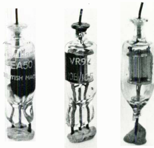
Mullard EA50. A detector diode originally released by Philips in 1939.
