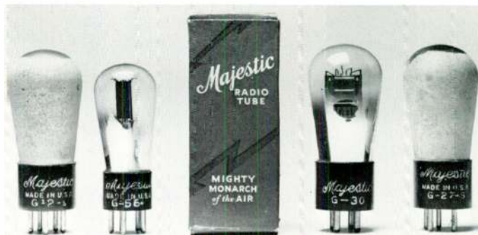
Typical Majestic tubes. Note the use of a large-size (S-14) bulb on the type G-30.
