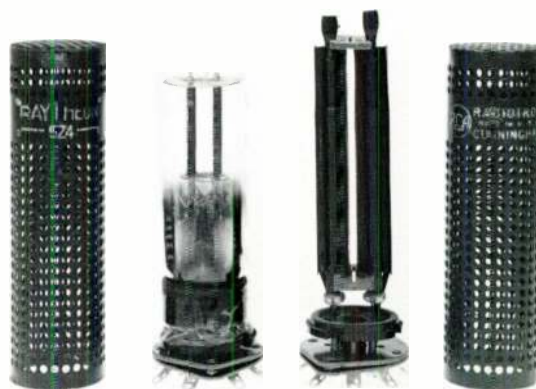
Two completely different versions of the 5Z4 rectifier. Both were original releases in 1935.
