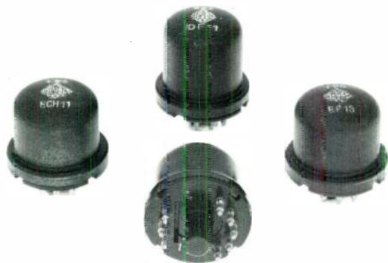
Telefunken metal tubes c. 1939.
