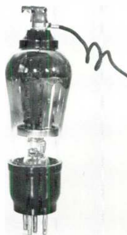
Osram VMS4 valve using hybrid top connector (1933).
