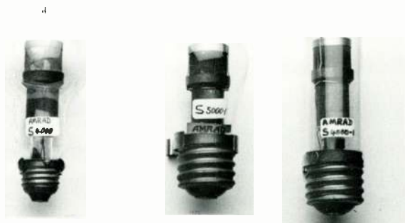
Amrad—the first gaseous rectifiers c. 1922.
