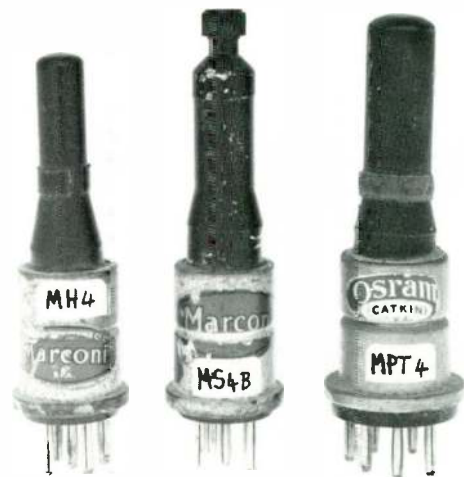
Marconi-Osram 'catkin' valves produced without screening cans.
