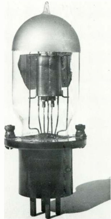
Farad—an early AC tube. Note twin heater-cathodes.
