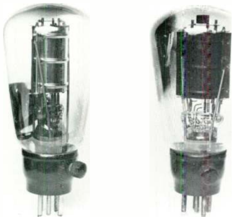
Example of a British 5-pin valve having a side terminal for the sixth connection (1930).
