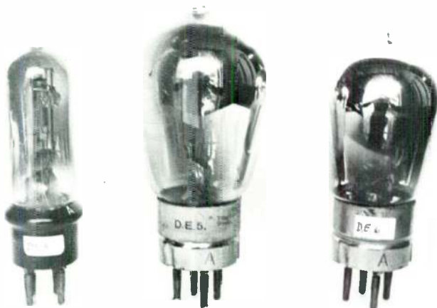
Marconi DE3, DE5, DE6 early dull emitter types.
