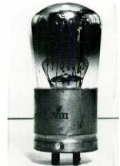
Example of a European tube using an American-style UV base c. 1924.
