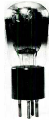
Example of tube using a Franco-British 4-pin bakelite base c. 1926.
