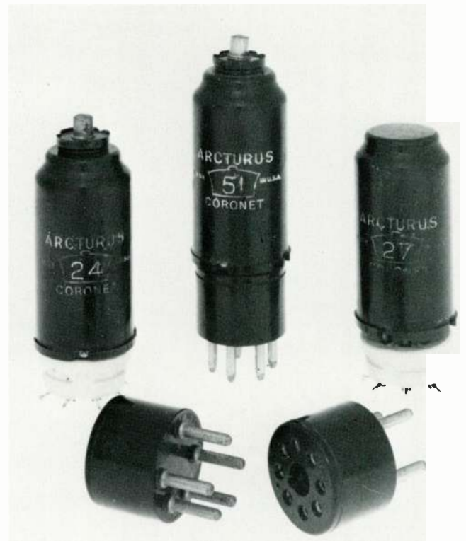
2.5-volt Arcturus 'Coronet' tubes with socket adaptors.
