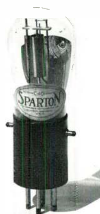
Sparton C401. Heater connections are to the side pins.
