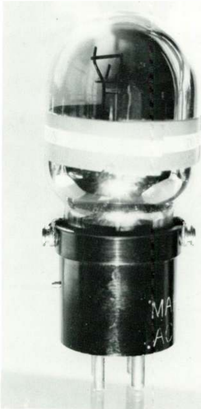
Marathon AC608R. Note heater connections on sides of base.
