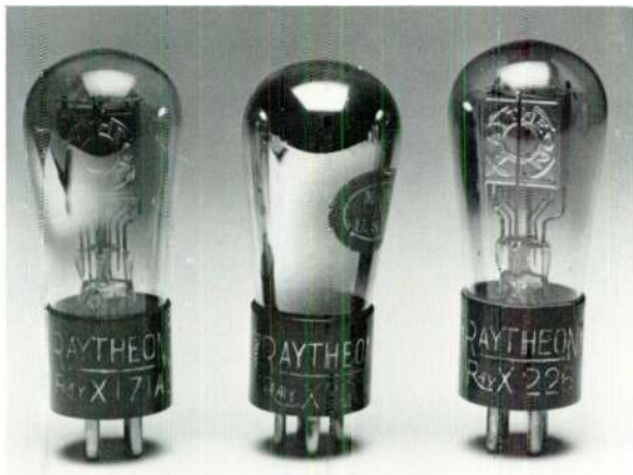
Raytheon Ray-X171A, 201A, 226. The centre tube was not of 4-pillar construction.
