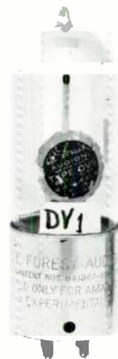
Example of a Shaw 4-pin base used on a De Forest type DV1 tube c. 1923.
