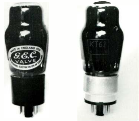
Osram KT63, the later version is on the right.
