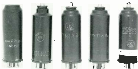
Metal-glass tubes by five different makers.
