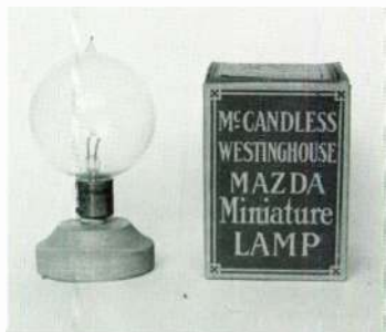
A McCandless motor-car lamp. The G-16½ bulb was also used for Audion manufacture.
