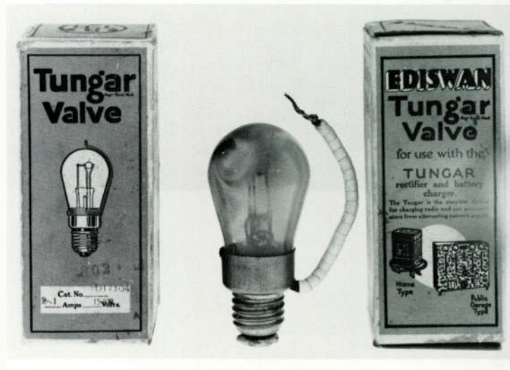
British-made 2-amp Tungar valve.
