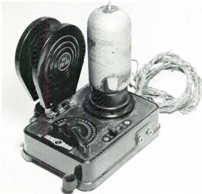
Loewe receiver using 3NFB tube.
