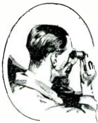
Illustration showing laboratory worker taking a temperature reading by means of the Pyrometer, an instrument for measuring temperatures which cannot be obtained by means of the ordinary thermometer system.
