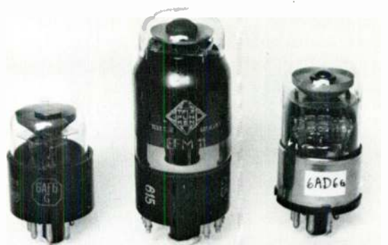
American types 6AF6G and 6AD6G Telefunken EF11M combined RF pentode and indicator tube (centre).
