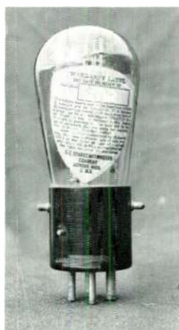
Sparton C181. Heater connections are to the side pins.
