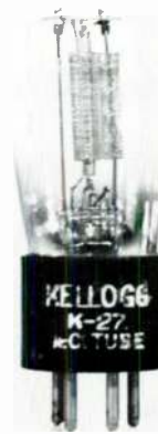
Kellogg version of the standard type '27 tube.
