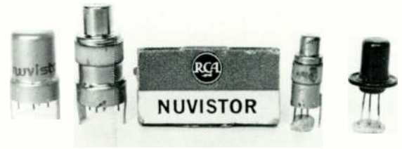
A group of three RCA Nuvistors compared with an early transistor (R.).
