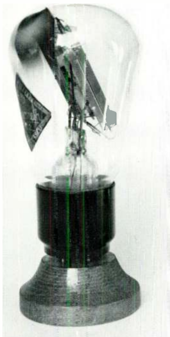
Standard-Micromesh R2, an early indirectly-heated rectifier.
