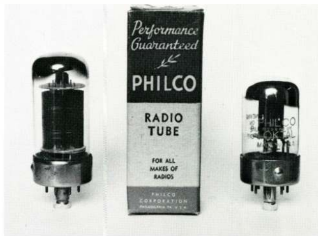
Philco 'Loktal' tubes, made by Sylvania.
