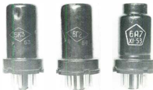
Russian metal tubes. Note open date coding indicating manufacture in 1953.
