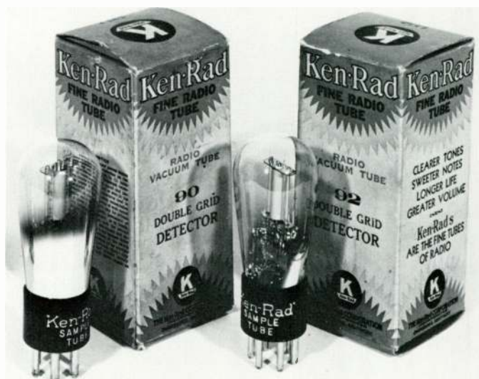
Types 90 and 92. Note base markings 'sample tube.'
