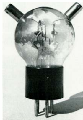
French Metal low-capacitance 'horned' tube c. 1925.
