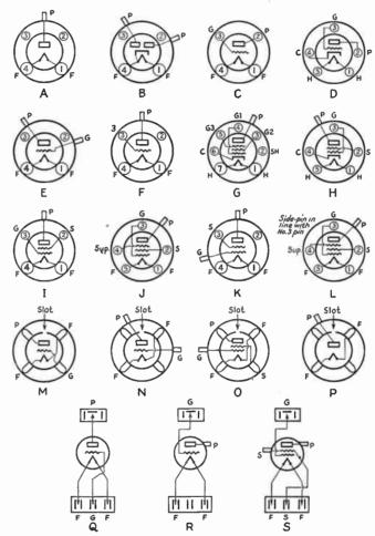
FIG. 519 — SOCKET CONNECTIONS FOR TRANSMITTING TUBES
