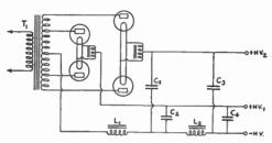
FIG. 1509 — A POWER SUPPLY CIRCUIT IN WHICH A SINGLE TRANSFORMER AND SET OF FILTER CHOKES IS MADE TO SERVE FOR DIFFERENT VOLTAGES
