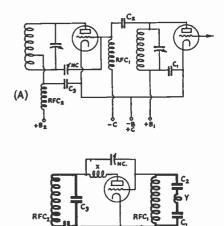
FIG. 833—HOW LOW-FREQUENCY PARASITIC OSCILLATIONS CAN BE GENERATED
