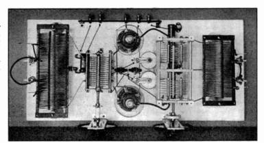
The complete circuit of the amplifier is shown in Fig. 925. Provision is made for link coupling to the grids and similar output coupling to an antenna tuning unit. Any of three bands, 3.5, 7 and 14 mc., can be selected by proper placement of the shorting clips on the grid and plate coils; shorting is from the center out-
