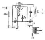
FIG. 1209-A — PENTODE PLATE-MODULATION CIRCUIT WITH SCREEN-DROP RESISTOR
