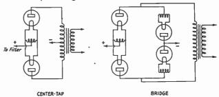
to get the load to divide evenly FIG. 1504 - CENTER-TAP AND BRIDGE RECTIFIER CIRCUITS In both circuits, the peak inverse voltage is equal to the total secondary voltage of the transformer multiplied by 1.4. Therefore, twice as much voltage can be obtained from the bridge as from the center-tap rectifier without exceeding the tube ratings. The tubes will pass the same load current in both cases.
