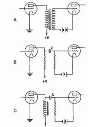
FIG. 507 — METHODS OF COUPLING BETWEEN AMPLIFIER TUBES
