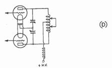
FIG. 831 — METHODS OF SWITCHING THE AM-PLIFIER PLATE TANK CIRCUIT FOR CHANGING BANDS
