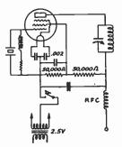
FIG. 1007—PENTODE CRYSTAL OSCILLATOR KEYING TO ELIMINATE CHIRPS
