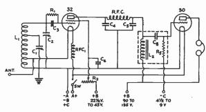
FIG. 707—THE TWO-TUBE RECEIVER DIAGRAM ADAPTED FOR TWO-VOLT TUBES
