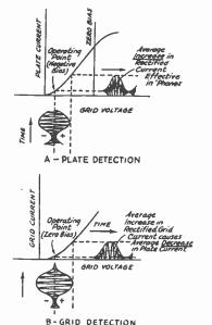
FIG. 513 — OPERATING CHARACTERISTICS OF PLATE AND GRID DETECTORS
