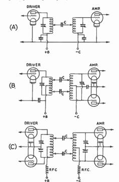
FIG. 816 — TRANSMISSION-LINE OR "MATCHED IMPEDANCE" COUPLING
