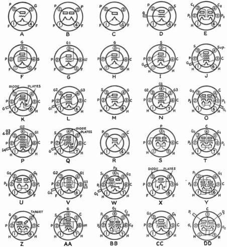
FIG. 517 -- BASE DIAGRAMS OF GLASS RECEIVING TUBES
