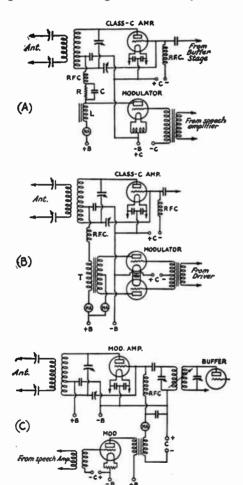
FIG. 1103 — CIRCUITS FOR THREE METHODS OF MODULATION
