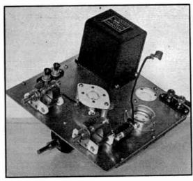
FIG. 703—THE "CHASSIS" OF THE TWO-TUBE RECEIVER
