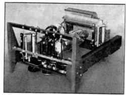
FIG. 914 — A BOTTOM VIEW OF THE RK-20 TRI-TET By-pass condensers are mounted on the brass-rod supporting structure.
