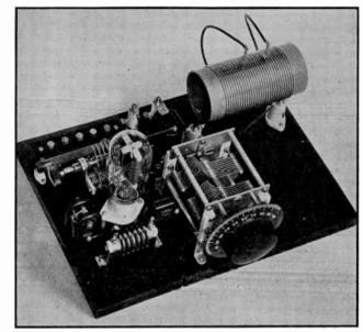
FIG. 921—A NEUTRALIZED AMPLIFIER FOR USE WITH A 10, 801 OR 830 TUBE
