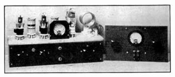
FIG. 934 — A GENERAL VIEW OF THE 50-WATT TRANSMITTER AND THE ANTENNA TUNING UNIT
