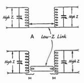
FIG. 409 — METHODS OF USING LINK COUPLING FOR IMPEDANCE MATCHING
