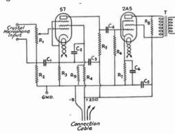
FIG. 1216 — CIRCUIT DIAGRAM OF THE SIMPLE GRID-BIAS OR SUPPRESSOR-GRID MODULATOR SHOWN IN FIG. 1201
