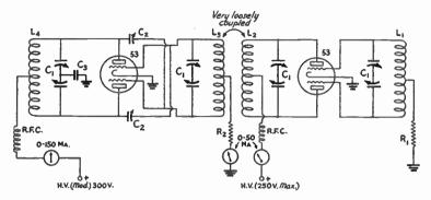
FIG. 1419 - CIRCUIT OF THE OSCILLATOR-AMPLIFIER TRANSMITTER USING DUAL TRIODES The antenna may be coupled with a conventional split antenna coil or by tapping the feeders on L<sub>4</sub>.
