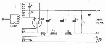
FIG. 1517 — A LOW-CURRENT POWER SUPPLY FOR REGENERATIVE OR T.R.F. RECEIVERS
