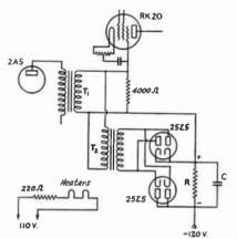
FIG. 1219 — CARRIER CONTROL WITH SUPPRES-SOR GRID MODULATION (VE2BC)
