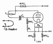
FIG. 1402—CIRCUIT SUITABLE FOR EXPERI-MENT ON 112 OR 224 MC.
