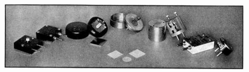
FIG. 806 - CRYSTALS AND CRYSTAL HOLDERS
