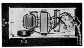
FIG. 1305 — UNDERNEATH THE "ACORN" RECEIVER all the items not above the chassis channel can be seen in this photograph. The location of the detector voltage control potentiometer is unconventional but convenient.
