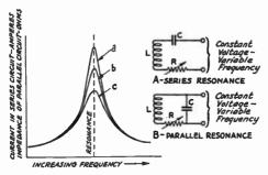
FIG. 402—CHARACTERISTICS OF SERIES-RES-ONANT AND PARALLEL-RESONANT CIRCUITS
