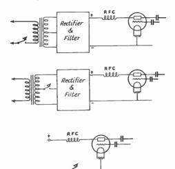
FIG. 1001 - PLATE-KEYING METHODS
