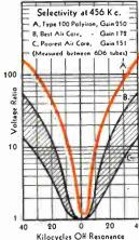
Small size Polyiron core I.f. transformers are particularly suitable for battery-oper-ated mobile receivers which must be built in the smallest space, yet have high gain.
