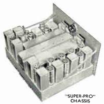
of a single front panel knob. One 6B7 is used in a combination fourth I.F. stage and diode second detector. A 6C6 is used as a low frequency beat oscillator. A 6B7 is used for amplified automatic volume control. A 76 is used in the first audio stage resistance coupled. Then comes a 42 used as a Class "A" driver stage. This is followed by two 42's as Class "AB" or "A Prime" push-pull audio output. Two rectifiers are used — a 5Z3 for plate voltage and a 1-V for grid voltage.
