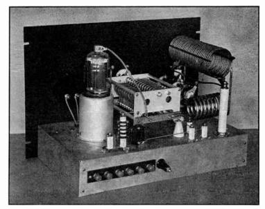
FIG. 926 — AN 803 BAND-SWITCHING AMPLIFIER FOR 3.5, 7 AND 14 MC.
