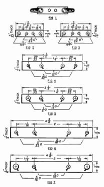
INSULATORS: A number of our standard condenser insulators are shown above. In addition to their obvious use as repair parts they may be used for a variety of other purposes such as supports for coils, spreaders, etc. The insulator shown in Fig. 1 is the same as Fig. 3, but has a metal solder lug riveted to each end. It is useful as a 5-meter lead-in spreader, or as a mounting for 5-meter inductances.
