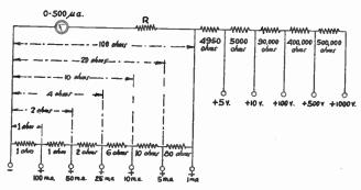
FIG. 1711 — A MULTI-RANGE VOLTMETER-MILLIAMMETER USING A 0-500 MICROAMMETER
