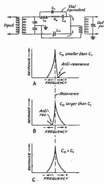
FIG. 618—THE REJECTION ACTION OF THE CRYSTAL FILTER CIRCUIT
