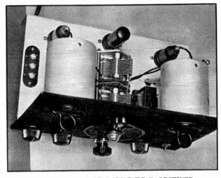
FIG. 717-718 -- A METAL-TUBE T.R.F. RECEIVER Such distinctive features as front-of-panel plug-in coils and metal tubes characterise this receiver design.
