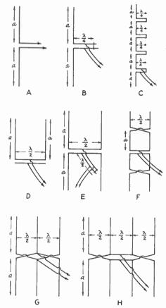
FIG. 1623 — A VARIETY OF DIRECTIVE ARRAYS INVOLVING THE USE OF PHASED ANTENNAS
