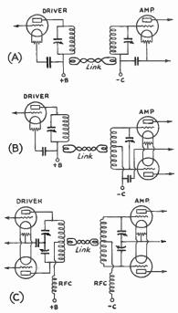
FIG. 817 — LINK COUPLING, USING A LOW-IMPEDANCE TRANSMISSION LINE
