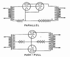
FIG. 506 — PARALLEL AND PUSH-PULL AMPLIFIER CONNECTIONS
