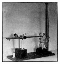
FIG. 1411 — A 112-MC. TRANSMITTER EMPLOY-ING THE CIRCUIT "C" OF FIG. 1407 Eimac 50T tubes are used in this set-up.
