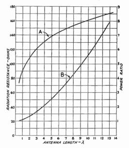
FIG. 1603 — THE IMPORTANT CURVES FOR HAR-MONICALLY-OPERATED HORIZONTAL ANTENNAS
