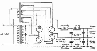
FIG. 1508—HIGH POWER BRIDGE RECTIFIER CIRCUIT. WHEN THE CENTER-TAP FILTER SHOWN IN DOTTED LINES IS USED, A TAP AT HALF MAXIMUM VOLTAGE WITH GOOD REGULATION IS PROVIDED. THE TOTAL CURRENT DRAWN FROM BOTH TAPS SHOULD NOT EXCEED 300 MA. FOR 866'S OR 1600 MA. FOR 872'S
