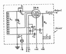
FIG. 1704 — CIRCUIT OF THE ELECTRON-COUPLED FREQUENCY METER
