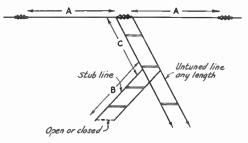
FIG. 1617 — ANTENNA SYSTEM WITH CORRECTIVE STUB FOR IMPEDANCE MATCHING
