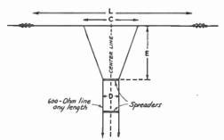
FIG. 1612—TWO-WIRE MATCHED-IMPEDANCE ANTENNA SYSTEM
