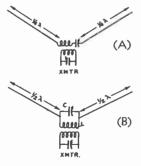
FIG. 1604 — DIRECT EXCITATION OF ANTENNAS, SHOWING CURRENT AND VOLTAGE FEED
