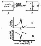
FIG. 405 — THE EQUIVALENT ELECTRICAL CIR-CUIT OF THE QUARTZ CRYSTAL PLATE
