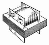
FIG. 1523 — A CONVENIENT METHOD OF ASSEMBLING THE WINDINGS ON A SHELL TYPE CORE
