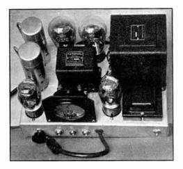
driver stage requirement of 50 volts peak grid swing is easily delivered by the two-stage speech amplifier with crystal microphone input. The total voltage amplification for the two stages is approximately 1400, adequate for close talking.
