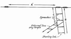
FIG. 1616 — IMPEDANCE-MATCHING ANTENNA SYSTEMS WITH QUARTER-WAVE OPEN WIRE MATCHING TRANSFORMERS
