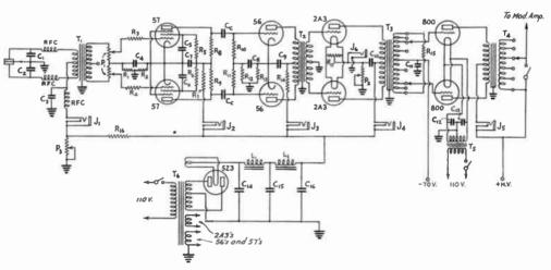
FIG. 1206 -- CIRCUIT OF THE 100-WATT AUDIO SECTION
