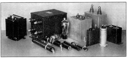
Chokes, transformers, condensers, rectifiers and resistors—the essentials of all power supply systems.
