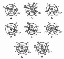
FIG. 518 — BASE DIAGRAMS OF METAL RECEIV-ING TUBES
