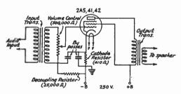
FIG. 607 — A TYPICAL PENTODE POWER AMPLIFIER CIRCUIT WITH VOLUME CONTROL
