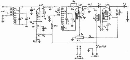
FIG. 720 - CIRCUIT DIAGRAM OF THE METAL-TUBE T.R.F. RECEIVER
