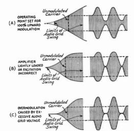
FIG. 1217 — OSCILLOSCOPE PATTERNS REPRESENTING PROPER AND IMPROPER GRID-BIAS OR SUPPRESSOR-GRID MODULATION
