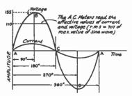
FIG. 306—REPRESENTING SINE-WAVE ALTER-NATING VOLTAGE AND CURRENT
