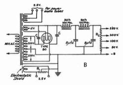
FIG. 1515 — WIRING DIAGRAMS FOR RECEIVER POWER SUPPLIES
