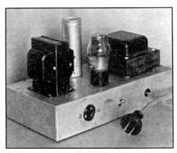
FIG. 1519 — A HEAVY-DUTY RECEIVER POWER-SUPPLY
