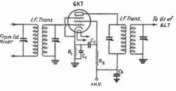
FIG. 1324 - WIRING OF THE SUGGESTED I.F. **AMPLIFIER**
