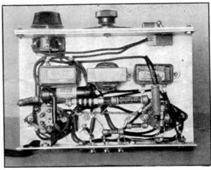
FIG. 710 — BOTTOM VIEW OF THE 6F7-41 TUBE RECEIVER CHASSIS
