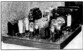
FIG. 1205 - THE SPEECH-AMPLIFIER AND 100-WATT CLASS-B MODULATOR
