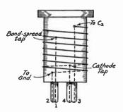
FIG. 706 — COIL SOCKET CONNECTIONS AND THE METHOD OF BRINGING OUT COIL TERMINALS
