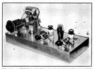
FIG. 931—A THREE-BAND TWO-STAGE PENTODE TRANSMITTER A 59, pentode or Tri-tet, drives an RK-20 amplifier, using 3.5- and 7-mc. crystals. No buffer stages are needed. This outfit was built by WIAF.
