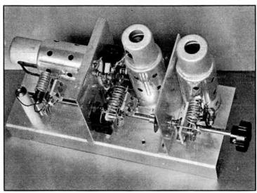
FIG. 1318 - THE GLASS-TUBE CONVERTER UNIT
