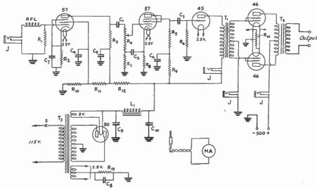
FIG. 1204 — CIRCUIT DIAGRAM OF THE SPEECH AMPLIFIER AND ECONOMY CLASS-B MODULATOR The power supply furnishes plate and filament power for the first three tubes only; the Class-B stage must be supplied from a separate source. If a power transformer having an additional 2.5-volt winding is used, filaments of the 46's may be heated from the second winding.
