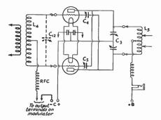
FIG. 1214 — GRID CIRCUIT CHANGES IN THE FINAL AMPLIFIER OF THE GENERAL-PURPOSE TRANSMITTER TO FIT IT FOR GRID-BIAS MODULATION
