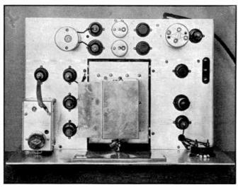
FIG. 730 — PLAN VIEW OF THE 12-TUBE S.S. SUPERHET DESCRIBED IN THE TEXT
