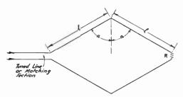
FIG. 1627 — THE GENERAL ARRANGEMENT OF THE "DIAMOND" OR "RHOMBIC" DIRECTIVE ARRAY
