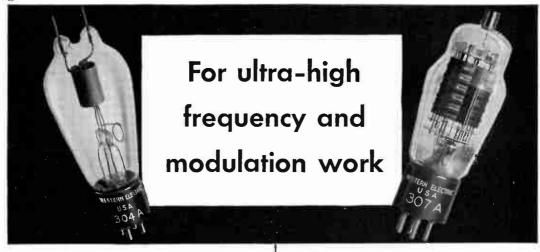
The Western Electric 304A is a triode developed especially for ultra-high frequency work. As a radio-frequency oscillator or power amplifier, it may be used at full rating at frequencies up to 100 megacycles—at reduced ratings up to 300 megacycles. Also suitable for use at audio frequencies, particularly in Class B audio amplifiers or modulators.
