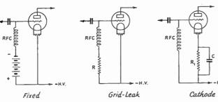
FIG. 825 — AMPLIFIER BIASING METHODS A "B" eliminator or "C" power pack can be substituted for the battery provided its bleeder resistance is not too high. See Chapter Fifteen for information on the design of "C" power packs.
