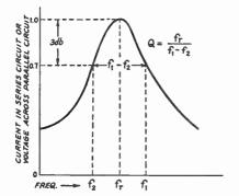
FIG. 403 — HOW THE VALUE OF Q IS DETERMINED FROM THE RESONANCE CURVE OF A SINGLE CIRCUIT
