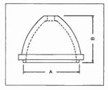
H.F. BUSHING. Larger in size than the bushings described above, and shaped to conform to the lines of electrical stress, these Steatite insulators are suitable for higher H.F. voltages. Prices are per pair, with metal fittings.
