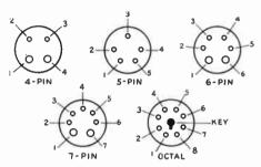
FIG. 516 - TUBE-BASE PIN NUMBERING SYSTEM
