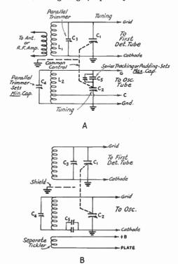
FIG. 613 — CONVERTER CIRCUIT TRACKING METHODS
