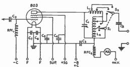
FIG. 927 - CIRCUIT DIAGRAM OF THE 803 AM-PLIFIER
