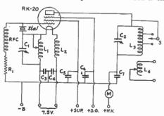
FIG. 913 - THE RK-20 TRANSMITTER CIRCUIT DIAGRAM
