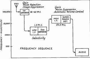
FIG. 1319 — ILLUSTRATING THE PRINCIPLE USED IN THE SUPER-INFRAGENERATOR RECEIVER
