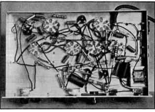
FIG. 724—A BOTTOM VIEW OF THE SIX-TUBE SUPERHET By-pass condensers and resistors are placed in the most convenient locations. The detector output transformer is mounted on the side wall of the chassis, and can be seen in the lower right-hand corner.
