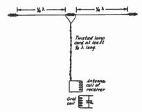
FIG. 1621 - DOUBLET RECEIVING ANTENNA
