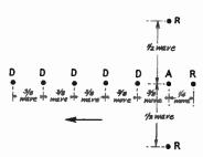
FIG. 1628—SHOWING THE ARRANGEMENT OF THE ANTENNA, REFLECTOR AND DIRECTOR ELEMENTS IN A "YAGI" DIRECTIVE SYSTEM
