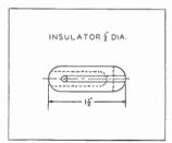
STRAIN INSULATOR. This aircraft-type insulator, in spite of its short leakage path, has a variety of uses in small portable, mobile and police installations. Being loaded in compression, the insulator provides great mechanical strength.
