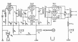
FIG. 936 - CIRCUIT DIAGRAM OF THE TRANS-MITTER
