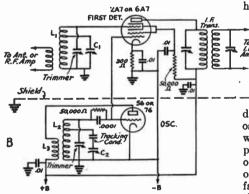
FIG. 609 — THESE FREQUENCY-CONVERTER CIR-CUITS ARE FOR USE WITH PENTAGRID TUBES
