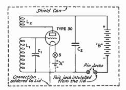
FIG. 1702 - WIRING DIAGRAM OF THE MONITOR
