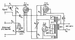
FIG. 1715 — A VACUUM TUBE VOLTMETER WITH D.C. AMPLIFIER
