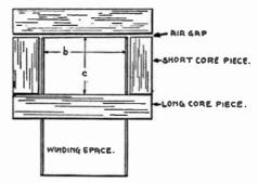
FIG. 1524 — CORE ARRANGEMENT FOR FILTER CHOKE COILS
