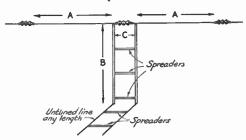
FIG. 1613 — THE "Q" ANTENNA WITH QUARTER-WAVE MATCHING SECTION USING SPACED TUBING
