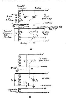
Fig. 418 — Converter circuit tracking methods. Approximate circuit values for 450- to 465-kc. intermediates with tuning ranges of approximately 2.15-to-1,  $C_1$  and  $C_2$  having a maximum of 140  $\mu$ dd. and the total minimum capacitance, including  $C_3$  or  $C_4$ , being 30 to 35  $\mu$ dd.
