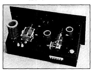
best to use some sort of indicator in the load circuit, such as an r.f. ammeter in the feeder, to assist in tuning for maximum output. Heavy loading should not affect the oscillator's keying characteristics. When loaded so that the tube draws 75 ma., the output should be close to 20 watts on any of the three bands under the conditions described.
