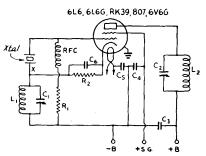
Fig. 506 — Tri-tet oscillator circuit, using pentodes or beam tetrodes. C<sub>1</sub> and C<sub>2</sub>, 200-μμfd. variables; C<sub>3</sub>, C<sub>4</sub>, C<sub>6</sub>, 0.001 to 0.01 μfd. by-passes, not critical; R<sub>1</sub>, 20,000 to 100,000 ohms; R<sub>2</sub>, 400 ohms for 400- or 500-volt operation.
