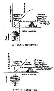
Fig. 332 — Operating characteristics of plate and grid detectors.
