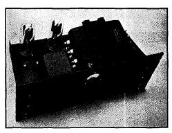
Fig. 1224 — A chassis arrangement for a higher-power Class-B modulator. This unit has a filament transformer for the tubes mounted on the chassis, as well as the input and output transformers. In cases where the input transformer is included with the speech amplifier, less chassis space is needed. The tubes are placed to the rear where ventilation is good.
