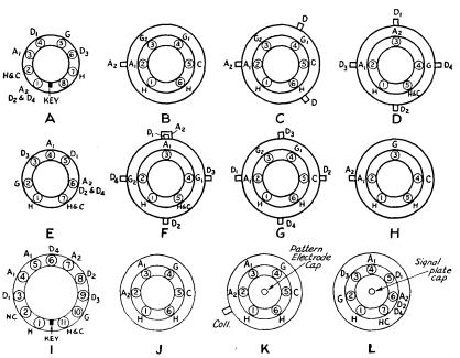
SOCKET CONNECTIONS FOR CATHODE-RAY TUBES
