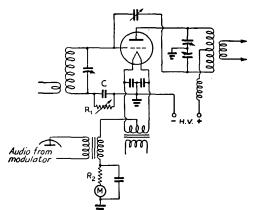
Fig. 609 — Cathode modulation of a Class-C triode amplifier. R1, grid leak; C, audio by-pass; R2, cathodebias resistor for initial bias, also by-passed for audio frequencies.
