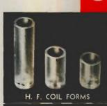
For ultra high frequency work, where very low losses are essential, these small Victron coil forms will be found extremely useful. They can be readily drifled and grooved with ordinary tools, and firmly cemented with National Coil Dope without impairing electrical characteristics.
