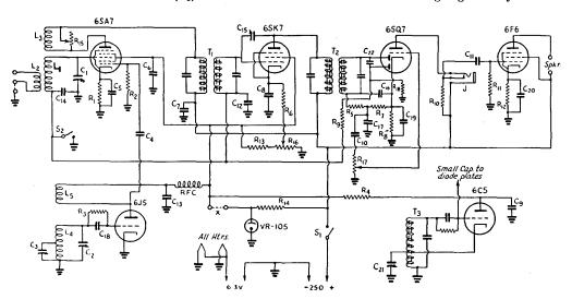
Fig. 815 - Circuit diagram of the regenerative superhet.
