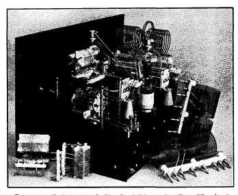
Fig. 1040 — Grid-circuit end of hand-switching push-pull amplifier showing switching arrangement and the 1.75-Mc. padder.
