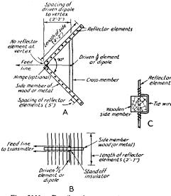
Fig. 3010 — Details of construction of a corner reflector antenna system with grid-type reflector. The reflector elements are stiff wire or tubing. The dimensions are for 224 Mc., and should he doubled for 112 Mc. (See Table 1.) The gain of the system is close to 10 db.
