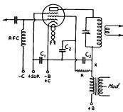
Fig. 605 — Plate-and-acreen modulation of a pentode Class-C r.f. amplifier.
