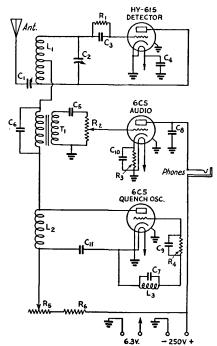
Fig. 2723 — Plug-in coil receiver circuit.
