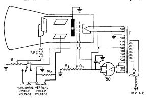
No intensity control provision is made in this oscilloscope — it is operated at maximum at all times. Accordingly, it is quite important that some provision be included for switching off the electron beam, reducing the spot intensity, or swinging the beam to one side of the scope with d.c. bias during periods of no transmission, when the pattern would be confined to a thin, bright line or a small spot of high intensity. This must be done to prevent "burning" the screen of the c.-r. tube.
