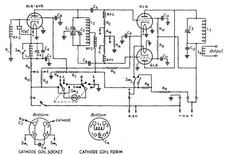
Fig. 1008 — Circuit diagram of the two-stage 6L6 transmitter. condenser, C<sub>7</sub>, C<sub>8</sub>, C<sub>9</sub>, C<sub>10</sub>, C<sub>11</sub>, C<sub>12</sub> — 0.01- R<sub>8</sub>, R<sub>9</sub> —
