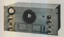
All models of the HRO are supplied with 6.3 volt heater type tubes. Table models and accessories are finished in black wrinkle enamel.
