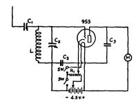
Fig. 1725 - Simple field-strength meter.
