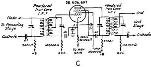
Fig. 419 - I.F. amplifier circuits for three types of transformers. A, double-tuned; B, triple-tuned; C, high-gain iron core.
