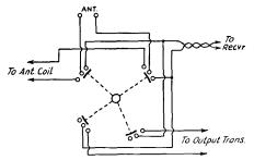
Fig. 821 — The converter antenna switch wiring diagram.
