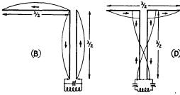
Fig. 2213 — Half-wave antennas fed from resonant lines. A and B, end feed with quarter- and half-wave lines; C and D, center feed. The current distribution is shown for all four cases.
