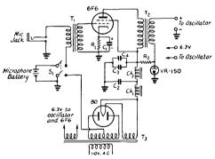
Fig. 1202 - A 4-watt modulator and associated power supply.
