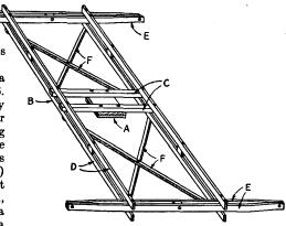
Fig. 2506 — Easily-built supporting structure. Made chiefly of 1 by 2's, the structure is strong yet lightweight. Antenna elements are supported on stand-off insulators on the "E" arms. The length of the "D" sections will depend upon the element spacing.
