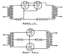
Fig. 325 — Parallel and push-pull amplifier con-
