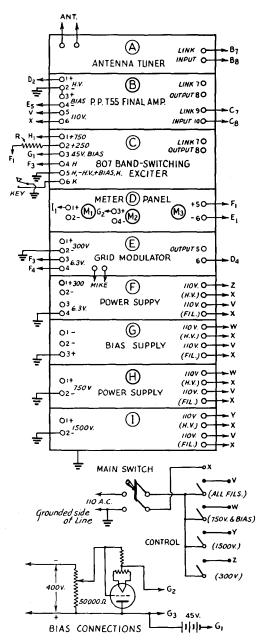
Fig. 1308 — Complete layout of grid-modulated 'phone-c.w. transmitter.
