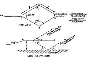
$\emptyset$  = Angle of tilt (Degrees) L= Length of one Side (WAVELENGTHS)  $\Delta$  = WAVE Angle (Degrees) H= Height (WAVELENGTHS)
