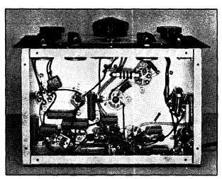
Fig. 817 — The below-chassis wiring is shown in this view of the 7-tube receiver.
