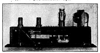
Fig. 1206 — The hottom view shows the tube- and transformer-mounting used in the 3-watt amplifier.
