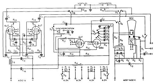
Fig. 1733 - Complete circuit diagram of sweep-circuit oscilloscope.
