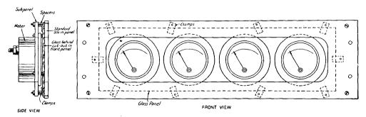
Fig. 1303 — Safety panel for meters. The meters are mounted in the usual manner on an insulating suh-panel spaced back of a glass-covered opening in the front panel. The glass is fastened in place with metal clamps or tabe fastened to the front panel with small screws or pins. The front panel is of standard size 19 in. by 5½ in.
