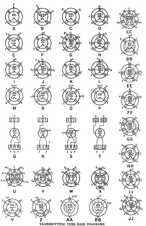
Bottom views are shown. F denotes filament, H heater, C cathode, G grid, S screen (or shell in octal-based tubes), P plate, G<sub>1</sub>, G<sub>2</sub>, G<sub>3</sub>, etc., denote grids numbered in order from cathode outward; numeral subscripts in multi-unit tubes denote elements common to one unit.
