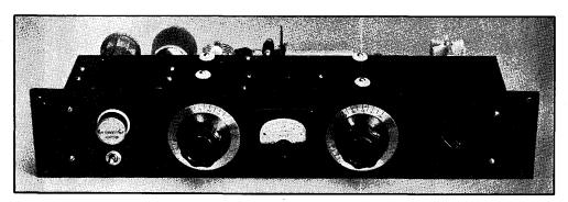
Fig. 1016 — The two-tube plug-in coil exciter is built to conserve space in the relay rack. The panel is 3½ in. by 19 in. A clearance hole is cut in the left end of the panel for the crystal socket which is mounted in the chassis directly above the cathode-circuit switch. The left-hand dial controls the tuning of the oscillator plate
