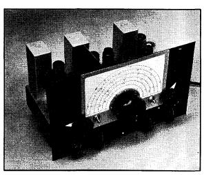
Fig. 814 — A 7-tube superhet using regeneration to give singlesignal reception and improve image ratio. The dial (National ANC) may be directly calibrated for each amateur band.
