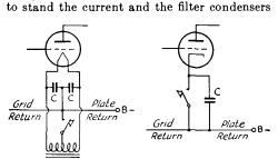
Fig. 1507 — Center-tap keying. Keying for filament type tubes is shown at the left and for cathode types at the right. The by-pass condensers, C, should be about 0.001  $\mu\mu$ fd. and capable of withstanding full plate voltage. They are necessary to furnish an r.f. return to ground. Full plate voltage appears across the key, so a relay should be substituted for the key if high voltages are used.
