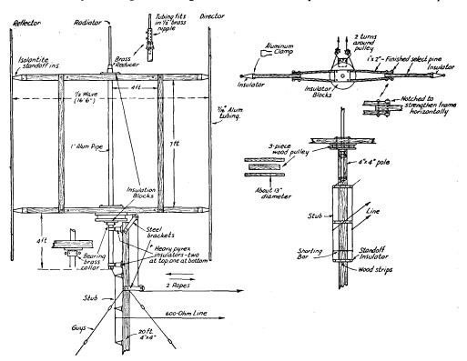
Fig. 2505 — A practical vertical-element rotatable array for 28 Mc. No special feeder-contact mechanism is needed, since the driven antenna is fixed. The reflector and director, parasitically excited, rotate around it. Close-spaced elements may be used if desired.
