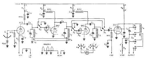
Fig. 1022 - Circuit diagram of the 807 band-switching exciter.
