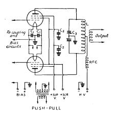
Fig. 510 — Tetrode-pentode r.f. amplifier circuits.  $C_1 - 0.01~\mu fd.$ ;  $C_2 - 0.001~\mu fd.$  or larger;  $C_8$ -L — See section on tank-circuit design.
