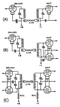
Fig. 509 — Link coupling, using a low-impedance transmission line. The link may be twisted lamp cord or consist of a pair of closely-spaced, but not twisted, wires. A concentric line is the best form.
