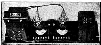
Fig. 1221 — A rear view of the modulator of Fig. 1220, showing how the components are supported. The panel is relay-rack size, 5½ inches high.
