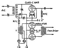
Fig. 604 - Transformer-coupled plate modulation.
