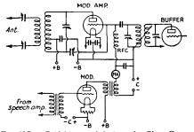
Fig. 607 — Grid-bias modulation of a Class-C amplifier.
