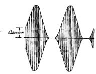
Fig. 603 - An overmodulated wave.
