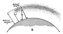
Fig. 2101 — Illustrating ground-wave and sky-wave transmission of radio waves. The density of the dots indicates that the electron density in the ionosphere increases and then decreases as the altitude becomes greater. This is a simplified representation; actually there are other ionized layers which affect different frequencies in different ways.
