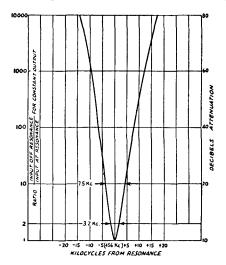
Fig. 401 — Selectivity curve of a modern superheterodyne receiver. The relative response is plotted against deviations above and below the resonance frequency. The scale at the left is in terms of voltage ratios; the corresponding decibel steps (see Chapter 20) are shown at the right.
