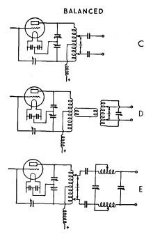
rent in the line measured. The tap positions, coupling between the coils and tuning of both tank circuits are then adjusted to give maximum line current with normal tube plate current.
