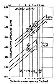
Fig. 2202 — Graphical table of characteristic impedances of typical spaced-conductor transmission lines. Use outside diameter of tubing.
