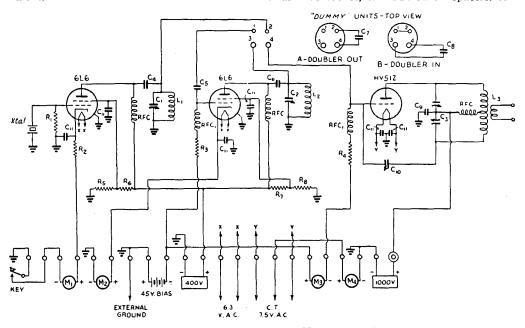
Fig. 1026 — Circuit diagram of 100- to 175-watt transmitter.
