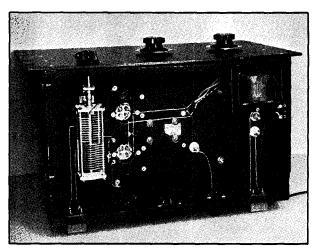
ing from a single-button carbon microphone. A meter switch allows metering of the oscillator, amplifier, or combined amplifier and modulator currents. The on-off switch on the panel also cuts the microphone current when the transmitter is not on the air.
