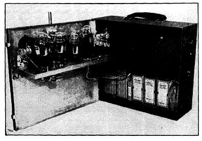
oscillation is accomplished by shorting out the larger of the two grid-leak resistances,  $R_2$ , by a set of contacts on the ganged send-receive switch. A second set of contacts connects the HY615 plate to the plate winding of the transceiver transformer, for receiving, or to the 6G6G plate circuit for transmitting. A third set of contacts grounds one side of the microphone jack during the transmission period.  $R_5$  is the regeneration control as well as the volume control.
