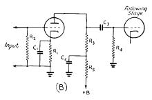
Fig. 612 - Resistance-coupled voltage amplifier circuits. A, pentode; B, triode. Designations are as follows:
