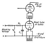
Fig. 1509 — Vacuum-tuhe keying. The series method is simple but does not completely cut off the current flow. It may be used in some applications where the following stage is heavily biased. C may be between 0.25 and 1.0 µfd. Resistor R should be adjusted to cause the plate current to drop to a minimum when the key is open. A variable resistor of 50,000 ohms should give enough range.
