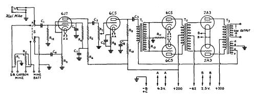
Fig. 1214 - Circuit diagram of the 15-watt speech amplifier.
