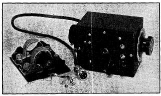
Fig. 2710 — This compact converter unit works on both 28 and 56 Mc. with any car broadcast receiver. The steering-column mounting, fastened to one side of the case, can be constructed from metal strip.
