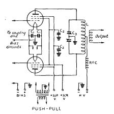
Fig. 510 — Tetrode-pentode r.f. amplifier circuits.  $C_1$  —  $0.01~\mu fd.$ ;  $C_2$  —  $0.001~\mu fd.$  or larger;  $C_3$ -L — See section on tank-circuit design.
