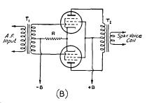
Fig. 408 — Audio power output amplifier circuits.
