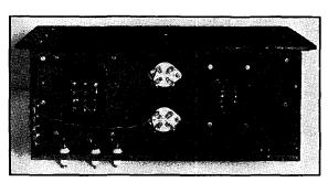
Fig. 1223 — The simplicity of modulator wiring is evident in this view of the bottom of the chassis of the modulator unit shown in Fig. 1222.
