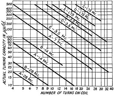
Fig. 517 - Coil-winding data for ceramic transmitting-type forms. Curve - ceramic form 21/2inch effective diameter, 26 grooves, 7 per inch; Curve B — same as A, but with turns wound in alternate grooves; Curve Cramic form 27%-inch effective diameter, 32 grooves, 7.1 turns per inch, app.; Curve D — ceramic form 4-inch effective diameter, 28 grooves, 5.85 turns per inch, app.; Curve E ceramic form 5-inch effective diameter, 26 grooves, 7 per inch. Coils may be wound with No. 12 or No. 14 wire.
