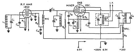
Fig. 2708 - The 1852-6K8 converter circuit,
