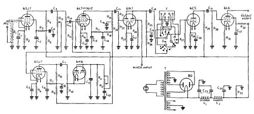
Fig. 1217 — Circuit diagram of speech amplifier with audio filter and compression.
