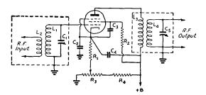
Fig. 411 — The circuit of a tuned radio-frequency amplifier. Circuit values are discussed in
