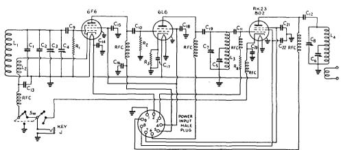
Fig. 1011 — Circuit diagram of the e.c.o. exciter.
