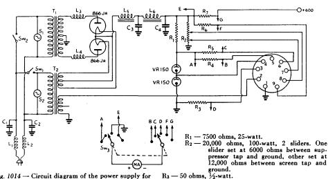
Fig. 1014 - Circuit diagram of the power supply for the e.c.o. unit.
