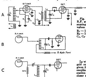
quent heavy loading of the detector will not allow the maximum possible r.f. selectivity. The coupling adjustment should therefore be varied to give the desired optimum performance considering both selectivity and sensitivity.
