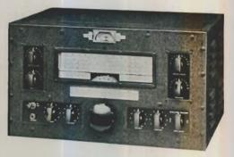
NHU Receiver, table model, complete with tubes, 8" speaker with cabinet and coils covering from 27 to 62 MC, but without power supply, black finish.
