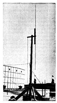
Fig. 3003 — The 56-Me. antenna at W2USA, dimensions of which are given in Fig. 3002.
