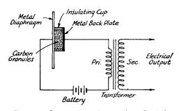
Fig. 601 — Construction and connections of a single-button microphone and its transformer.
