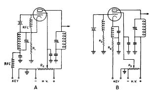
Fig. 1511 — Cathode keying for tri-tet oscillator. Typical values for 6L6: R<sub>1</sub> — 50,000 ohms; R<sub>2</sub> — 20,000 ohms. B—Cathode keying for grid-plate oscillator. Typical values for 6L6: R<sub>8</sub>—50,000 ohms; R<sub>4</sub>—400 ohms; Rs - 20,000 ohms.
