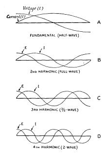
Fig. 2301 — Current and voltage distribution along an antenna operated at various harmonics of its fundamental resonant frequency.
