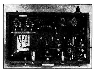
Fig. 1015 — Bottom view of power supply showing line-filter and hash-filter chokes and the meter switching. The terminal at the rear of the chassis is for external connection to the 600-volt line.
