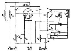
Fig. 1729 — Audio signal generator circuit diagram.
