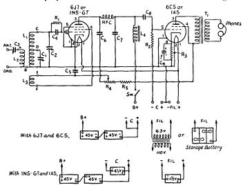
Fig. 803 - Wiring diagram of the two-tube receiver.
