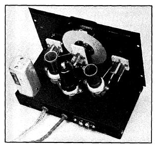
Fig. 822 — Top view of the converter. L<sub>1</sub> and L<sub>2</sub> are to the right and left of the 6K8. The output transformer stands at the left. The power-cable output leads and antenna terminals may be seen along the rear wall of the chassis.
