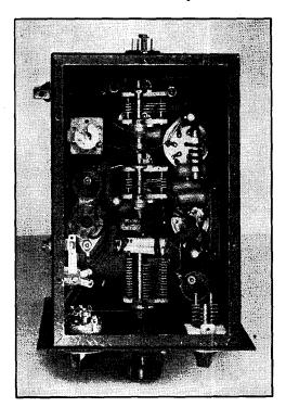
Fig. 1012 — Bottom view with bottom plate removed showing arrangement of components under the chassis. The removable top and bottom plates make the assembly easy. Shielded single conductor is used for the key-circuit leads.
