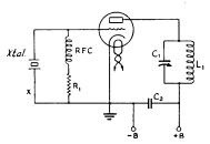
Fig. 503 — Triode crystal oscillator. The tank condenser C<sub>1</sub> may be a 100-μμfd. variable, with L<sub>1</sub> proportioned so that the tank will tune to the crystal frequency. (See coil charts, Figs. 516-517.) C<sub>2</sub> should be 0.001 μfd. or larger. The grid leak, R<sub>1</sub>, will vary with the type of tube; high-μ types take lower values, 2500 to 10,000 ohms, while medium and low-μ types take values of 10,000 to 25,000 ohms.
