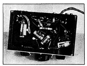
Fig. 813 — Additional parts for the audio output stage can readily be identified in this sub-chassis view of the receiver.
