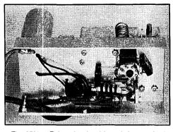
Fig. 2709 - Below-chassis wiring of the metal-tube converter. The 1852 socket may be seen at the right.
