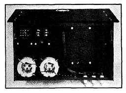
Fig. 1225 — Bottom view of the modulator of Fig. 1224. Mounting the sockets below the chassis saves panel height and conceals the wiring. The output terminals should be protected as described in connection with Fig. 1222.
