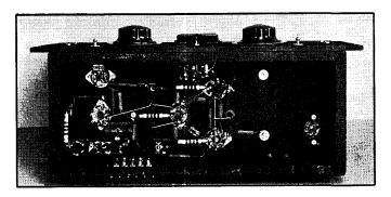
17. The cathode circuits of both stages are keyed simultaneously.
