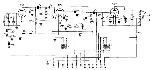
Fig. 1029 - Circuit diagram of the 250-watt transmitter.
