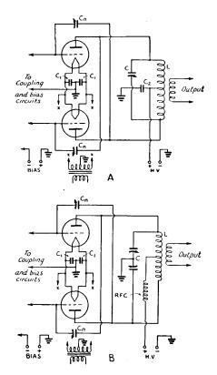
shaft are avoided. While an amplifier using the circuit of B may appear easier to drive compared to circuit C because of effects of regeneration when the tank circuit of B is tuned slightly off resonance, with proper neutralization, there should be no difference. With pushpull amplifiers, the circuit of Fig. 512-B is also preferred for the same reasons.
