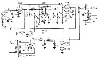
Circuit diagram of the frequency standard.
