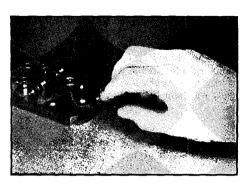
Fig. 205 — Illustrating the correct position of the hand and fingers for the operation of a telegraph key.
