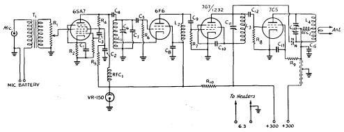
Fig. 2906 — Wiring diagram of the 56-Mc. f.m. transmitter.
