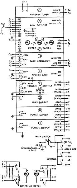
D - Modulator (Fig. 1222), TZ40's operating at 1250 v. plate and 4.5 v. bias. Output transformer set for 14,000 to 7200 ohms.
