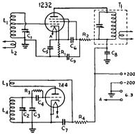
5 Mc.: 45 turns No. 30 d.s.c. closewound; coupling coil is 14 turns No. 30 d.s.c. closewound
