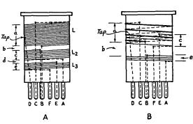
Fig. 805 — Tube and socket connections for the receiver. All of the coils except No. 5 for metal tubes and No. 4 for battery tubes are wound as at A; B shows how coil No. 5 for metal tubes and No. 4 for battery tubes are wound. All coils for any one range must be wound in the same direction. In the table (p. 110) the values given in parentheses apply only to the battery-tube coils, otherwise the values are the same for both types of tubes.
