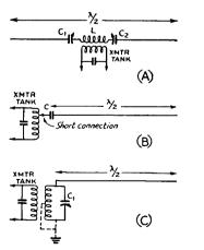
Fig. 2201 — Methods of direct feed to the half-wave antenna. A, current feed, series tuning; B, voltage feed, capacity coupling; C, voltage feed with inductively coupled antenna tank. In A, the coupling apparatus is not included in the antenna length.
