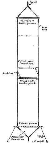
Fig. 2504 — A simple arrangement for a rotatable directive antenna. It may be suspended from any suitable support, such as another antenna, having the requisite height. The antenna shown is a 28-Me. extended double Zepp with reflector.
