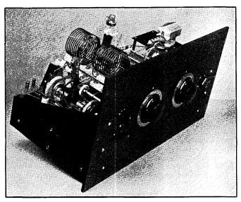
Fig. 1037 — The panel of the band-switching amplifier is  $10\frac{1}{2}$  inches by 19 inches. The dials control the plate- and grid-tank condensors. The uppermost of the two small knobs to the left is for adjusting the variable link-output coupling, while the lower one is for the plate band switch. The grid hand switch knob is to the right.
