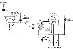
Fig. 2718 - Circuit diagram of the 112-Mc. battery receiver.
