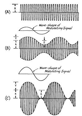
Fig. 602 — Graphical representation of (A) unmodulated carrier wave, (B) wave modulated 50%, (C) wave modulated 100%.
