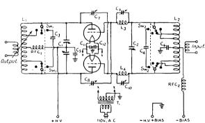
Fig. 1039 — Circuit diagram of the 450-watt band switching amplifier.
