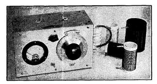
The absorption frequency meter is particularly useful for checking the tuning of a transmitter stage (to insure that the stage is not tuned to a harmonic instead of the desired frequency, for instance), for determining the frequency of parasitic oscillations in the transmitter, and for finding the frequency range covered by various oscillators.
