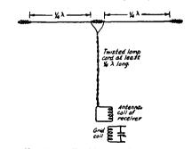
Fig. 2508 — Doublet receiving antenna.
