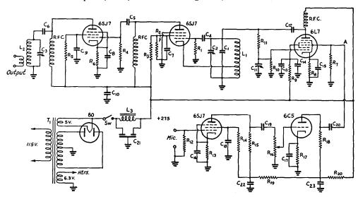
Fig. 2903 — Circuit diagram of the control unit for use with normally crystal-controlled transmitters.
