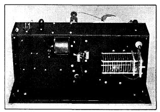
Fig. 1041 - The chassis for the bandswitching amplifier is 10 inches by 17 inches by 3 inches. The plug-in air padding condenser for 1.75 Mc. is spaced with equal distance between top and bottom of the chassis. Filament bypass condensers are soldered to the terminals of the fibre lug strip to which transformer terminals filament are anchored.
