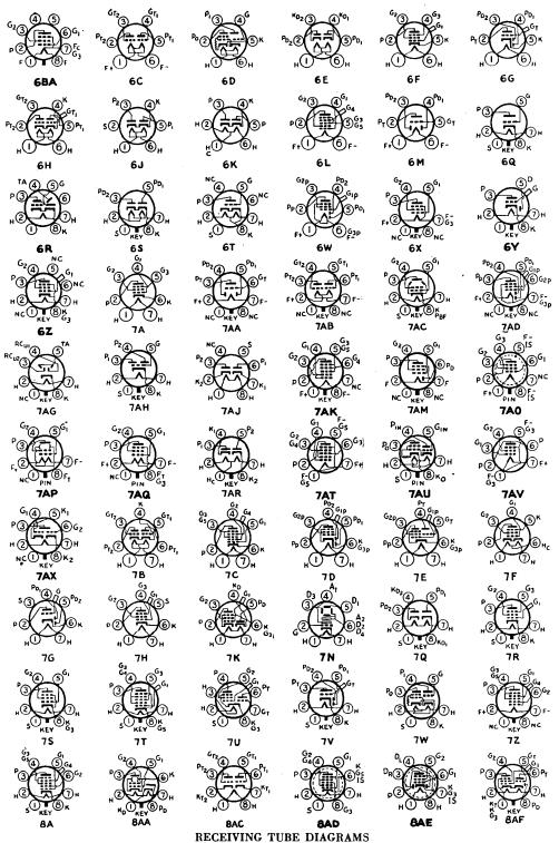
Bottom views are shown. Terminal designations on sockets are as follows: P = Bayonet Pin H = Heater P = Plate (Anode) S = Shell
