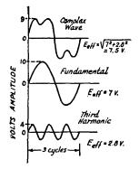
Fig. 319 — A complex wave and its sine-wave components.
