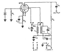
Fig. 1712 — Crystal calibrator circuit diagram.  $C_1 = 35 \cdot \mu_{\mu} fd$ , midget variable (Hammarlund HF-35).  $C_2 = 100 \cdot \mu_{\mu} fd$ , mica trimmer (Hammarlund CTS-85).  $C_3$ ,  $C_4$ ,  $C_5 = 0.1 \cdot \mu fd$ , 400-volt paper.  $C_6 = 0.001 \cdot \mu fd$ , midget mica.
