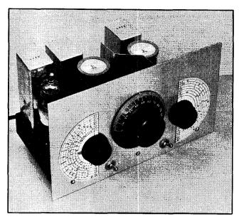
Fig. 806 — The three-tube superbet, designed for either a.c. or d.c. heater operation and 90-volt "B" hattery plate supply.
