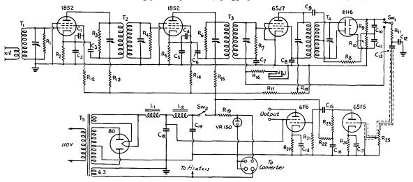
Fig. 2914 Wiring diagram of the 5-Mc. f.m /a.m. amplifier.
