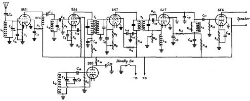
Fig. 2715 — 56-Mc. superhet circuit diagram.
