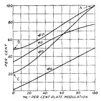
Fig. 609-A — Cathode-modulation curves, in terms of percentage of plate modulation against per eent of Class-C telephony tube ratings.
