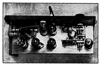
Fig. 2833 — A plan view of the outfit. Transmitter at left, receiver at right. A quarter-wave rod antenna fits into the receptacle mounted by standoff insulators on the front panel.
