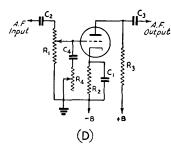
Fig. 407 — Audio amplifier circuits for voltage amplification and headphone output.
