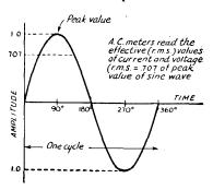
Fig. 308 — Representing sine-wave alternating current and voltage.
