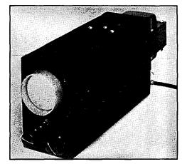
1730 — Oscilloscope using 902 2-inch tube, housed in a 5 x 10 x 3-inch chassis with bottom plate.
