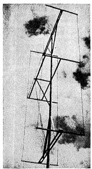
ultra-high frequencies. A possible exception to this rule is the antenna of Fig. 3006, which, while shown with quarter-wave spacing, can be used with spacing as close as one-eighth wavelength when tuned feeders are used. The gain will be slightly higher with the closer spacing but the antenna must be built more rigidly because the closer spacing will make relative motion of the elements more noticeable.
