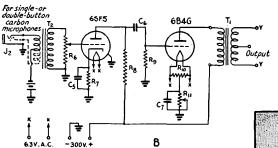
The amplifier is constructed on a standard black-crackle chassis 17 inches long, 4 inches deep, and 3 inches high. Tubes and output transformer, instead of being placed in the conventional arrangement on top of the chassis, are mounted on the rear flange, while the front flange is screwed against the back of mounting panel as in ordinary chassis-panel units. With this layout, a  $3\frac{1}{2}$ -inch relay-rack panel is adequate, and rack-space compactness results.
