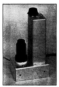
Fig. 825 Top view of the beat oscillator assembly.
