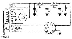
Fig. 1121 - Circuit diagram for receiver power supplies.
