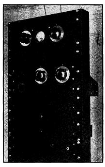
Fig. 1311 - 200-250-watt transmitter for c.w. plate-modulated phone. Rear view shown in Fig. 1313 and complete layout in Fig. 1312.
