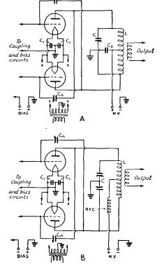
shaft are avoided. While an amplifier using the circuit of B may appear easier to drive compared to circuit C because of effects of regeneration when the tank circuit of B is tuned slightly off resonance, with proper neutralization, there should be no difference. With pushpull amplifiers, the circuit of Fig. 512-B is also preferred for the same reasons.
