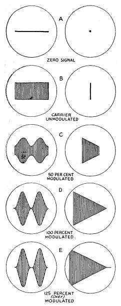
Fig. 1603 — Wave-envelope (left) and trapezoidal (right) oscilloscope patterns.
