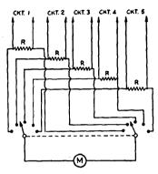
Fig. 1304 — Method of switching a milliammeter to various circuits with a two-gang switch. The control shaft should be well insulated from the contacts and grounded. The resistances should be ten to twenty times the resistance of the meter; 20 ohms will usually be satisfactory.
