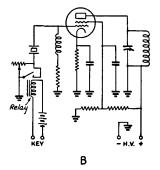
Fig. 1513 — Crystal keying circuits.
