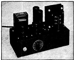
Fig. 1207—A low-cost speech-amplifier or low-power modulator with a maximum audio output of 20 watts. The 6SJ7 is in the left near corner of the chassis, with the 6J5 to its right, just above the volume control.
