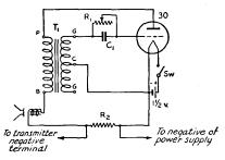
Fig. 1518 — An audio-oscillator keying monitor.
