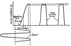
Fig. 329 — Class-C amplifier operation.
