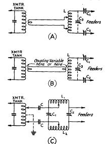
Fig. 2215 — Antenna coupling systems without movable coils. A and B, link-coupled circuits for series and parallel tuning; C, balanced low-pass filter. In A and B, dotted lines show connections for parallel tuning when called for; in such case the series condensers, C1 and C2, may be set at maximum capacity or shortcircuited. Constants for L, C1, C2 and C8 are the same as for inductive coupling, and are discussed in the text.
