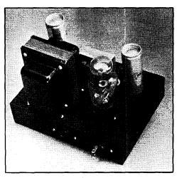
Fig. 1102 - This small unit delivers 480 volts at fullload current of 130 ma. with 0.3% ripple and measured regulation of 17%. By converting to choke-input filter hy inserting a similar choke between rectifier and present filter, the output voltage would be reduced to about 300 volts. The chassis measures 7 in. by 9 in. by 2 in. All exposed component terminals are underneath the chassis. Filament and plate terminals are brought out to a 5-prong socket.
