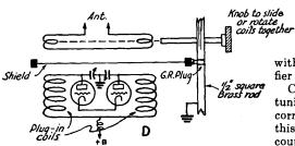
Fig. 1410 — Arrangements for using the shields with single-ended and push-pull circuits.
