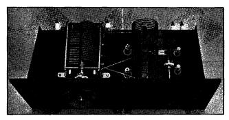
Fig. 1051 — Wide-range antenna coupler. The unit is mounted on a chassis 7 in. by 17 in. by 2 in. with a panel  $8\frac{3}{4}$  in. by 19 in. The condenser is a split-stator unit having a capacity of 210  $\mu\mu$ fds. per section, 0.07-in. plate spacing (Cardwell XT-210-PD). The coils are the B & W TVL series.
