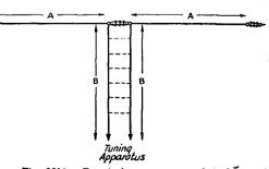
Fig. 2310 — Practical arrangement of a shortened antenna. The total length A + B + B + A, should be a half-wavelength for the lowest-frequency hand, usually 3.5 Mc. See Table II for lengths and tuning data.
