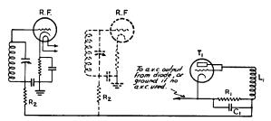
Fig. 1905 — Another protective device for receiver. L<sub>1</sub> is a pickup coil coupled to the transmitter output tank circuit. Size of coil must be determined by experiment.  $C_1 - .002 \mu fd$ .  $R_1 - 100,000$ ohms suggested for first trial. Experiment with particular set-u will be necessary. R2 — Decoupling resistors in receiver AVC system.  $T_1$  — Any tube with grid and plate tied together.
