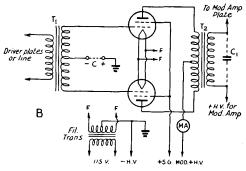
Fig. 1219 — Class-B modulator circuit diagrams. Circuit considerations are discussed in the text.
