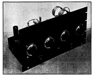
a 6L6 Tri-tet oscillator using a 7-Mc. crystal quadruples to 28 Mc. The 807 intermediate amplifier drives the HK-54 as a straight-through amplifier at 28 Mc. or as a doubler to 56 Mc.
