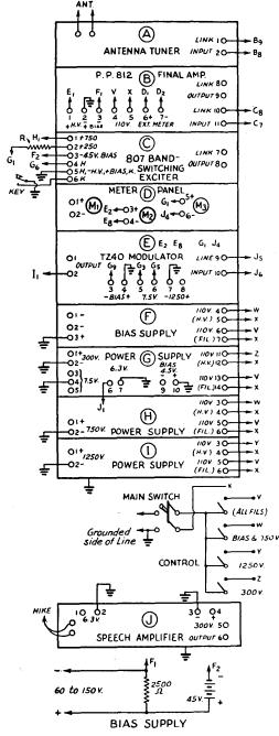
Fig. 1310 - Layout for 300-watt 'phone-c.w. transmitter.
