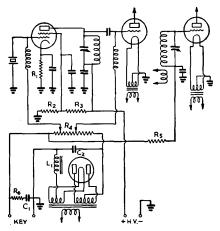
Fig. 1517 - Blocked-grid keying system for break-in. R<sub>1</sub>, R<sub>2</sub>, R<sub>3</sub> — Usual values; R<sub>4</sub> — 20,000 ohms, 50 watts; R<sub>5</sub> — Final stage grid leak.
