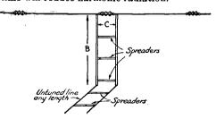
Fig. 2212 — The "Q" antenna with quarter-wave matching section using spaced tubing. Antenna length can be found from Fig. 2204. The matching section length, B, is given by Equation (3). The spacing, C, depends upon the impedance of the untuned line, and can be found from Fig. 2202 for a given size of tubing to make a line having surge impedance determined by Equation 4.
