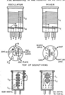
Fig. 810 — How the coils for the three-tuhe superhet are constructed. On the hand-wound coils, all windings are in the same direction.
