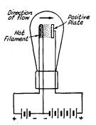
Fig. 305 — Illustrating conduction by thermonic emission of electrons in a vacuum tube. One hattery is used only to heat the filament to a temperature where it will emit electrons. The other hattery places a positive potential on the plate, with respect to the filament, and the electrons are attracted to the plate. The flow of electrons completes the electrical path, and current flows in the plate circuit.
