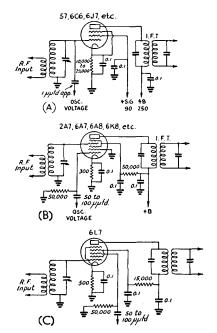
Fig. 416 — Mixer or Converter Circuits. A, grid injection; B and C, separate injection circuits for converter tubes. If an 1851 or 1852 is used in circuit A, the cathode resistor should be changed from 300 to 500 ohms.
