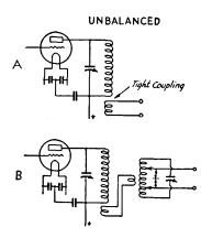
Fig. 2209 — Suitable methods for coupling output circuits to all types of two-wire untuned transmission lines including twisted pair lines, concentric lines and open wire lines. Arrows indicate directions for change of coupling. Link lines always should be coupled to a point of low r.f. potential on the transmitter tank, to avoid transfer of harmonics to the antenna.
