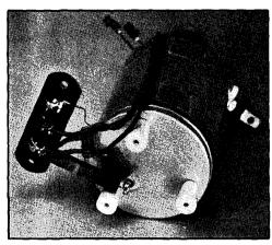
Fig. 2823 - A view under the oscillator shows the grid condenser and leak, the r.f. choke and supporting pillars.
