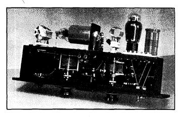
case, it may be of advantage to alter somewhat the values of resistance specified for the voltage dividers in order to increase the voltages on the oscillator plate and screen and also that of the screen of the 807. With a 600-volt supply,  $R_8$  and  $R_9$  should be changed to 1000 ohms each and  $R_4$  to 20,000 ohms and  $R_6$  to 10,000 ohms. Power output will average 30 to 35 watts with the 807 operating as a straight amplifier. (Bib. 2.)
