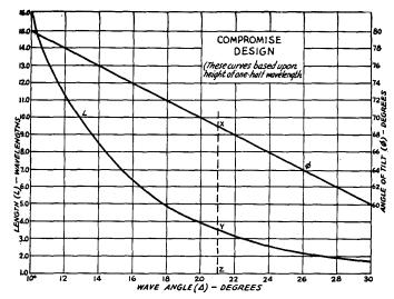
Fig. 2315 — Design chart for rhombic antennas with fixed height (one-half wavelength). The following example illustrates the use of the Chart: Given: Height = ½ wavelength.
