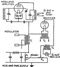
Fig. 1601 — A negative-peak modulation-per cent and overmodulation indicator.
