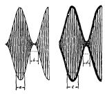
from the output of the modulator rather than from a preceding stage of the audio system. Fig. 1606 is a photograph of the pattern which resulted when the sweep voltage for a trapezoidal pattern was obtained from the output of the audio driver stage instead of the output of the modulator.
