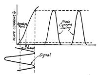
Fig. 327 — Operation of the Class-B amplifier.
