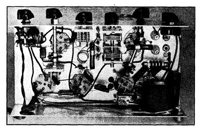
Fig. 2911 - A view underneath the chassis shows the location of parts. The microphone transformer is at the lower right, right next to the microphone connector. The small 3-μμfd. condenser used iu the modulator ean be seen to the left of the transformer, and directly above is the oscillator tuning con-denser. The power cable runs out the back of the set at the lower left-hand corner; the twisted pair taken out the same hole goes to the meter.
