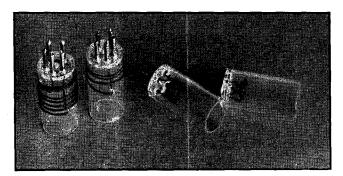
Fig. 2706—The 112-Mc. coils (right) are self-supporting inside the coil forms, while the 56-Mc. coils are wound in the usual manner.
