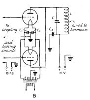
Fig. 519 — Frequency-multiplying circuits. A shows circuit for single or parallel tubes. The arrangement at B is known as the "push-push" doubler circuit. Either capacitive or link coupling may be used.
