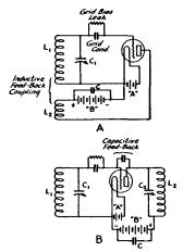
Fig. 330 — Two general types of oscillator circuits.
