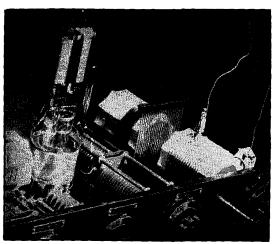
Fig. 1409 — Showing the manner in which the electrostatic shield is mounted between final tank and antenna coupling coils.
