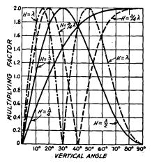
Fig. 2104 — Effect of ground on radiation at vertical angles for four antenna heights. This chart applies only to horizontal antennas, and is based on perfectly conducting ground.
