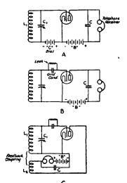
Fig. 331 — Detector circuits of three types. A, plate detection; B, grid detection; C, regenerative grid detection.
