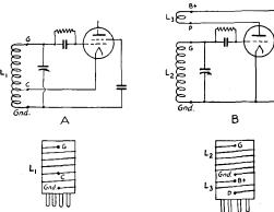
Fig. 903 — The two common types of oscillator circuits used in receivers and the corresponding way in which the coils must be wound to insure proper feedback for oscillation.
