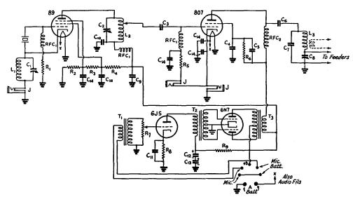
Fig. 2814 - The 89-807 transmitter circuit.
