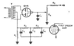
Fig. 616 — Output limiting circuit to prevent overmodulation.
