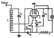
Fig. 1727 — The two-stage field-strength meter circuit diagram.
