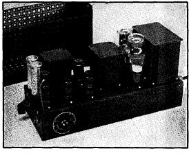
Fig. 1213 — Fifteen-watt speech-amplifier or driver for use with either crystal or double-button carbon microphones.
