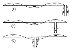
Fig. 2306 — Current distribution and feed points for long-wire antennas. A 3/2-wave antenna is used as an illustration. With two-wire feed, the line may be connected at the end of the antenna or at any current loop (not at a current node). The feeders may he of the resonant type, or a 600-ohm line may be used through a quarter-wave matching section. The "Q" type of matching section also may he used.
