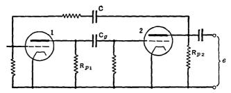
Fig. 14 G. Basic circuit of the multivibrator. Battery voltages omitted for simplicity in explaining its operation
