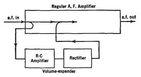
FIG. 32 S. Block diagram of a volume expander
