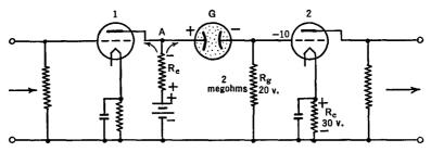
FIG. 24 F. A d.c. amplifier with a glow-tube in the inter-tube coupling unit
