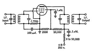
FIG. 33 D. An f.m. limiter circuit
