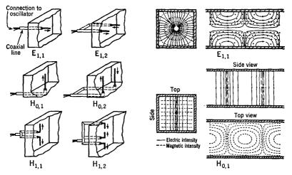
FIG. 38 O. Methods of launching electromagnetic waves into a rectangular waveguide, together with the  $F_{11}$  and  $H_{01}$  field patterns. (See references to Barrow at end of chapter)
