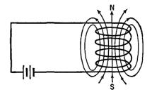
FIG. 3 G. Magnetic field of a solenoid
