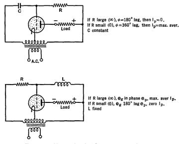
FIG. 19 K. Circuits for the phase control of thyratrons
