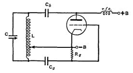
FIG. 14 B. A Hartley oscillator
