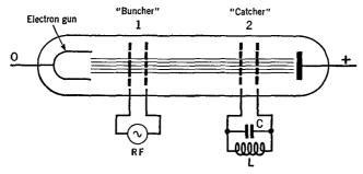
FIG. 38 J. The principle of the klystron
