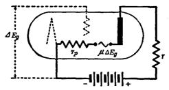
Fig. 12 E. The plate resistance  $r_p$  of a triode. The symbol  $e_g$  is used in the text in place of  $\Delta E_g$  in this figure. (From E. & N. P.)
