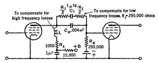
FIG. 25 E. Coupling unit in a wide-band amplifier. See Proceedings of the Institute of Radio Engineers, Vol. 29, page 261, May 1941
