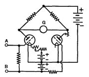
FIG. 24 B. A balanced d.c. amplifier
