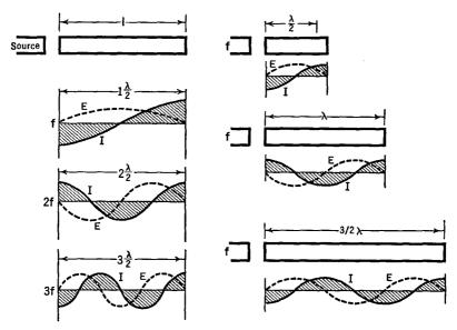
FIG. 36 C. A short-line closed at both ends and resonating to its fundamental and overtones
