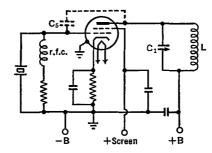
FIG. 29 E. A beam-tetrode crystal oscillator circuit
