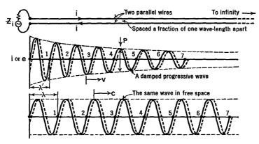
Fig. 35 C. A "long-line" is long in comparison with the wave-length associated with it
