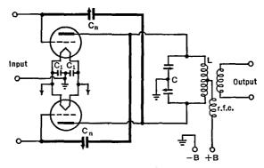
FIG. 27 I. Neutralization of a push-pull amplifier
