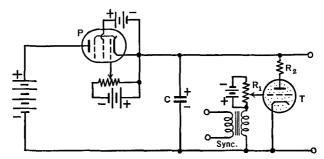
FIG. 22 H. The thyratron T replaces the glow-tube G of Fig. 22 G
