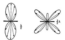
Fig. 8 F. Top view of radiations from horizontal Hertz antennas
