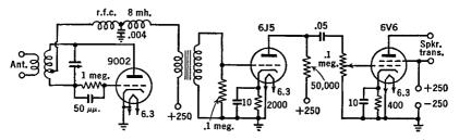
FIG. 37 C. Circuit of an u.h.f. super-regenerative receiver
