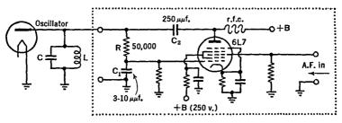
FIG. 33 B. A reactance modulator
