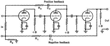
FIG. 26 E. A three-stage feedback amplifier
