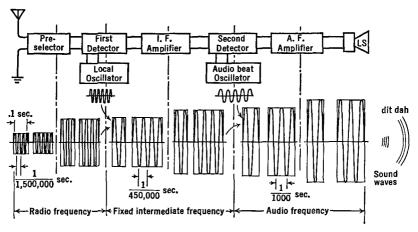
FIG. 32 H. Superheterodyne reception of c.w. signals
