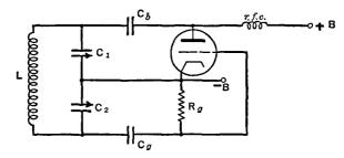
FIG. 14 C. A Colpitts oscillator
