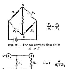
FIG. 2 D. For shunts, the current i is given by the equation above
