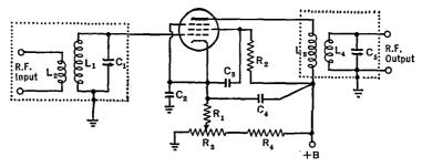
FIG. 27 A. A typical tuned radio-frequency amplifier
