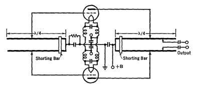
FIG. 37 H. A tuned-grid, tuned-plate, push-pull u.h.f. oscillator
