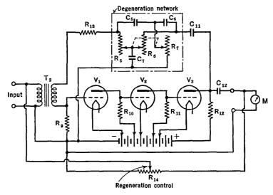
FIG. 26 K. A band-pass amplifier
