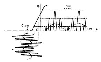
FIG. 16 K. The principle of grid-bias modulation
