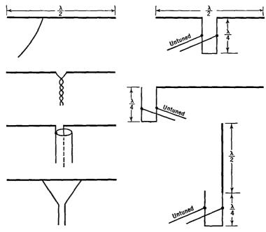
FIG. 36 K. Non-resonant line feeders
