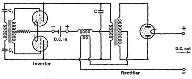
FIG. 19 O. A "d.c. transformer" circuit
