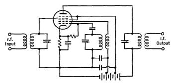
FIG. 32 K. A typical pentagrid converter
