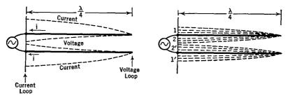
FIG. 36 A. Current and voltage distribution along a quarter-wave folded resonant-line circuit
