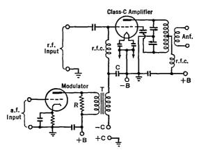
Fig. 28 D. Grid-bias modulation of a r.f. Class C amplifier. The by-pass condenser C should not be greater than approximately  $0.002 \ \mu fd$ .
