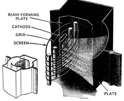
FIG. 15 D. A beam-power tube. (Courtesy R.C.A. Review)
