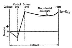
FIG. 15 E. Potential distribution in a beam-power tube
