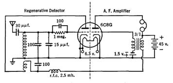
FIG. 32 A. A simple receiver circuit
