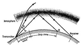
FIG. 9 C. Bending of sky waves
