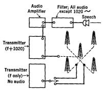
FIG. 34 P. Simultaneous message and beacon transmission
