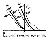
FIG. 18 G. The striking curves of gas-filled triodes. (From E. & N. P.)
