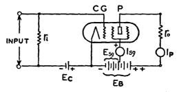
FIG. 15 A. A screen-grid tube. (From E. & N. P.)
