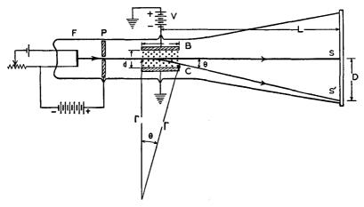
FIG. 1 B. Measurement of the mass and velocity of the electron. (From E. & N. P.)
