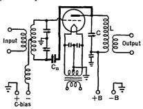
FIG. 27 G. A grid-neutralized r.f. amplifier circuit
