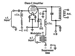
FIG. 28 E. A suppressor-grid modulation circuit. Condenser C should not be greater than  $0.002 \ \mu$ fd.
