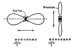
FIG. 36 O. Bi-directional patterns of vertical dipoles with half-wave spacings
