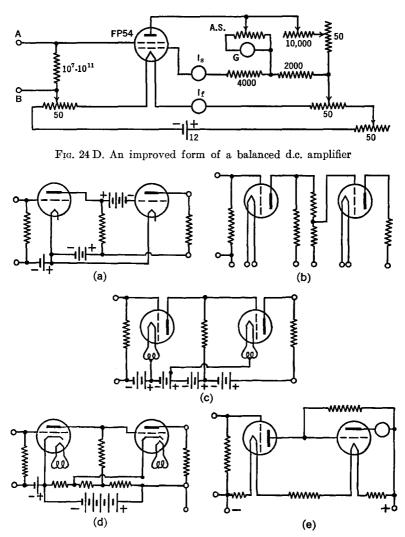
FIG. 24 E. Simple forms of multistage d.c. amplifiers
