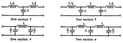
FIG. 7 E. — T- and  $\pi$ -type, low-pass filters
