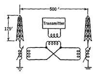
FIG. 34 O. One-half of an A and N transmitting antenna system
