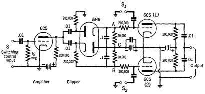
FIG. 30 N. An electronic switch
