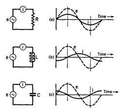
FIG. 4 E. The current i is "in-phase" with the impressed voltage e in a resistance; it lags 90° in an inductance and it leads 90° in a capacitance
