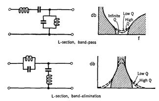
FIG. 7 H. Simple band-pass and band-elimination filters
