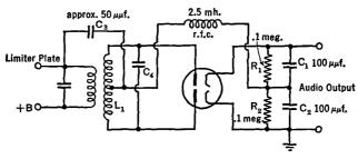
FIG. 33 E. A typical discriminator circuit
