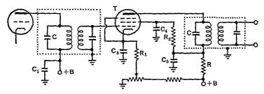
FIG. 27 C. A one-stage i.f. amplifier. T = variable-mu pentode. Typical values;  $C_1$ ,  $C_8$ ,  $C_4$ ,  $C_5 = 0.1 \,\mu$ fd at 455 kc. (= 0.01  $\mu$ fd at 1600 kc. or higher);  $R_1 = 300$  ohms;  $R_2 = 0.1$  megohm; R = 2000 ohms
