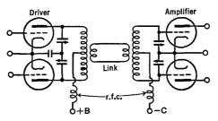
FIG. 31 E. Complete symmetry in coupling
