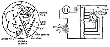
Fig. 20 M. The R.C.A. 931 multiplier phototube
