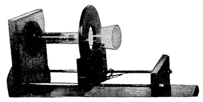
FIG. 21 R. A thin magnetic lens
