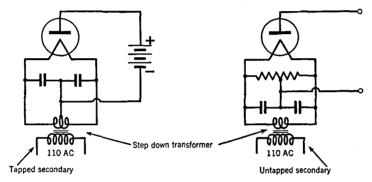
FIG. 10 D. Methods of reducing hum when directly heated filaments are used
