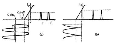
FIG. 30 F. The biasing method of producing sharp pulses
