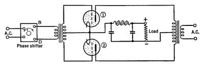
FIG. 19 L. Phase controlled thyratron rectifier circuit
