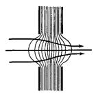
FIG. 21 D. A two-aperture lens
