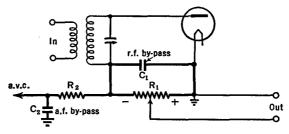
FIG. 32 N. Principle of automatic volume control (a.v.c.)
