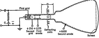
FIG. 21 L. A kinescope (No. 1804)
