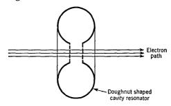
FIG. 38 K. A cavity resonator
