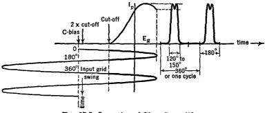
FIG. 27 J. Operation of Class C amplifiers
