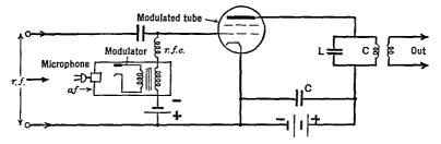
FIG. 16 J. Further details of grid-bias modulation
