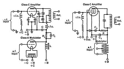
FIG. 28 B. Choke-coupled plate-modulation of a r.f. amplifier
