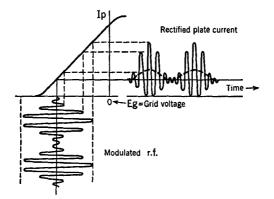
FIG. 17 F. Principle of plate detection
