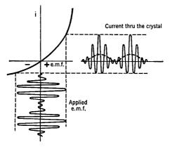
FIG. 17 B. Principle of a crystal detector
