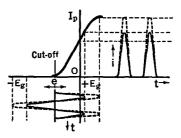
FIG. 23 G. A "characteristic" curve which yields an unusual double-pulse output
