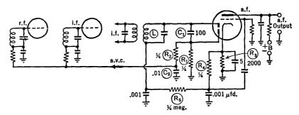
FIG. 32 P. A modern second-detector circuit with delayed a.v.c.
