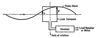
FIG. 34 A. Directional principle of a loop antenna
