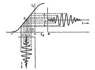
Fig. 13 C. Principle of Class A operation. The output wave-form duplicates the input wave-form
