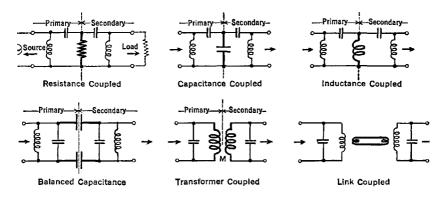
FIG. 7 A. Typical coupling methods
