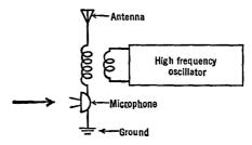
FIG. 16 E. A crude method of amplitude modulation
