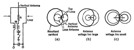
Fig. 34 G. A sensedetermining radiocompass
