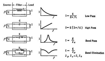
F10. 7 C. Crude filters. Low-pass types use series inductance (top figure). Highpass use series capacitance. Band-pass use series LC circuits. Band-elimination use parallel LC circuits (bottom figure)
