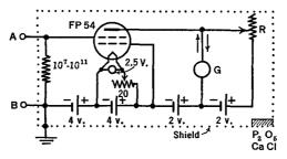
FIG. 24 A. A simple d.c. amplifier
