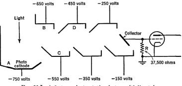
FIG. 20 L. A 6-stage electrostatic photo-multiplier tube
