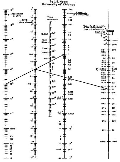
FIG. 3 J. From *Electronics*, Sept. 1937. Instructions for use: Connect resistance and capacitance values to obtain RC product. Connect RC product and time values to obtain quantity of electricity (charge) in condenser at the end of given time value. Example: One microfarad and one megohm gives RC product of unity. At the end of 0.2 second, the condenser is 20 per cent charged or 80 per cent discharged
