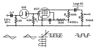
Fig. 30 D. A circuit for changing 60-cycle sine waves into 60-cycle square waves by blocking action. Sharp pulses will be obtained if the time constant RC is made very small
