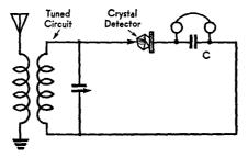
FIG. 17 A. A simple crystal receiver
