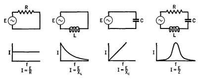
FIG. 5 A. Current from an a.c. generator of variable frequency
