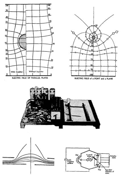
FIG. 3 A. The electrical fields and equipotential lines around several charged bodies together with the apparatus used to measure them. The circuit is taken from the author's book "Electricity Laboratory," distributed by the University of Chicago Bookstore
