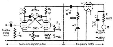
FIG. 30 I. A circuit to convert random pulses into uniform pulses. Also, a frequency meter. (See *Rev. Sci. Inst.*, Dec. 1936)
