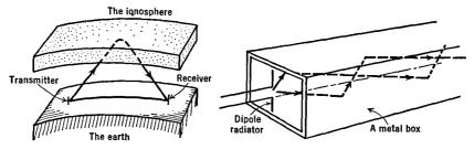
Fig. 38 N. Two shapes of conducting surfaces which will guide electromagnetic waves
