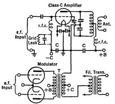
Fig. 28 F. Cathode-modulation. Both of the condensers C should be less than 0.002  $\mu {\rm fd}.$
