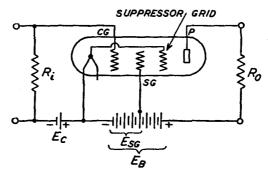
FIG. 15 C. A pentode. (From E. & N. P.)
