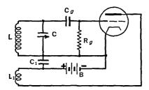
FIG. 14 A. A tickler-circuit oscillator
