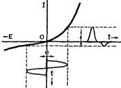
FIG. 23 A. Symmetrical ohmic element
