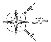
FIG. 34 N. Principle of the A and N beacon
