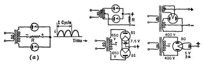
FIG. 11 C. Full-wave center-tap rectifiers
