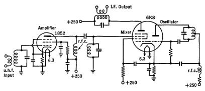
FIG. 37 B. Circuit of an u.h.f. amplifier and converter
