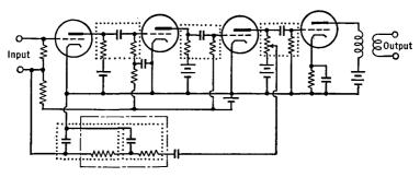
FIG. 26 G. An R-C coupled feedback amplifier
