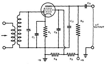
FIG. 17 G. A pentode plate detector
