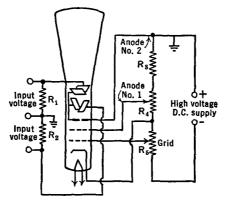
FIG. 21 K. A typical cathode-ray tube circuit. Three-inch 906 tube.  $R_1$  and  $R_2 = 1$  to 10 megohms.  $R_3 = 0.5$  megohms.  $R_4 = 200,000$  ohms.  $R_5 = 20,000$  ohms. High voltage = 1300 volts d.c.
