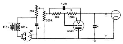
Fig. 30 R. A voltage-stabilized C-bias supply circuit. (k = 1000 ohms)
