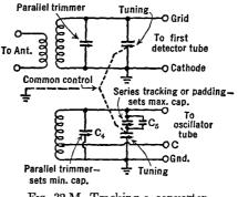
FIG. 32 M. Tracking a converter
