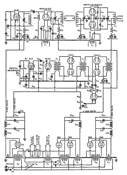
FIG. 31 H. The circuits of a complete transmitter. The r.f. units are at the top, a.f. in the middle and power supplies at the bottom. (Courtesy The "Radio" Handbook, Eighth Edition, Santa Barbara, Calif.)
