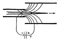
Fig. 21 F. A short-focus double-cylinder lens. (From E. & N. P.)
