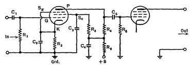
FIG. 25 A. A typical resistance capacitance coupled amplifier
