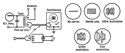
Fig. 31 I. Oscilloscope circuit and wave-envelope patterns for checking the modulation of a transmitter
