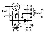
FIG. 27 F. A plate-neutralized r.f. amplifier circuit
