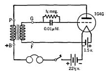
FIG. 14 J. A simple audio frequency oscillator
