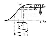
FIG. 23 C. Half-wave non-ohmic element
