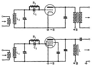
FIG. 17 H. Grid-leak detector circuits
