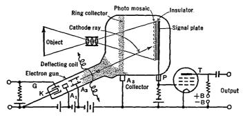
FIG. 21 M. An iconoscope and its circuits
