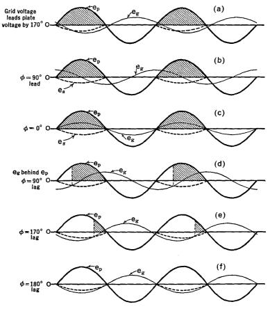
FIG. 19 F. Phase control of the plate current of a thyratron
