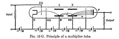
mutual conductance  $(g_m = \text{change of plate current per volt change on the grid})$  of these tubes can be varied greatly by changing the voltage applied to each multiplying stage because this changes the number of secondaries per primary.
