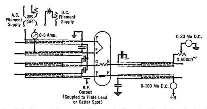
Fig. 37 O. Concentric lines are used to tune the filament, grid, and plate circuits of a 368A "door-knob" tube
