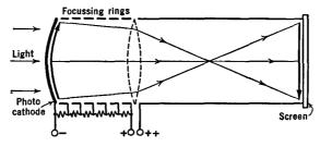
Fig. 21 O. An electron telescope
