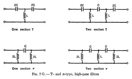
sist of a series condenser, whose reactance is large for low frequencies and small for higher frequencies, and a shunt inductance, which readily bypasses low frequencies but forces the higher frequencies to continue on out to the load R.
