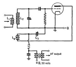
F10. 17 I. A simple regenerative detector.  $(L_3$  has from 10 to 25 per cent the number of turns of  $L_2$ )
