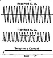
FIG. 32 C. An unmodulated carrier wave will not operate the receiver of FIG. 32 B
