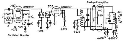
FIG. 37 E. Circuit diagram of an u.h.f. transmitter
