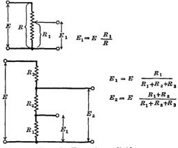
FIG. 2 E. For voltage dividers
