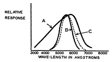
Fig. 20 J. Spectral distribution curves of photronic cells A, compared with the response (B and C) of the human eye to different colors. (From E. & N. P.)
