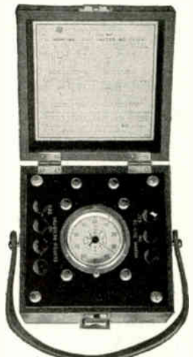
Type MF Synchronous Timer, Calibrated in Cycles, or in Hundredths of Seconds for Setting Relays, 6 1/2 Inches Square
