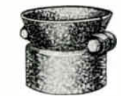
Conduit Bell for Closing Top of Conduit and Supporting Cables
