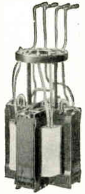
Typical Interior Assembly of Larger Transformer Using Distributed Core Construction
