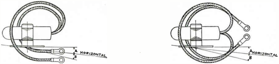
Showing Mounting Arrangement, Minimum Degree of Travel from "Off" to "On" Positions, and Method of Arranging Leads
