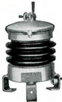
No. 9LA1E17 One-Pole Thyrite Arrester, Max. Rated 3 Kv. for 4160-Volt Grounded or 2400-Volt Ungrounded Neutral Systems (Half Unit Shown)
