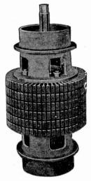
Fig. 396. Movable Core of the Primary Member of an Induction Regulator
