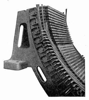
Fig. 135. Armature Coil Support Construction—General Electric Alternator
