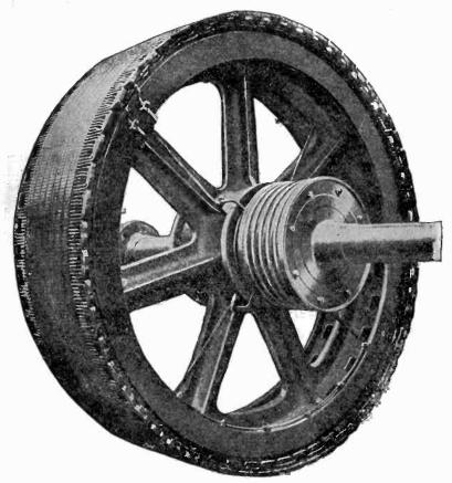
Fig. 112. Completed Armature with Strap Winding, Four Slots Per Phase
