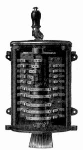
Fig. 337. Westinghouse Controller for Induction Motors
