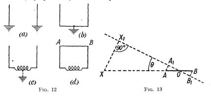
Fig. 12 shows how a pair of spaced aerials can be developed into a "frame" aerial—
