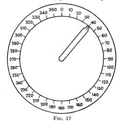
occur in the neighbourhood of  $90^{\circ}$  and  $270^{\circ}$ . In Fig. 17 a bearing of  $40^{\circ}$  is indicated.
