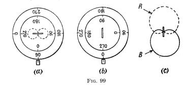
thus rotating the loop through  $90^{\circ}$ . In (c) the two heart-shape diagrams given by the sense switch are shown, and it is clear that, if the transmitter is at  $000^{\circ}$ , "B" will give a minimum. A sensed bearing of  $000^{\circ}$  is, therefore, indicated.
