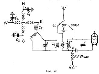
Fig. 76 is the input circuit for a short-wave Adcock installation, and from what has been said previously the diagram will be selfexplanatory. The variable coupling between  $L_1$  and  $L_2$  provides control for a heart-shape balance. The small pre-set condensers  $C_1$ ,  $C_2$ ,  $C_3$ , and  $C_4$  are for the purpose of balancing the aerials on installation in order to compensate for slight aerial inequalities and any unbalance effects due to wiring and switches.
