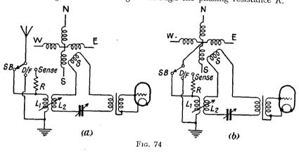
The variable coupling between  $L_1$  and  $L_2$  will assist in obtaining a heart-shape balance.
