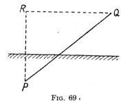
RQ is parallel to the ground and is therefore the normally polarized component.
