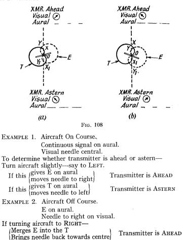
If turning aircraft to RIGHT— Increases volume of E Moves needle further to right
