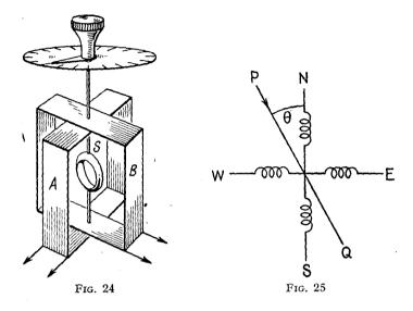
if the transmitter is due east or west, there will be maximum current in the E.-W. loop and none in the N.-S. loop.
