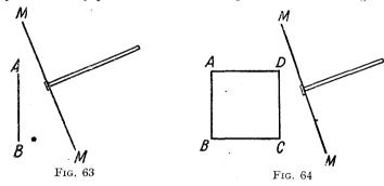
cause a  $90^{\circ}$  error in D/F with a simple frame, because the signal is received on the *horizontal* limbs of the frame instead of the vertical.
