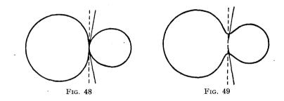
because it is due to the frame aerial acting partly as an ordinary vertical aerial, thus superimposing a circle polar diagram on the figure-8. From what has been previously said, it will be seen that if the "vertical" current is in phase with the resultant frame current, the result will be a "cottage-loaf" polar diagram, the minima being sharp but displaced. This is shown in Fig. 48, the dotted line being the correct minimum position.
