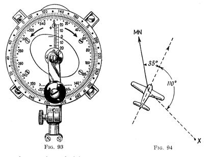
arm has a scale marked from  $+20^{\circ}$  to  $-20^{\circ}$ , and a curve drawn on the stationary dial intersects the scale. The point of intersection gives the correction for quadrantal error at that position. The outer scale is engraved on a movable verge ring, and its purpose will be described shortly.
