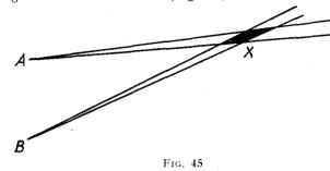
The addition of a third bearing from another D/F station increases the accuracy of the fix by reducing the "area of doubt."
