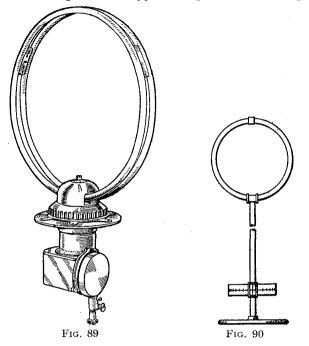
comparatively small air resistance, which is only about 10 lb. at an air speed of 300 m.p.h. with the loop set at  $090^{\circ}$  to the line of flight.
