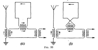
E.M.F.'s due to the open aerial and the loop will thus be aiding one another for one position of the loop and in opposition for the other. The combination will, therefore, give one maximum and one minimum position instead of two equal maxima as in the case of the
