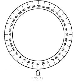
Since the relative movement is reversed, the scale engraving must be anti-clockwise, as in Fig. 18, in which a bearing of 40° is indicated.
