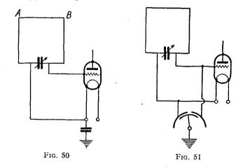
of capacity between the two sides of the frame and earth and hence to effect a balance.
