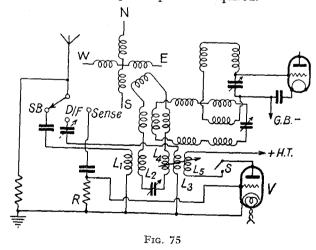
Fig. 75 is a rather more complex input circuit for a medium wave Adcock installation. The complexity is, however, more apparent than real and arises from the special precautions taken to secure
