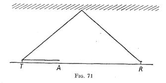
space in which the signal cannot be heard, points in this space being too far away to receive the direct ray and not far enough to receive the first reflection.
