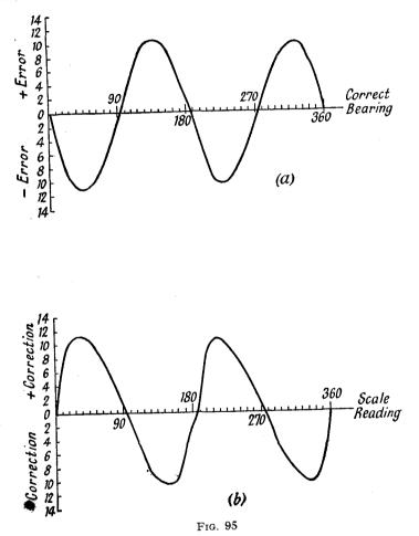
mounted on the fuselage or hull well clear of the wings. If the loop is mounted on or very close to the wings, the bearings may be pulled towards the athwartships line, thus causing a positive error in the first quadrant.
