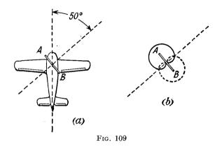
determined angle if a correction for drift due to cross-wind is applied). This is the position at which the indications shown in Fig. 108 and described in the context hold good. It is clear, however, that if the loop is set to a scale reading of  $180^{\circ}$ , the heart-shape diagrams will be laterally reversed, and the indications normal for a transmitter ahead will then be given by a transmitter which is astern, all the indications shown in Fig. 108 being reversed.
