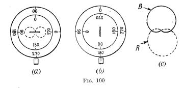
180°. In (c) the two heart-shape curves are shown. Since the transmitter is actually at  $000^{\circ}$  it is clear that "R" will give a minimum, thus indicating that the true bearing is the reciprocal of 180°, i.e.  $000^{\circ}$ .
