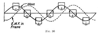
this is the case the reasoning breaks down and heart-shape reception does not exist. Unfortunately, a  $90^{\circ}$  phase difference occurs to start with, because the E.M.F. induced in an open aerial is in phase with the wave influencing it, whereas the resultant E.M.F. in a
