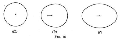
This is by no means difficult, and it should be remembered that a polar diagram is qualitative rather than quantitative, i.e. it is a handy pictorial way of showing the behaviour of an aerial rather than a mathematical figure. So much is this the case that switches on D/F apparatus are often engraved with small representations of polar diagrams instead of words. The aerial systems and polar diagrams which lead directly to D/F will now be discussed.
