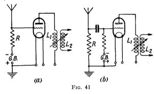
aerial. The resistance R is about 100,000 ohms and the value is biased to zero grid current and works on a straight portion of its mutual characteristic. The variable coupling between  $L_1$  and  $L_2$ serves to control the amplitude of the signal from the vertical aerial and is useful to secure a heart-shape balance.
