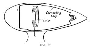
a fore-and-aft correcting loop is quite useless if the error is positive in the first quadrant.
