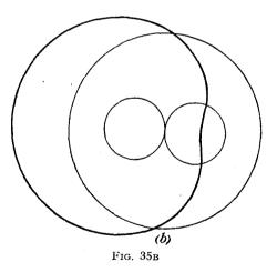
only requirement is *sufficient difference* between the heart-shape minimum and maximum. The "perfect" heart-shape of Fig. 34 is not always easy to obtain and in practice is not invariably aimed at. ' So long as a reasonable approximation to heart-shape reception is available, bearings can be satisfactorily sensed.
