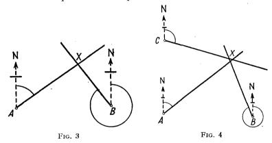
cross-bearings, and will be the point at which the bearings from two or more D/F stations intersect.
