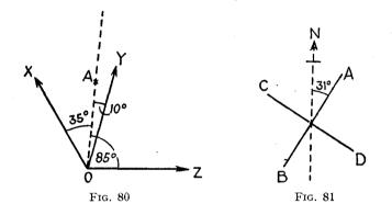
For illustration, bearings of  $35^{\circ}$ ,  $10^{\circ}$ , and  $85^{\circ}$  have been taken. A represents a ranging pole which is moved under the direction of the person using the theodolite or sextant until the three angles are correct. This fixes the N.-S. line and the E.-W. line can then be laid down by a combination of theodolite or sextant observations and geometrical checks as previously described.
