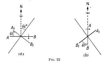
the stop-watch. If  $A_1B_1$  is the position of the frame at the minimum signal the bearing of the receiving station must clearly be on the line at right angles to  $A_1B_1$ . If t seconds are shown on the stop-watch, the bearing will be either  $6t^{\circ}$  or  $(6t + 180)^{\circ}$ .
