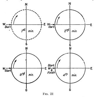
misunderstood, is that the position of the frame at the *north* starting signal is *east-west*. An aircraft or ship which is nearly due north or south of the beacon will, therefore, not hear this signal because the frame will, at that moment, be at  $90^{\circ}$  to his bearing. This is the reason for providing the *east* starting signal which occurs when the frame is *north-south*.
