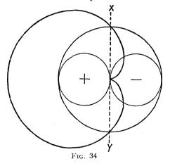
frame alone. The reversal of E.M.F. in the frame occurs as it passes through the minimum position, so that the frame E.M.F. must be considered positive for one circle of the figure 8 and negative for the other, the open aerial E.M.F., of course, remaining positive, as this is unaffected by direction.
