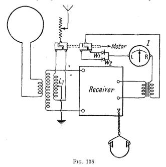
rotary switch running synchronously with the first. Both switches are on the same shaft, and are driven by a small electric motor supplied from the aircraft's main battery.
