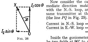
Now consider the case for an inter- $\cos\theta$  mediate direction making an angle  $\theta$ with the N.-S. loop, and assuming the same transmitter at the same distance
