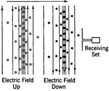
Fig. 9-17. Reception of an Electromagnetic Wave by a Receiving Antenna.
