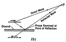
Fig. 16-21. Image Antenna Due to a (Perfectly) Reflecting Ground. (a) Vertical antennas (reflection without phase reversal). (b) Horizontal antennas (phase reversal on reflection).
