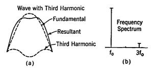
Fig. 14-3. Distorted Wave and Components.
