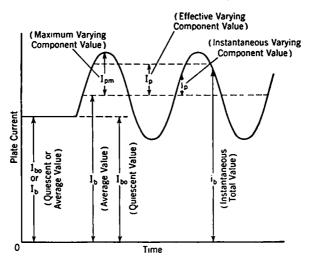
Fig. 4-10. Components of Plate Current.
