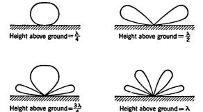
Fig. 16-23. Vertical Radiation Patterns of a Horizontal Antenna at Various Heights above a (Perfect) Ground.
