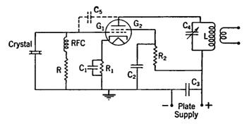
Fig. 12-4. Crystal-controlled Circuit-Tetrode Tube.
