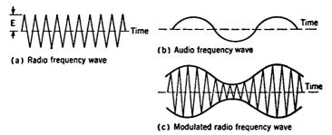
Fig. 10-6. Modulation of a Radio-frequency Wave.
