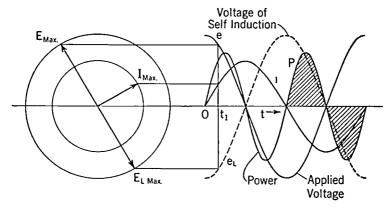
Fig. 3-13. Current, Voltage, and Power in an Inductive Circuit.
