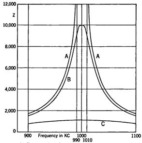
(b) Frequency, impedance characteristic of parallel circuit Fig. 11-2. Impedance of Parallel Circuit.
