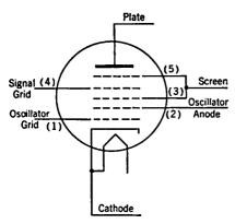
Fig. 4-20. Pentagrid Converter.
