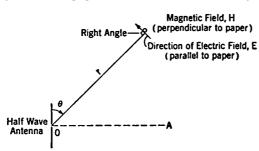
Fig. 9-16. Direction of the Electric Field about an Antenna.
