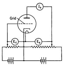
Fig. 4-7. Circuit for Obtaining Triode Characteristics.
