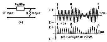
Fig. 11-24. Rectification of Radio-frequency Signal.
