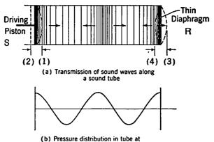
Fig. 9-8. Transmission of Sound Waves along a Tube, Showing the Instantaneous Pressure Distribution.
