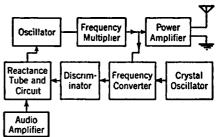
Fig. 14-6. Reactance-tube or Crosby System Frequency-modulation Transmitter.
