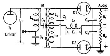
Fig. 14-10. Frequency-modulation Detector or Discriminator.
