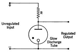
Fig. 5-10. Regulated Voltage Supply.
