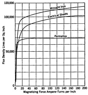
Fig. 2-27. Typical Magnetisation Curves.
