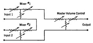
Fig. 7-26. Complete Mixing System.
