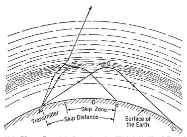
Fig. 15-5. Effects on Transmission Due to the Angle at Which the Sky Wave Is Transmitted.
