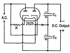
Fig. 5-5. Voltage-doubler Circuit.
