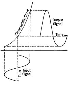
Fig. 6-2. Nonlinear Distortion.
