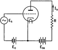
Fig. 4-11. Triode with Resistance Load.
