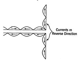
Fig. 9-14. Antenna Longer than One Wave Length, Showing Canceling Current Loops,
