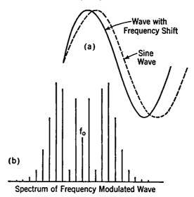
Fig. 14-4. Distorted Wave and Frequency-modulation Spectrum.
