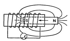
Fig. 3-7. The Bar Magnet Being Inserted in the Coil.
