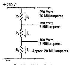
Fig. 2-34. A Voltage Divider.
