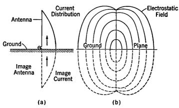
Fig. 16-4. A Quarter-wave Vertical Antenna at the Surface of the Earth. (a) Antenna and its image, showing current distribution. (b) Electrostatic field about the antenna, showing how the image antenna can be used to account for the effect of the ground.
