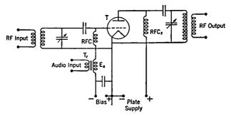
Fig. 12-7. Grid-modulation Circuit.
