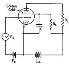
Fig. 4-15. Screen Supply for Tetrode.
