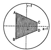
Fig. 8-9. Trapezoid Pattern Showing Modulation.
