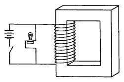
Fig. 3-12. Energy Is Stored in the Magnetic Field of a Transformer.
