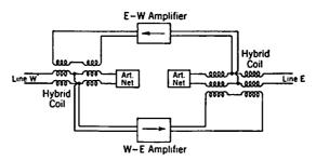
Fig. 6-8. Type 22 Telephone Repeater.
