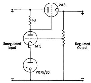
Fig. 5-11. Electronic Voltage Regulator.
