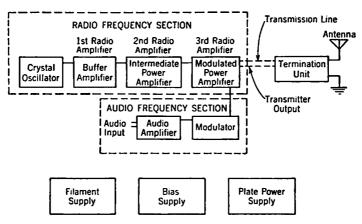
Fig. 12-1. Block Diagram of Crystal-controlled Amplitude-modulated Transmitter (high-level modulation).
