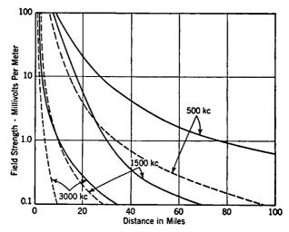
Fig. 15-2. Effect of Frequency and Ground Conductivity upon the Strength of the Ground-wave Signal. Solid lines: fairly good conductivity ( $100 \times 10^{-15}$  e.m.u.). Dashed lines: poor conductivity ( $20 \times 10^{-15}$  e.m.u.).
