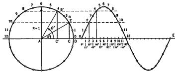
Fig. 1-8. Construction for Sine Curve.
