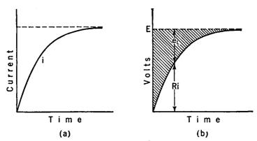
Fig. 3-11. (a) Current Rise in an Inductive Circuit. (b) Voltage Distribution in an Inductive Circuit.
