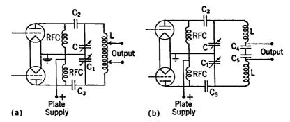
Fig. 11-17. Types of Push-pull Radio-amplifier Output Circuits.
