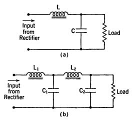
Fig. 5-6. Choke-input Filter Circuits: (a) Singlesection, (b) Two-section.
