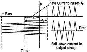
Fig. 11-23. Grid-voltage-Plate-current Relation in Class C of Radio Amplification.
