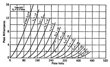
Fig. 4-9. Plate Characteristics of 6J5 Triode.
