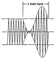
Fig. 14-1. Frequency-modulated Wave.
