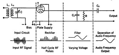
Fig. 11-30. Linear Plate Detector.
