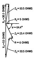
Fig. 3-25. Vector Diagram — Resistance, Inductance, and Capacitance in Series.
