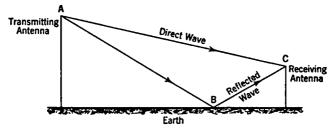
Fro. 15-11. Reception of Direct and Reflected Waves at Ultrahigh Frequencies.
