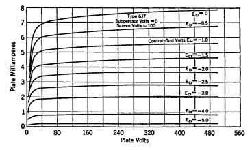
Fig. 4-16. Plate Characteristics of 6J7 Pentode.
