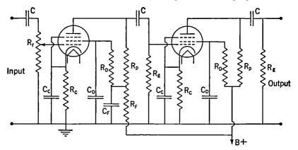
Fig. 7-5. A Two-stage Resistance-coupled Amplifier Using Pentodes.
