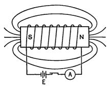
Fig. 3-10. The Magnetic Field of a Coil Carrying Current.
