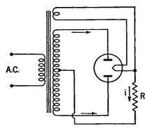
Besides giving a better wave form than the half-wave rectifier, the fullwave circuit has the advantage of symmetrical action in the transformer. In the half-wave circuit, the secondary currental ways flows in the
