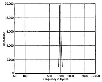
Frg. 11-3. Parallel Resonant Circuit at Audio Frequencies. Electrical Constants Equivalent to (B) of Fig. 11-2.
