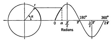
Fig. 3-1. A Rotating Radius Vector May Be Used to Produce a Sine Wave.
