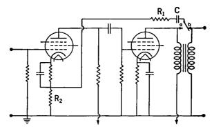
Fig. 7-15. Two-stage Amplifier with Inverse Feedback.
