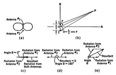
Fro. 16-17. Horizontal Radiation Pattern for Two Vertical Antennas Spaced One Half Wave Length and Fed In-phase. (a) Radiation pattern. (b), (c), (d), and (e) Method of obtaining pattern.
