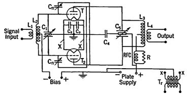
Fig. 11-16. Push-pull Triode Radio-frequency Amplifier.
