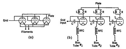
Fig. 11-15. Parallel Operation of Vacuum Tubes.
