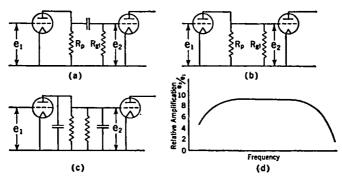
Fig. 7-3. Equivalent Circuit for a Resistance-coupled Amplifier at: (a) low, (b) medium and (c) high frequencies; and (d) the type of response obtained.
