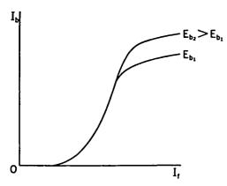
Fig. 4-3. Limitation of Diode Current by Space Charge.
