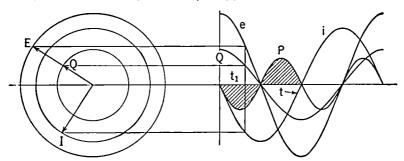
Fig. 3-23. Current, Voltage, and Power in a Capacitive Circuit.
