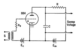
Fig. 8-4. Cathode-ray Sweep Generator.
