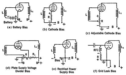
Fig. 11-7. Grid-bias Voltage Supplies.
