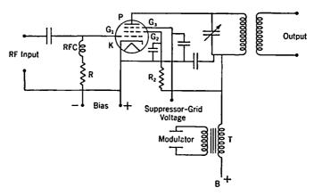
Fig. 12-9. Modulation of Screen-grid Tube.
