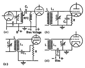
Fig. 11-5. Types of Radio-amplifier Input Circuits.
