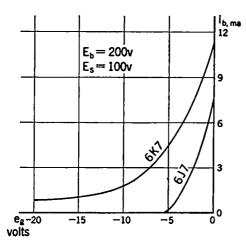
Fig. 4-17. Mutual Characteristics of 6J7 and 6K7, Showing Sharp Cutoff and Remote Cutoff.
