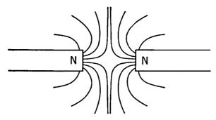
Fig. 2-22. The Magnetic Field about Two Like Poles.
