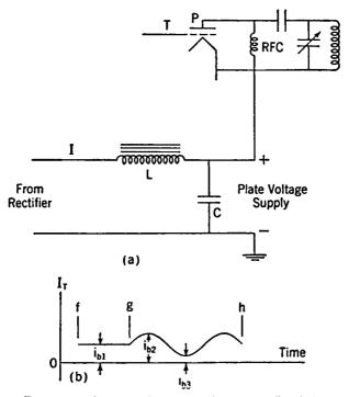
Fig. 12-11. Class B Radio Amplifier Plate-supply Regulation.
