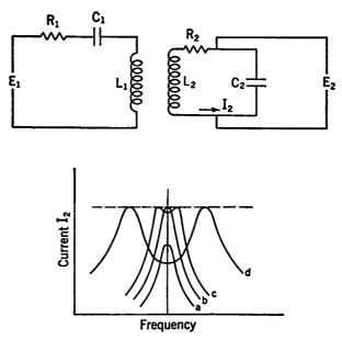
Fro. 3-32. Resonance Curves for Tuned Circuits with Different Amounts of Mutual Coupling.
