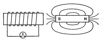
Fig. 3-6. A Coil and a Bar Magnet.
