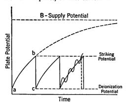
Fig. 8-6. Plate Potential of the Sweep Generator Tube.
