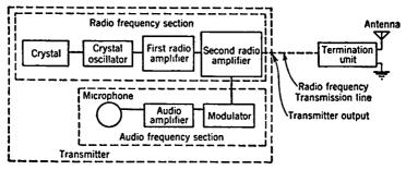
Fig. 10-2. Radiotelephone Transmitting Station.
