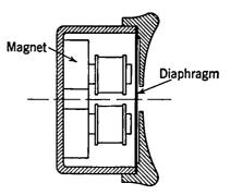
Fig. 6-4. Telephone Receiver.
