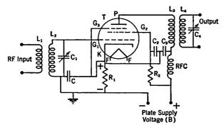
Fig. 11-12. Diagram of Pentode Radio-frequency Amplifier
