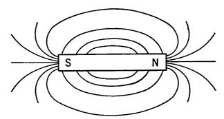
Fig. 2-20. The Magnetic Field of a Bar Magnet.
