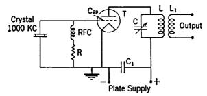
Fig. 12-3. Simple Crystal-control Circuit-Triode Tube.
