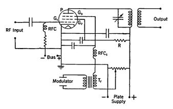
Fig. 12-10. Suppressor-grid Modulation.
