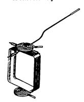
Fig. 2-32. The Moving-coil Assembly.
