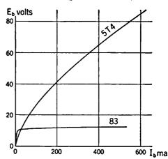
Fig. 5-9. Plate Characteristics of Rectifier Tubes.
