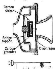
Fig. 6-3. Carbon Microphone.
