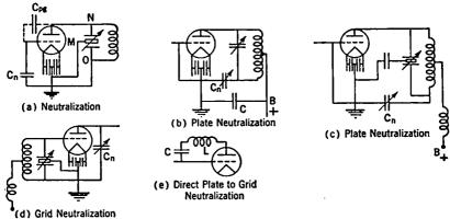
Fig. 11-11. Types of Neutralization for Radio Amplifiers.
