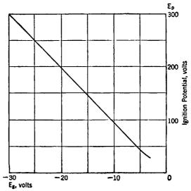
Fig. 8-5. Control Characteristic of Type 884 Gas Triode.
