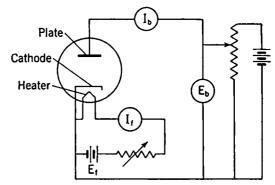
Fig. 4-1. Circuit for Obtaining Diode Characteristics.
