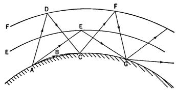
Fig. 15-9. Fading Due to Interference between Waves Which Have Traveled Different
