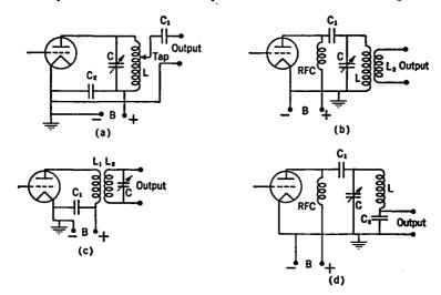
Fig. 11-6. Types of Single-ended Radio-amplifier Output Circuits.
