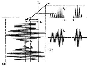
Fig. 11-19. Grid-voltage-Plate-current Relation in Class B Radio Frequency Amplification. Improper Operation. Bias Too Figh.
