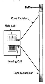
Fig. 6-5. Cone Type of Loudspeaker.
