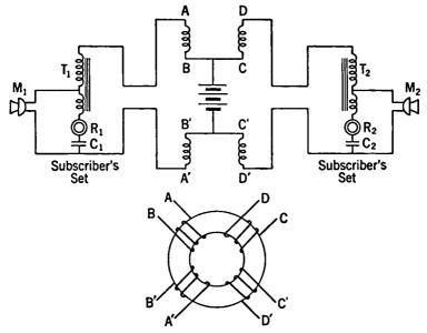
Fig. 6-7. Common-battery Telephone Circuit.
