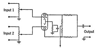
Fig. 7-24. Improved Electronic Mixing Circuit.
