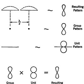
Fig. 13-20. Pattern of a Colinear Array (Half Waves In-phase)—Obtained by Multiplication of Group and Unit Patterns.
