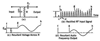
Fig. 11-25. Filtering of Radio-frequency Wave to Obtain Audio Frequency.
