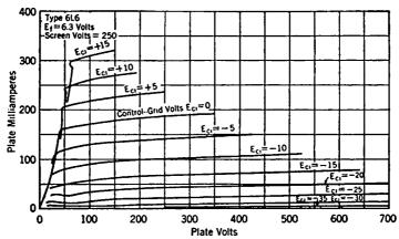
Fig. 4-19. Plate Characteristics of 6L6 Beam Power Tube.
