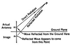
Fig. 16-5. Vertical Antenna at the Earth's Surface Showing How the Image Can Be Used to Account for the Reflected Wave.
