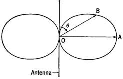
Fig. 16-3. Radiation Characteristic of a Half-wave Antenna.
