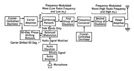
Fig. 14-5. Block Diagram of Armstrong Frequency-modulation Transmitter System.
