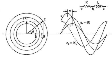
Fig. 3-16. Alternating Current and Voltage with Resistance and Inductance in Series.
