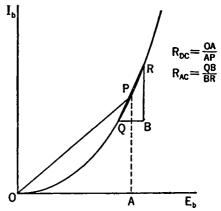
Fig. 4-4. D.C. and A.C. Plate Resistance.
