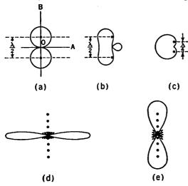
Fig. 16-18. Radiation Patterns for Commonly Used Antenna Arrays. (a) Two antennas spaced one half wave length and with 180° phase difference. (b) Same with 90° phase difference. (c) Two antennas spaced one quarter wave length and fed with 90° phase difference. (d) Broadside array (currents in-phase). (e) End-fire array (currents 180° out-of-phase).
