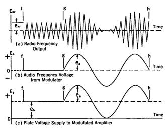
Frg. 12-6. Plate Modulation: Variation of Power Output with Variation in Plate Voltage.
