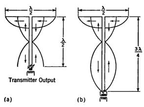
Fig. 16-7. Resonant Line Feed to Half-wave Antenna. (a) Line has low input impedance when it is an integral number of half wave lengths Long. (b) Line has high input impedance when it is an odd number of quarter wave lengths long.
