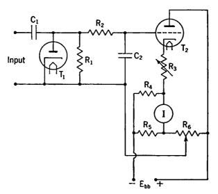
Fig. 8-10. Diode Vacuum-tube Voltmeter with D.C. Amplifier.
