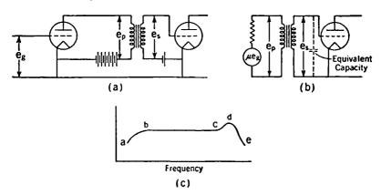
Fig. 7-9. (a) Transformer-coupled Amplifier. (b) Approximate Equivalent Circuit Showing Effect of Capacities. (c) Typical Frequency-response Curve.
