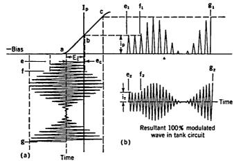
Fig. 11-18. Grid-voltage-Plate-current Relation in Class B Amplification of a Modulated Radio-frequency Wave. Proper Operation.
