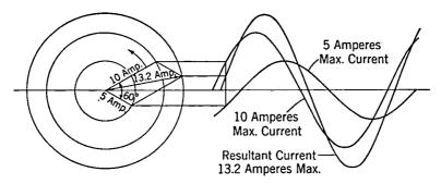
Fig. 3-3. Addition of Alternating Currents.
