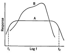
Fig. 6-1. Frequency Distortion.
