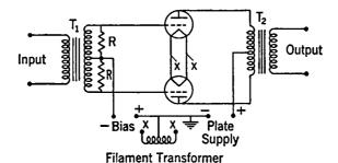
Fig. 11-22. Circuit Diagram of a Push-pull Class B Audio Amplifier.
