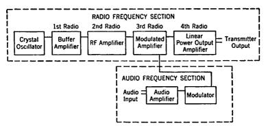
Fig. 12-2. Block Diagram of Crystal-controlled Amplitude-modulated Transmitter (low-level modulation).
