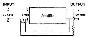
Fig. 7-14. Principle of Inverse Feedback.
