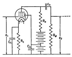
Fig. 7-4. Circuit of a Resistance-coupled Pentode Amplifier.
