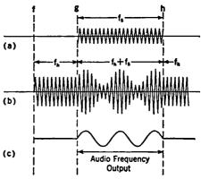
Fig. 11-34. Detection of Keyed Transmitted Continuous Wave.
