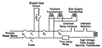
Fig. 12-16. Transmitter Control Circuit.
