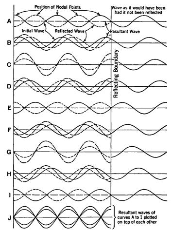
Frg. 9-5. Reflection of a Wave at a Boundary, Showing Addition of Initial and Reflected Waves to Give Standing Waves.
