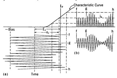
Fig. 12-8. Grid-voltage-Plate-current Relation in Grid Modulation.
