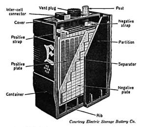
Fig. 2-19. An Assembled Lead Storage Cell (cut away to show the construction).
