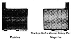
Fig. 2-16. Storage-battery Plates.
