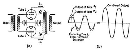
Fig. 7-12. (a) A Push-pull Amplifier. (b) Reduction of Even Harmonic Distortion by Use of Push-pull Connection.
