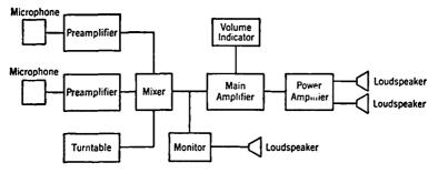
Fig. 7-21. Block Diagram of a Large Public-address System.
