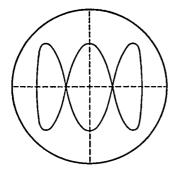
Fig. 8-8. Lissajous Figure, Frequency Ratio 3:1.
