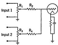
Fig. 7-22. Resistance Mixing Circuit.
