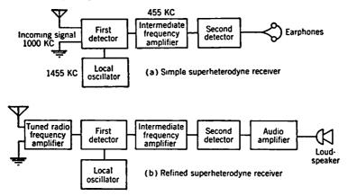
Fig. 10-4. Superheterodyne Receivers.
