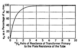
Fig. 7-10. Voltage  $c_p$  across the Primary Winding of a Transformer as a Function of the Reactance of the Winding
