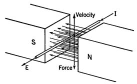
Fig. 2-23. Relation Between (a) Magnetic Field, Motion, and Voltage; (b) Magnetic Field, Current, and Force.
